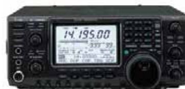
IC-7400, HF/6 M, VHF, 100 Watt 13,8 VDC
