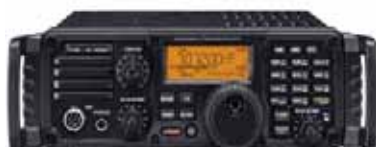
IC-7200, HF/6 M, 100 Watt 13,8 VDC
