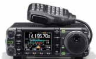
IC-7000, HF/6 M, VHF, UHF 100 W, 13,8 VDC
