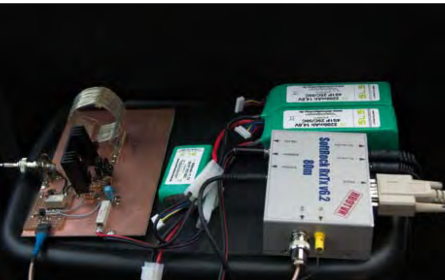
Le transceiver SDR de Peter Kohler, HB9TVK. SDR-Transceiver von Peter Kohler, HB9TVK.
