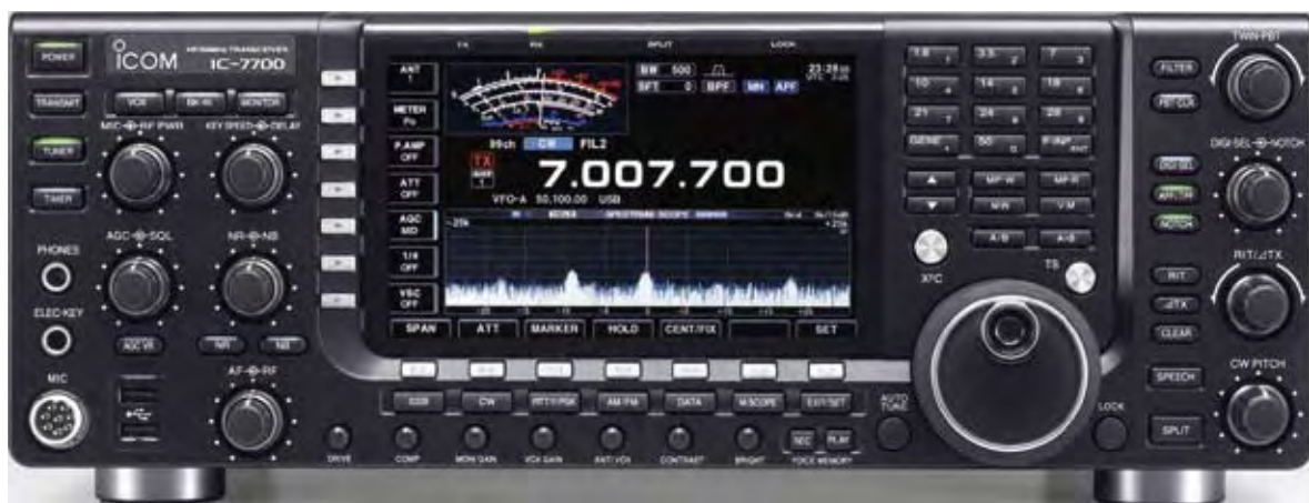
HF/6 Meter (RX 0.030 – 60.000 MHz), TX 200 Watt Betriebsarten USB, LSB, CW, FM, PSK31, RTTY (FSK)
