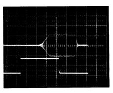
Fig. 3 — Cw keying waveform of the IC-740. Upper trace is the actual key closure; lower trace is the rf envelope. Each horizontal division is 5 ms. This keyed wave has a rapid fall time, which *may* cause key clicks.
