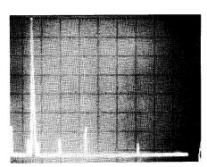
Fig. 1 — Spectral display of the IC-740. This is the worst-case condition, operating with 105-W output on 14 MHz. Each vertical division is 10 dB, and each horizontal division is 10 MHz. The IC-740 complies with current FCC specifications for spectral purity.
