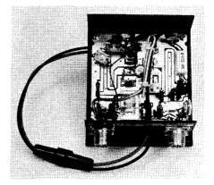
Fig. 8 — Neat, compact layout of the B-23 amplifier. This package can easily be tucked out of sight - even in today's compact cars.
