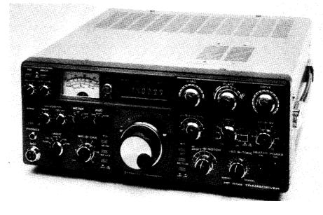
Age is manually switched. Three switch positions are provided: FAST, SLOW or OLF. This is a welcome feature, especially for ew operators. Age action is smooth with no evidence of popping.
