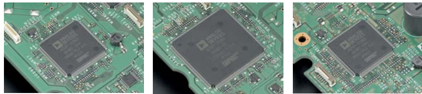
For main receiver IF DSP ADSP-21363 clock @333 MHz
