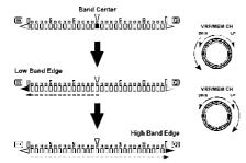
Alternately, you can have the segments expand outwardly as you tune either direction from the nearest displayed frequency. This lets you view tuning increments smaller than 10 Hz (the maximum display resolution).
