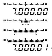
The rate and distance of segment displacement in either mode are proportional to the selected tuning step size and depend on whether or not the [FAST] button is engaged. The tuning meter mode is selected by menu selection 3-2.
