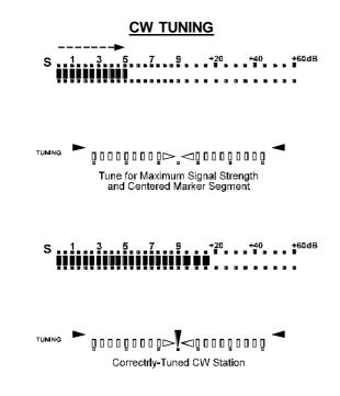
For RTTY and Packet, dual segments appear (representing the mark and space tones), and in this case optimum tuning is achieved when even balance and maximum separation between the dual segments occur. The minimum separation between the segments is proportional to the mark and space tone shift (170 Hz, 425 Hz or 850 Hz). We will cover more about RTTY and Packet operation later.
