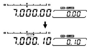
When the VRF feature is engaged, the segments briefly indicate the peak position for the narrow bandpass "preselector" when you are turning the VRF/MEM CH knob. Be sure to see page 44 for more details on VRF operation.
