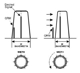
Using WIDTH control to reduce QRM
