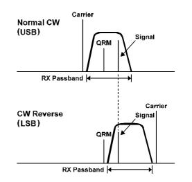
**Operating Hint** - An added benefit from this feature is QRM rejection. If you have interference on a CW station that the IF SHIFT does not easily eliminate, you can try switching to the reverse sideband, retuning the signal, and trying the IF SHIFT again.
