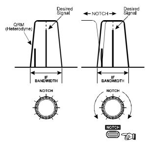
The NOTCH feature actually has three operating modes, involving different combinations of the IF Notch filter and/or the EDSP Notch filter. You may use *menu selection 2-9* to utilize only the IF Notch (*IF NOTCH* selection), the EDSP Notch (*Auto DSP* selection), or both Notch filters (*SELECT*). With *Select* engaged, any residual interference getting past the IF Notch will be eliminated by the EDSP Auto-Notch, and this combination of filters provides impressive results!
