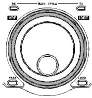
frequency steps incrementing through the arc of the **Shuttle Jog** (from 10 Hz ~ 100 kHz). The **Shuttle Jog** speed (encoder rate) is also configurable from 1 ~ 100 msec. via *menu selection 1-1* on page 99.
