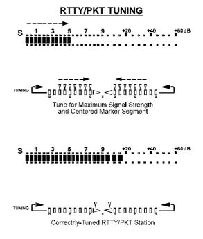
"Peak-Hold" Feature - During receive, the S-Meter segments respond instantaneously to the relative signal strength (in S-Units) of stations. The meter "peakhold" circuitry keeps the right-most bargraph segment on for a user-selectable time delay from 10 msec up to 2 seconds. The peak-hold feature is off by default, but you can enable it and select the desired delay time via *menu function 3-7*.
