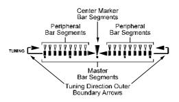
In the CW mode, when you tune a signal near the center of the receiver passband, the boundary arrows light, and the upper signal strength segments increase as you slowly tune the VFO knob. The idea is to tune for maximum indication, and so that a lone center marker illuminates in the lower tuning meter (the boundary arrows turn off when the marker is centered). If you detune, the arrows illuminate, indicating that you need to re-center the marker.
