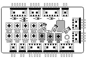
Meter Calibration Points (Top Panel Access)
