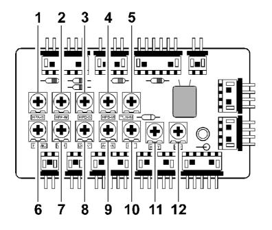
The following controls are accessible beneath the removable panel on the top half of the transceiver case. Push the slide rearward and pry up the lid to expose the ALC UNIT circuit board and potentiometer controls. Most control settings are preset at the factory for normal operation. Should you desire to change a particular setting, use a small insulated screwdriver to rotate the desired potentiometer.
