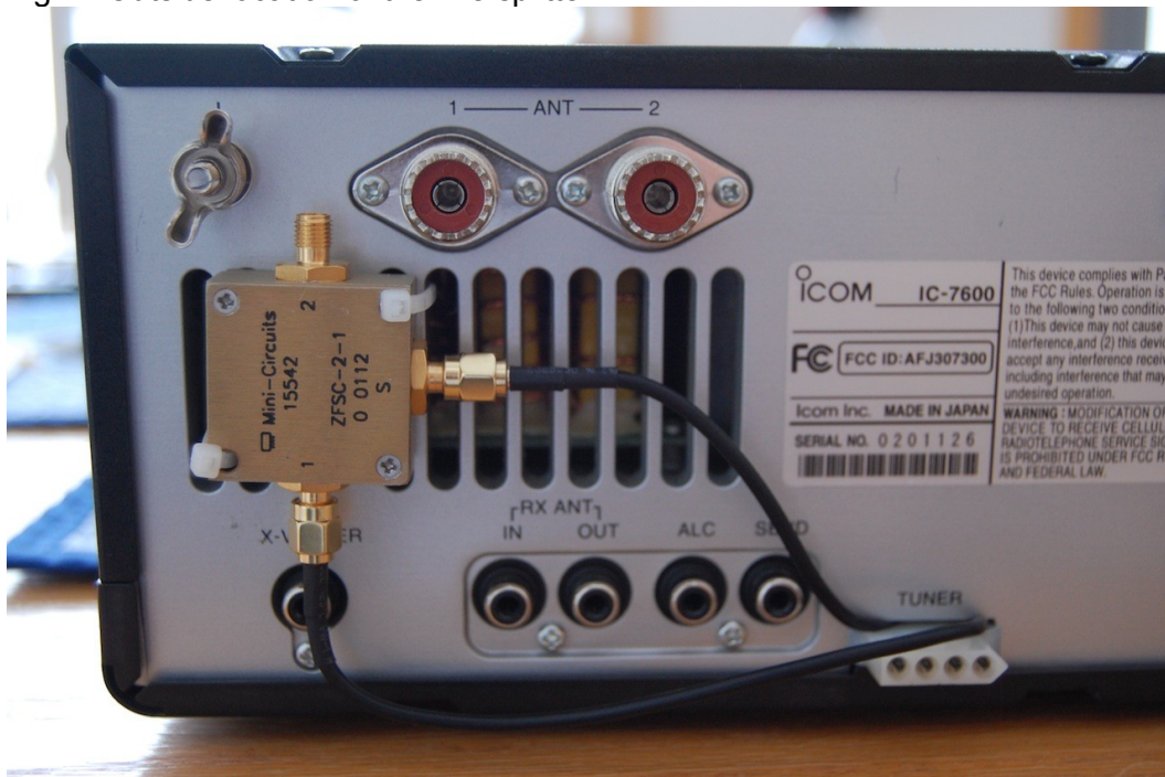
Fig. 4: Outside location of the line splitter.
