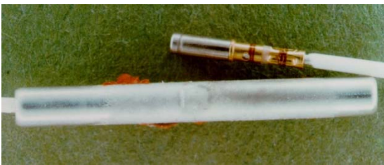
Figure 19-33. Crimped Contact Outside Junction Device
