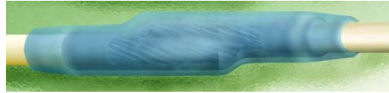
Figure 19-5. Double Sleeving over Soldered Connection
