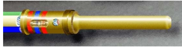
Figure 19-23. Wires Crimped Within Contact
