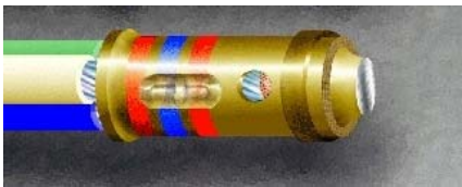
Figure 19-24. Contact Trimmed and Deburred
