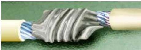
Figure 19-11. Soldered Lash Splice
