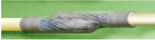
Figure 19-4. Sleeving over Soldered Connection
