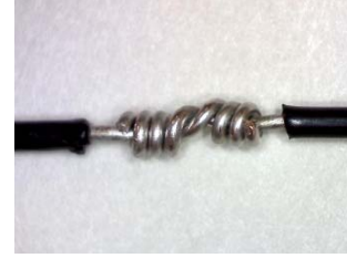
Figure 19-17. Completed Wrap for Western Union/Lineman Splice
