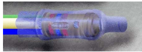
Figure 19-25. Contact Covered With Shrink Sleeving
