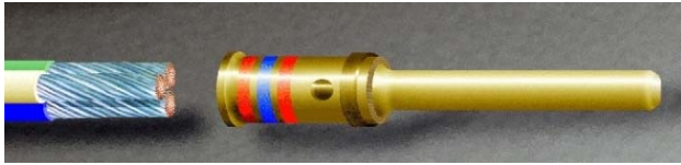
Figure 19-22. Stripped Wire Bundle Prior to Insertion
