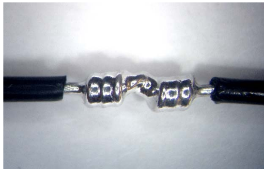
Figure 19-18. Soldered Western Union/Lineman Splice
