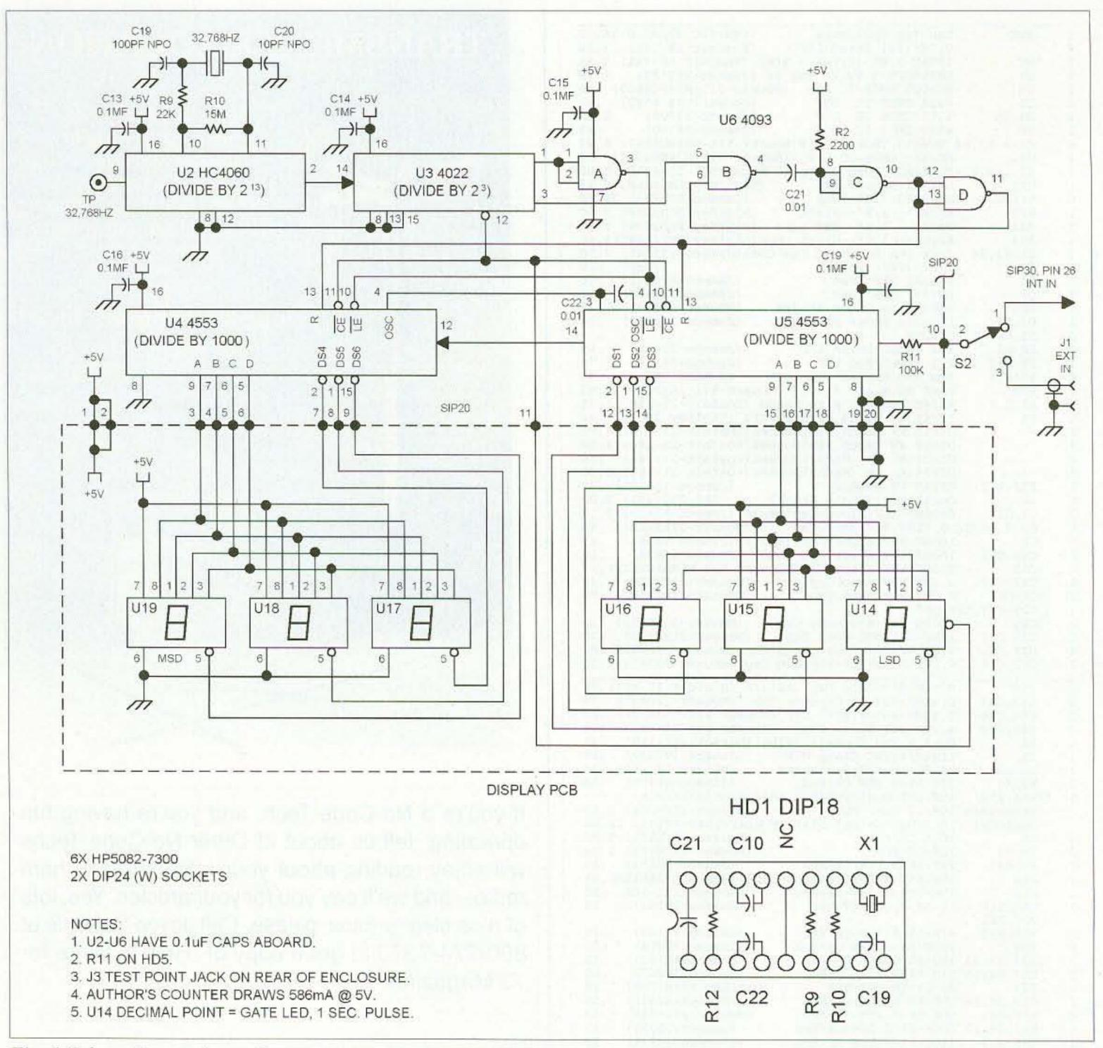
Fig. 4. Schematic, counter section.
