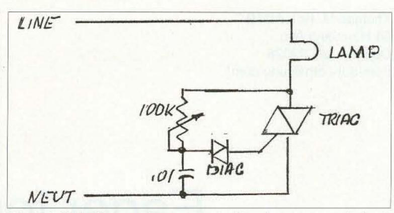
Fig. 2. A light dimmer phase-controls the voltage across the load.
