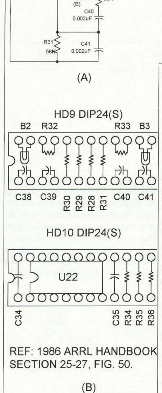
Fig. 9. Schematic, SSB tone test (optional).
