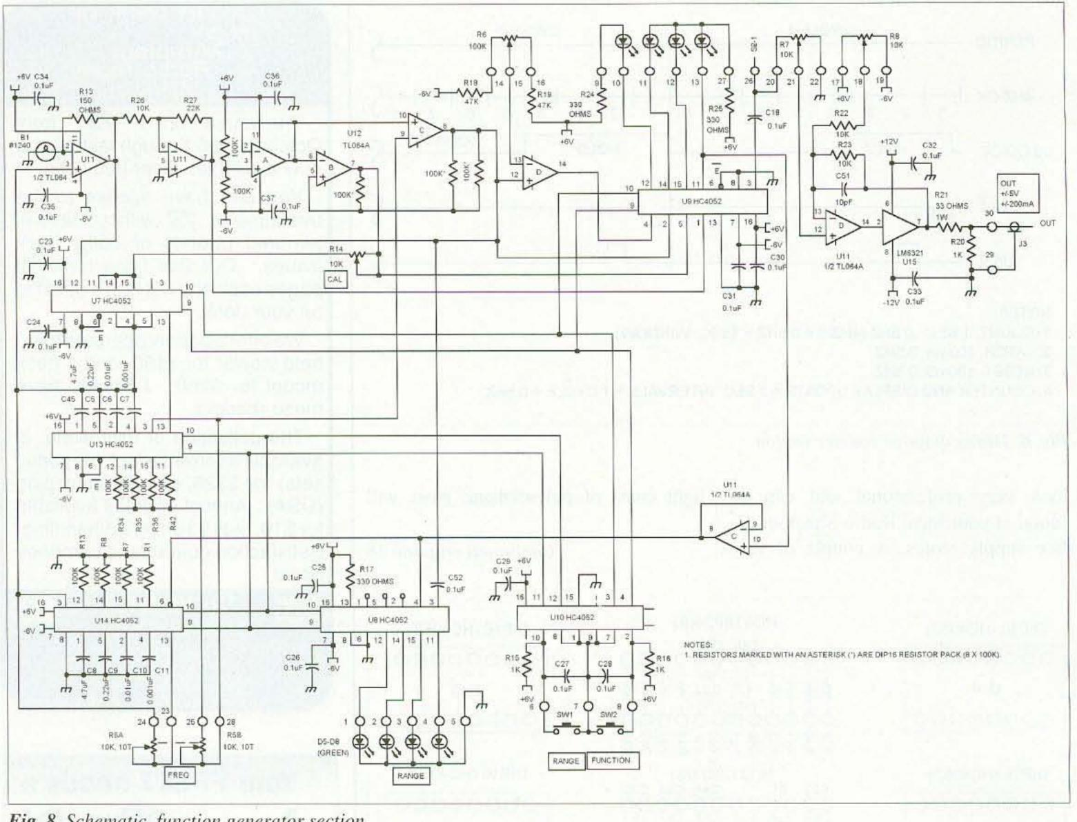
Fig. 8. Schematic, function generator section.
