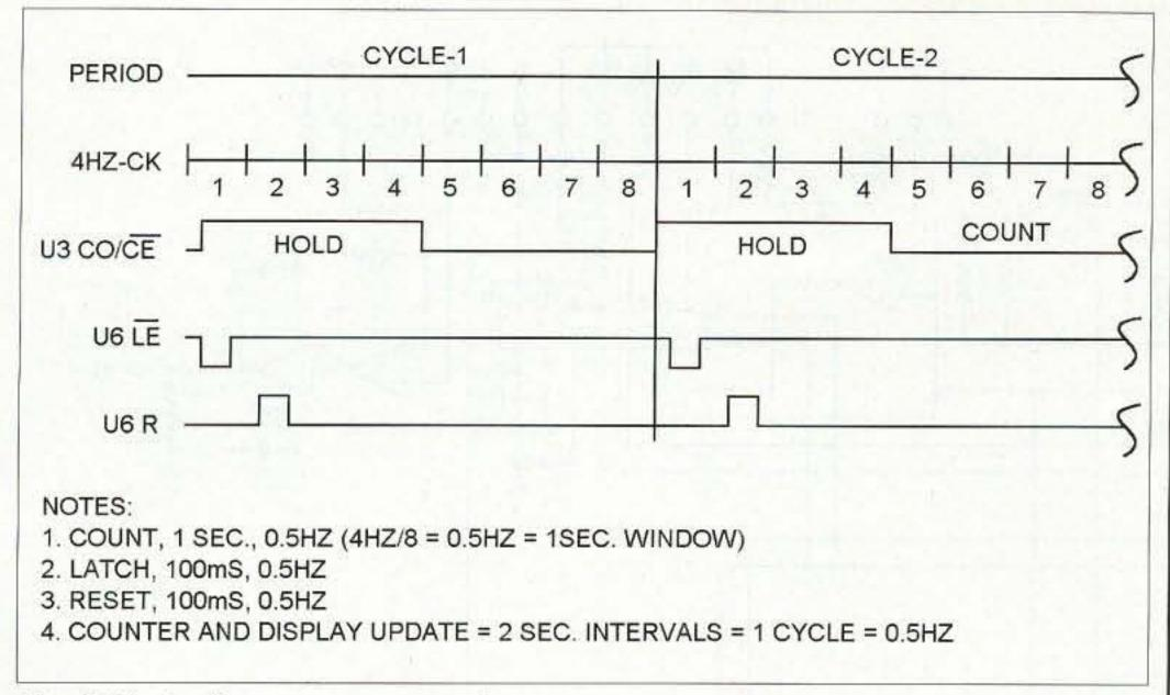
Fig. 6. Timing diagram counter section.
