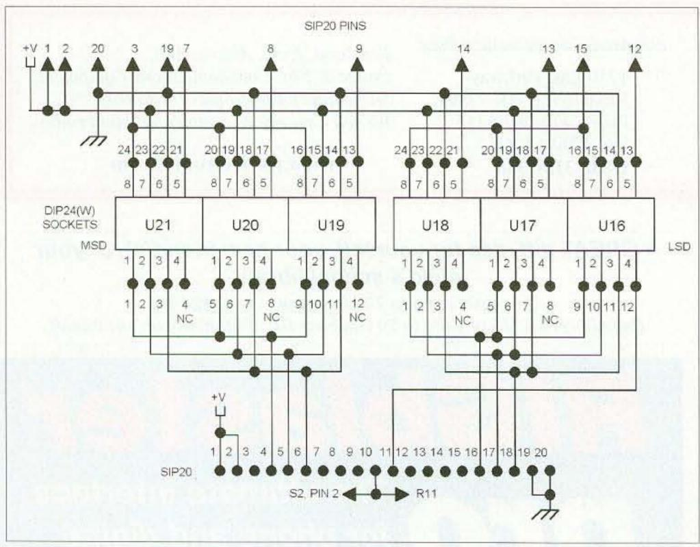
Fig. 5. Schematic, counter display section.
