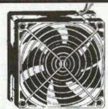
0.6 Amps. 45 Dba max @ 1M. Designed for 50,000 hours @ 25 deg. C. Thermoplastic housing and 7 blade impeller. Three 7" pigtail leads with 3-pin connector (0.1" cntrs). Third lead is for sensing rotation. Prepped with metal finger guard. UL, CSA,CUL, CE. Large quantity available.
