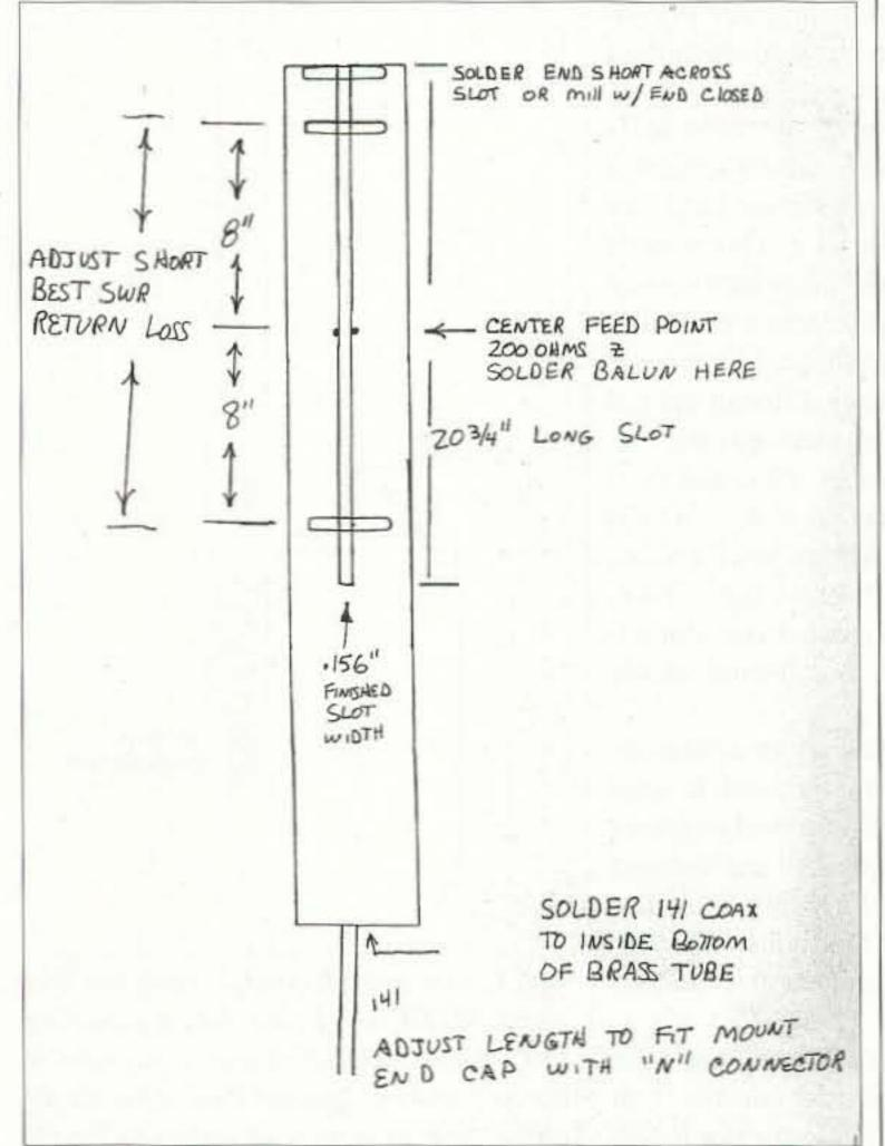
Fig. 3. Slot antenna construction. Note top end of brass tube has short on end. Second short determined when frequency measurements for 1296 made and short placed 8 inches above center feed balun on antenna I constructed. Bottom short same scenario as top short and adjustment short spacing, 8 inches in my construction test.
