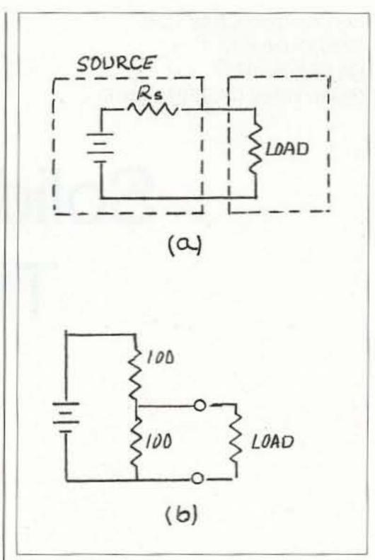
Fig. 2 (a) A battery has internal resistance. (b) A voltage divided source has an internal resistance.
