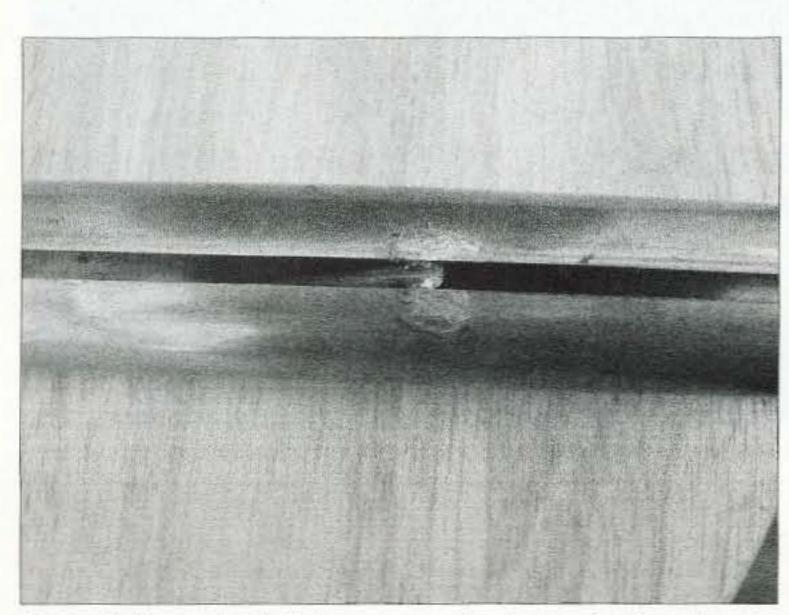
Photo C. Center feed of slot antenna showing each edge of center feed point soldered to 141 balun side contacts, or "leaves."
