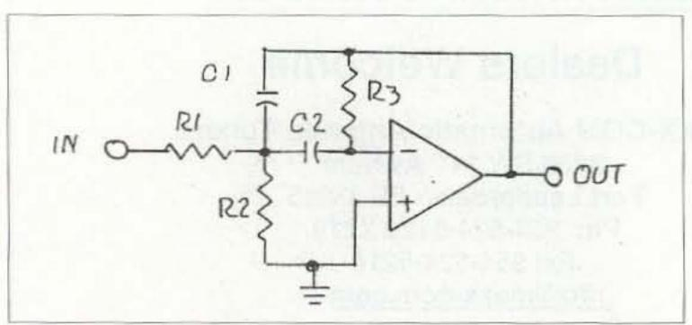
Fig. 1. A single pole active filter uses one op-amp.
