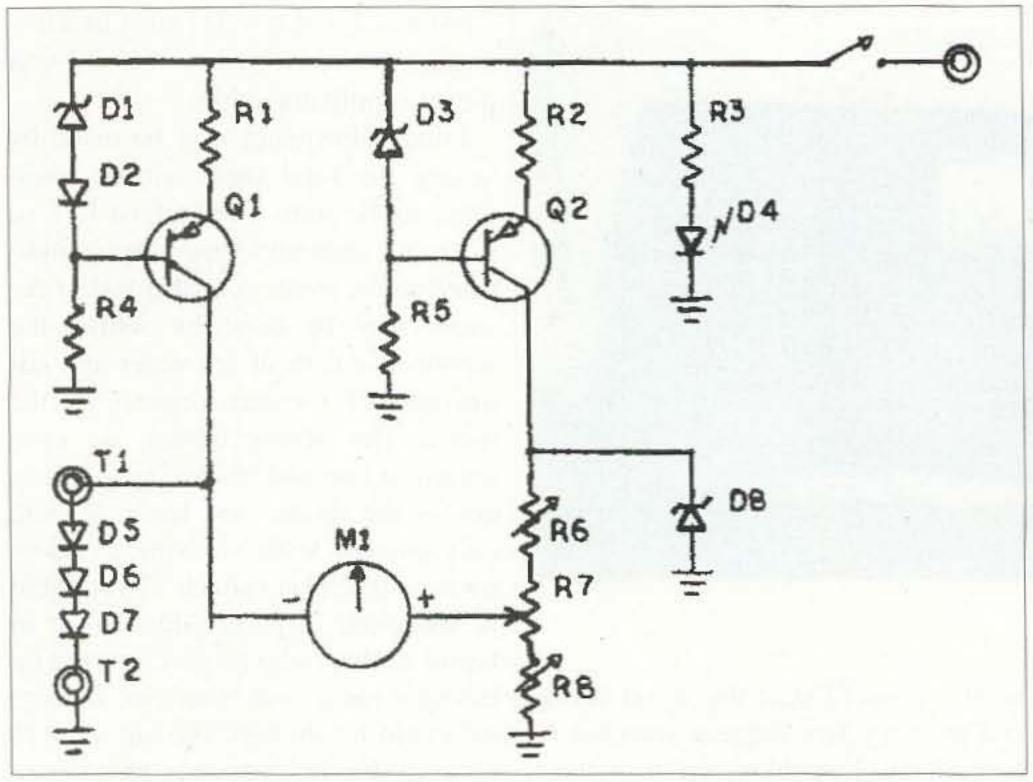
Fig. 2. Digital 0-100° C thermometer.
