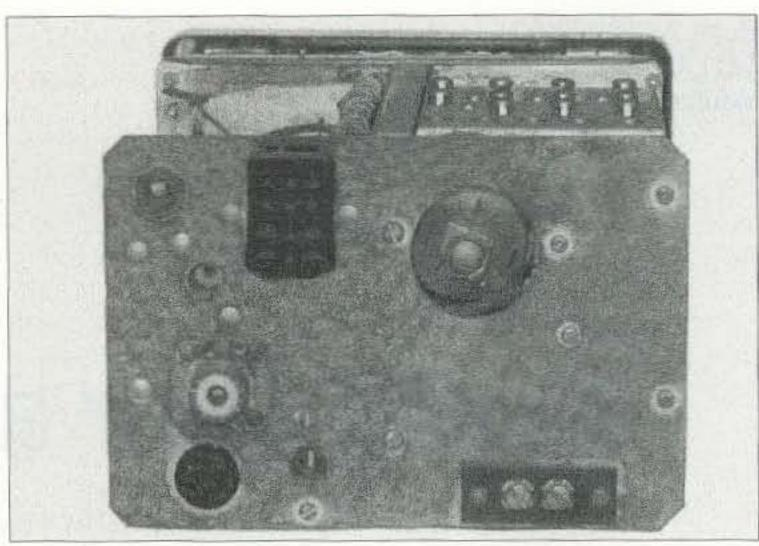
**Photo C.** This is a rear panel view of the transmitter showing the various connectors. Take note of the Jones power connector, antenna connectors, and the terminals for optional low band loading capacitance.
