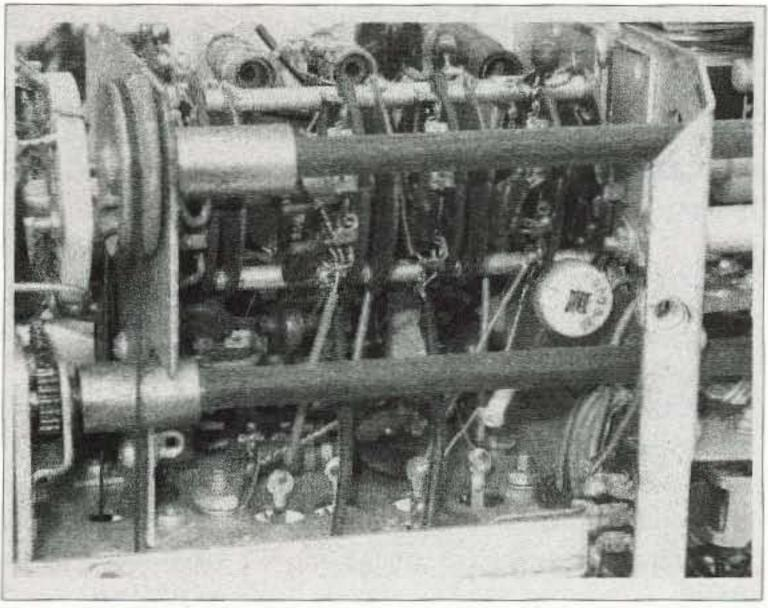
**Photo E.** During tracking alignment, the ceramic trimmer capacitor shown mounted on the band switch wafer is the C value that is adjusted for the 10m band.
