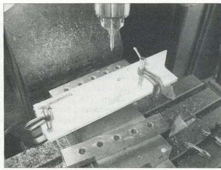
Photo D. To ensure the bearing holes are aligned, clamp the two pieces of angle together and drill simultaneously.
