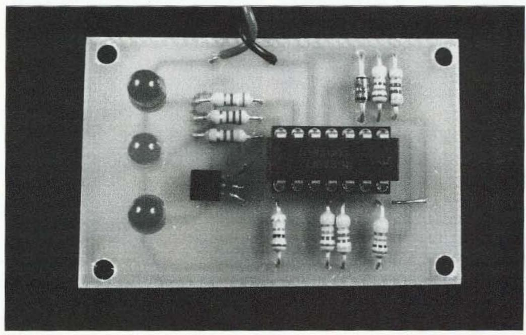
Photo A. Automotive battery voltage monitor.
