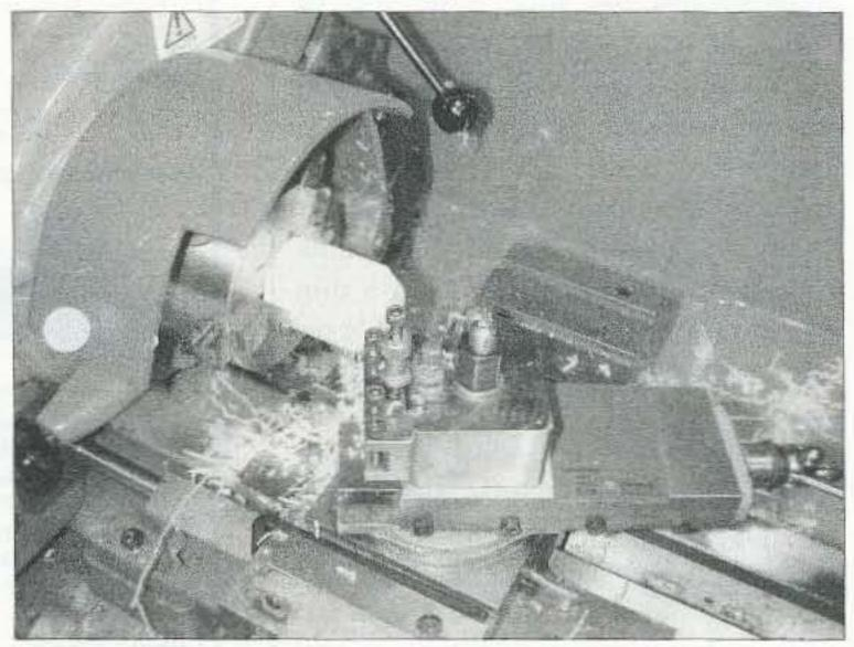
Photo I. Turning the large mandrel cones.
