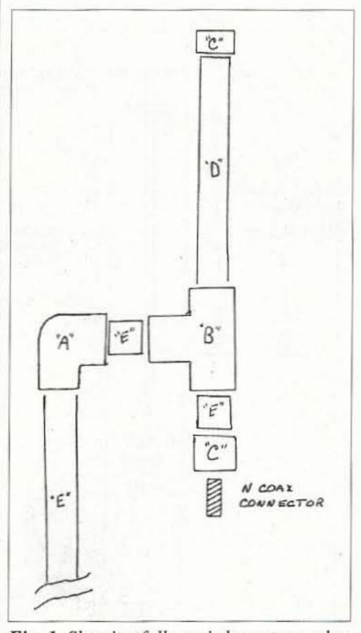
Fig. 1. Showing full omni slot antenna that Kerry N6IZW and I constructed including PVC pipe mount using excess remainder of the inch and one quarter PVC schedule 40 pipe length as a mast to attach to the 90 degree plumbing elbow. A = 90 degree SCHD 40 1-1/4" elbow. B = SCHD 40 1-1/4" "T". C = SCHD 40 1-1/4" end cap. D = 1-1/4" fluorescent light shield "tube guard." E = SCHD 40 1-1/4" PVC pipe.
