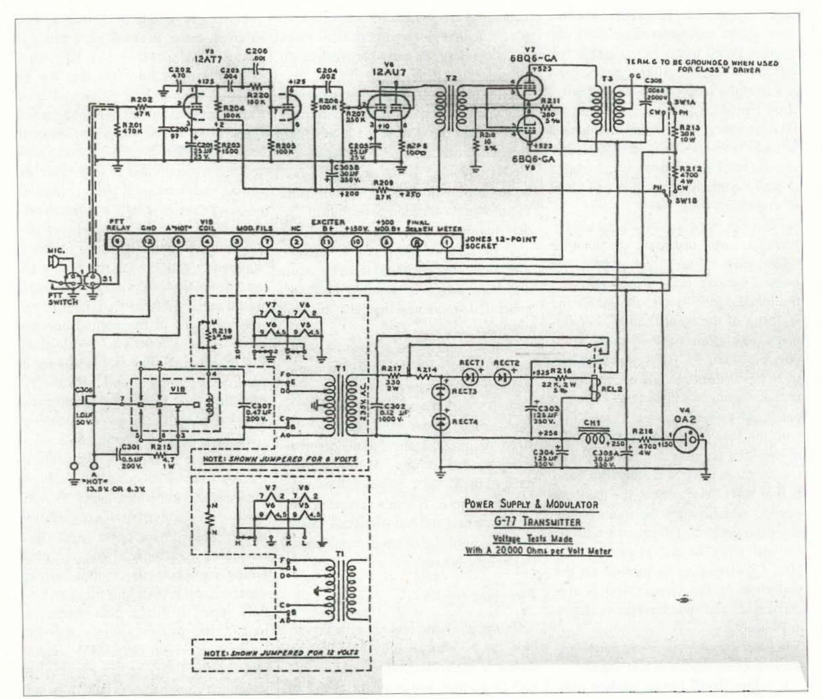
Fig. 1. Modulator-power supply schematic.
