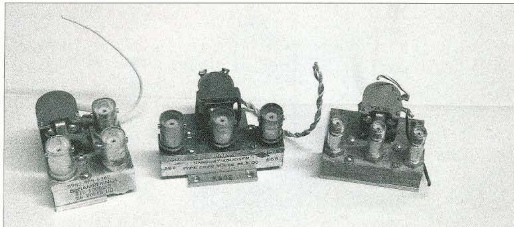
Photo B. Picture of high-loss BNC relay not usable at 1296 MHz (center top), better suited for low frequencies like 50 or 144 MHz. An early SMA version of a better-than-BNC relay, but still not top performer above 1 GHz, is at far right.
