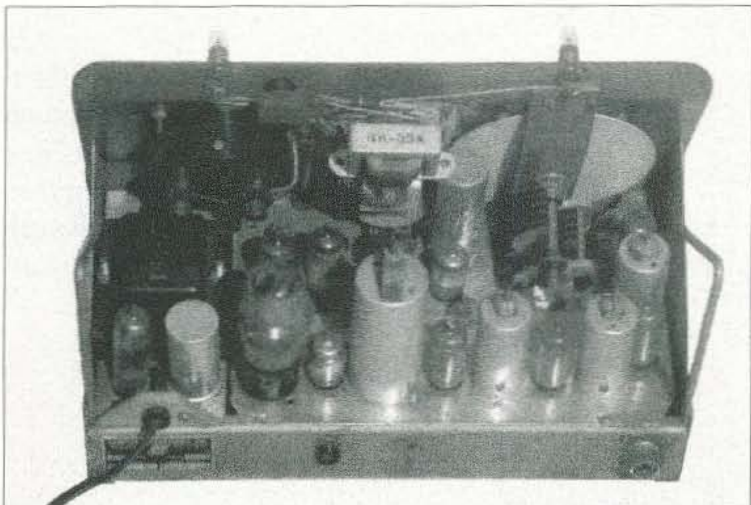
Photo D. An inside top view of the chassis and tube layout.
