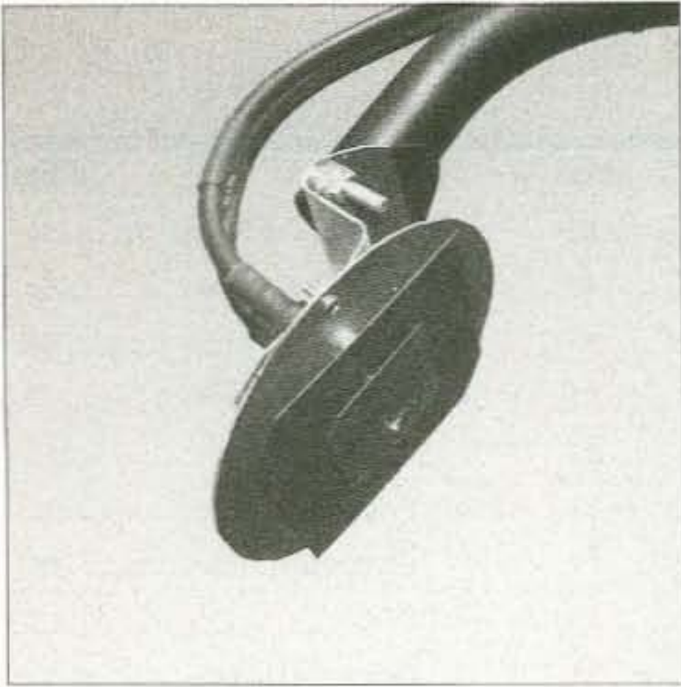
Photo C. Close-up view of the dual band (L & S) circular patch feed on the AO-40 dish.
