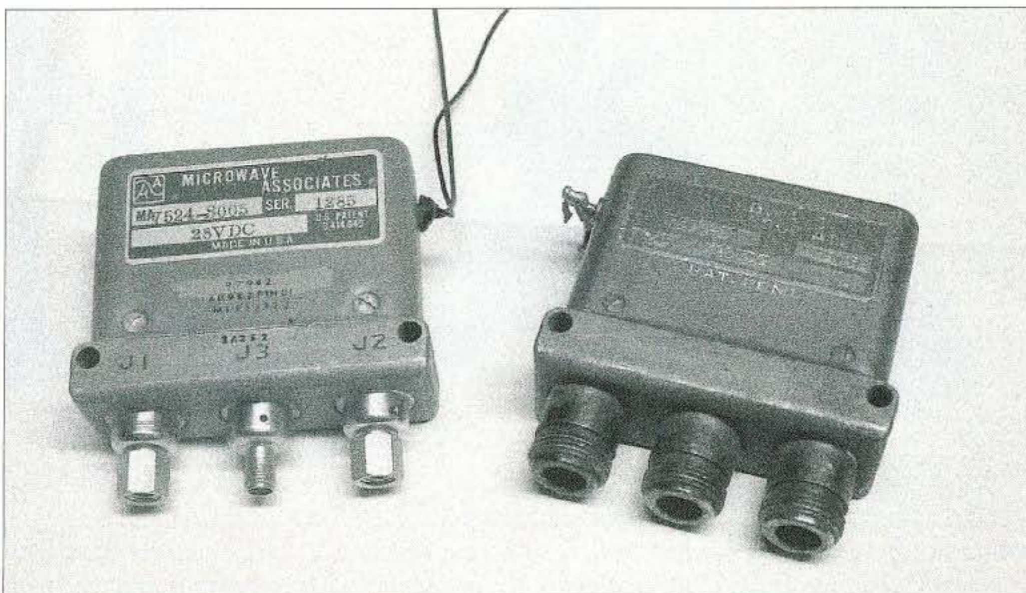
Photo C. Picture of large, high-power “N” connectorized on right, and SMA version of same relay on the left. Both rated to 2 GHz for reasonably good performance. Just large and high-power.
