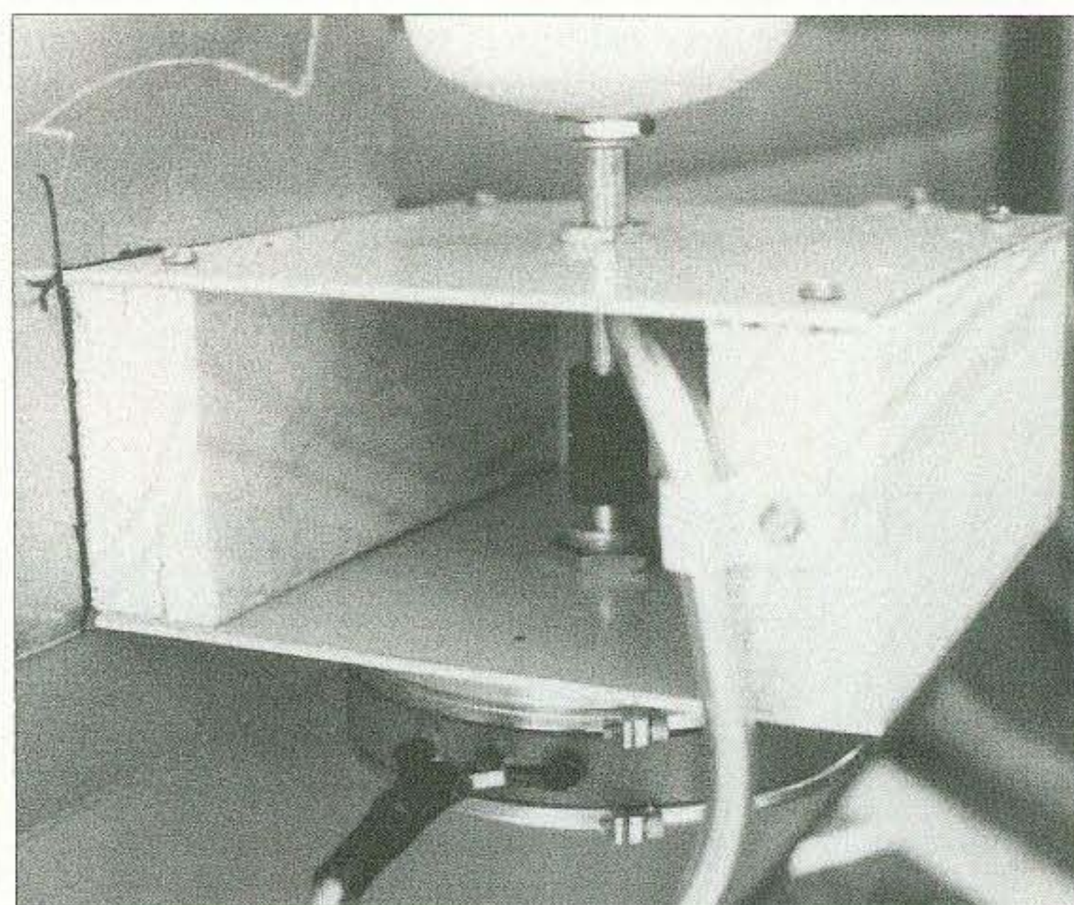
Photo E. This is how Jerry Boyd WB8WFK of Albuquerque attaches the bottom of his mobile antenna mast to the continuous-turning potentiometer that senses azimuth. The pot must be linear-taper with minimum dead zone. The assembly mounts to the inside of the driver-side door.
