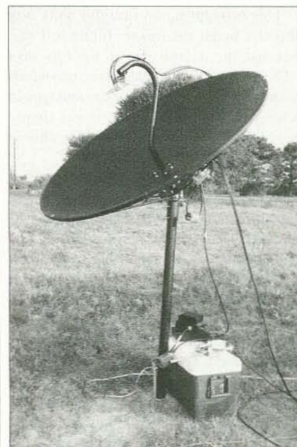
Photo B. An elegant system for L-band uplink and S-band downlink for AO-40 operation during Field Day 2002 at K5OE.
