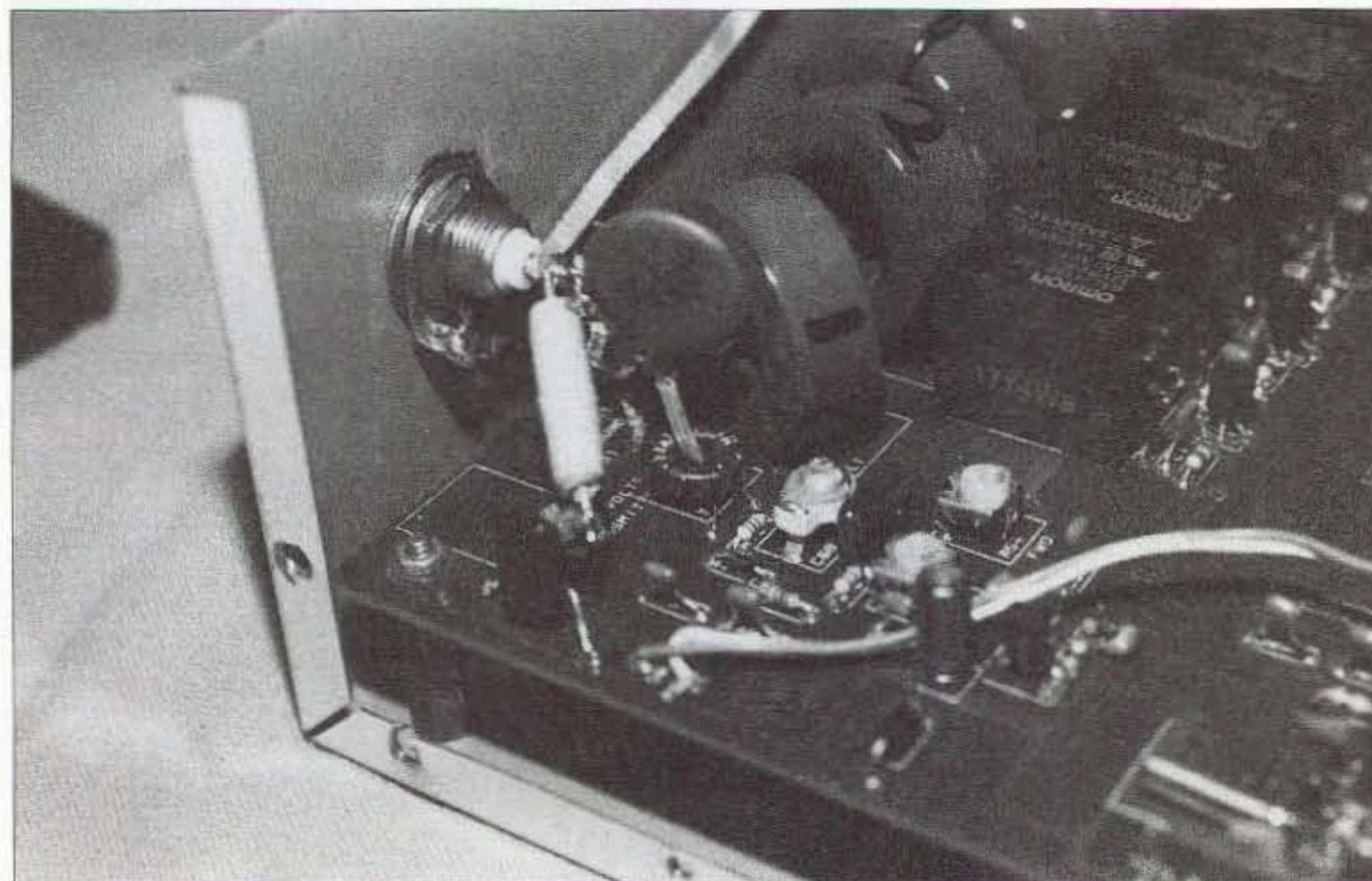
Photo B. The power extractor mounted inside the tuner enclosure, showing one lead of C3 passing through T1, a part of the ATU.
