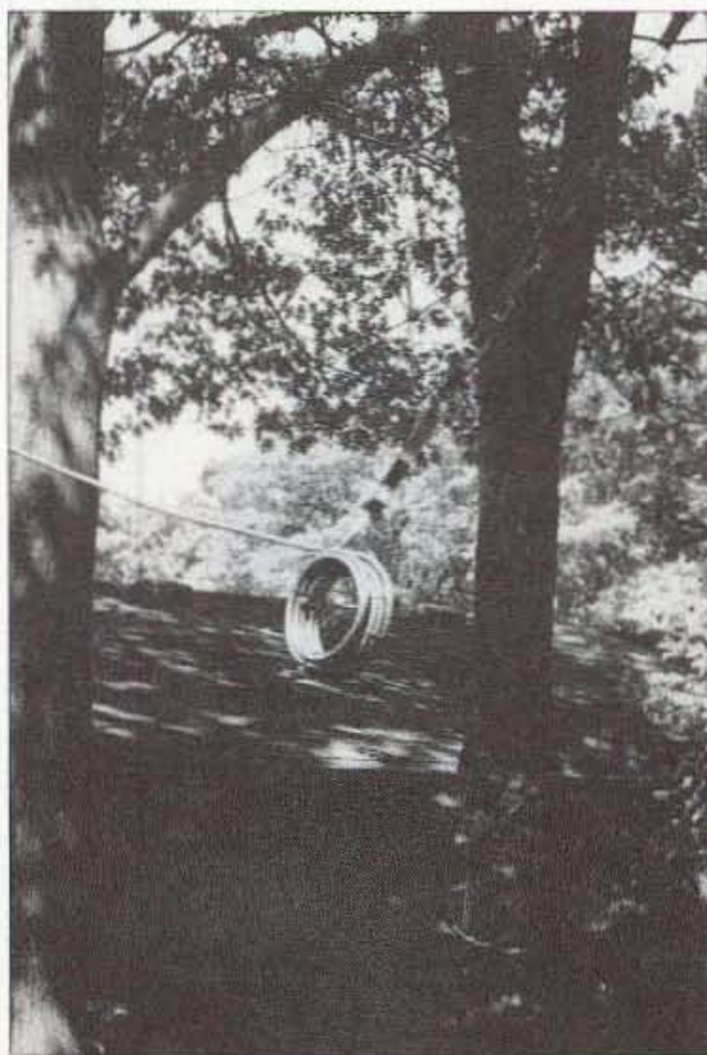
Photo A. The coax balun on my G5RV dipole.
