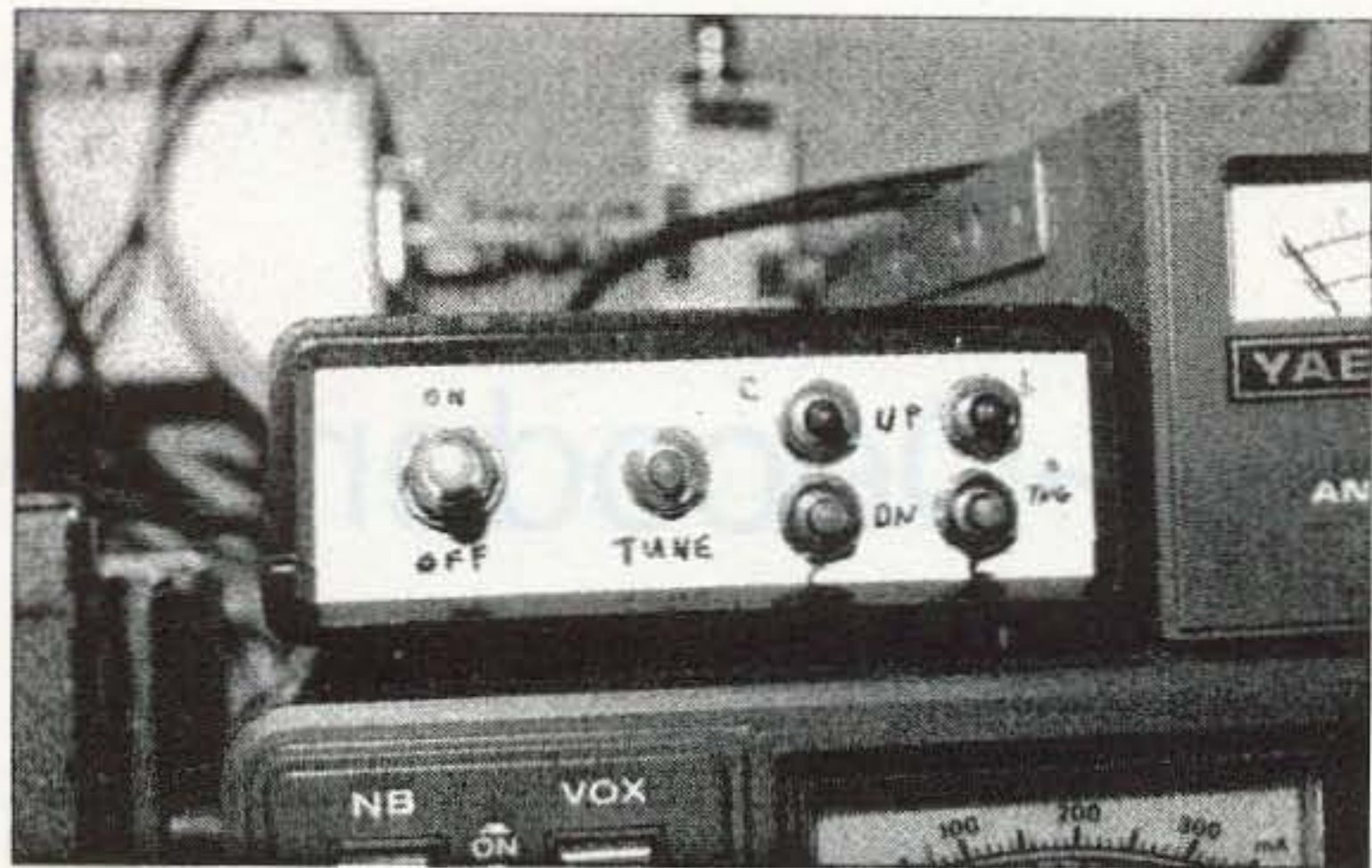
Photo D. Front view of the transmitter, with the TUNE indicator on the right marked TNG.
