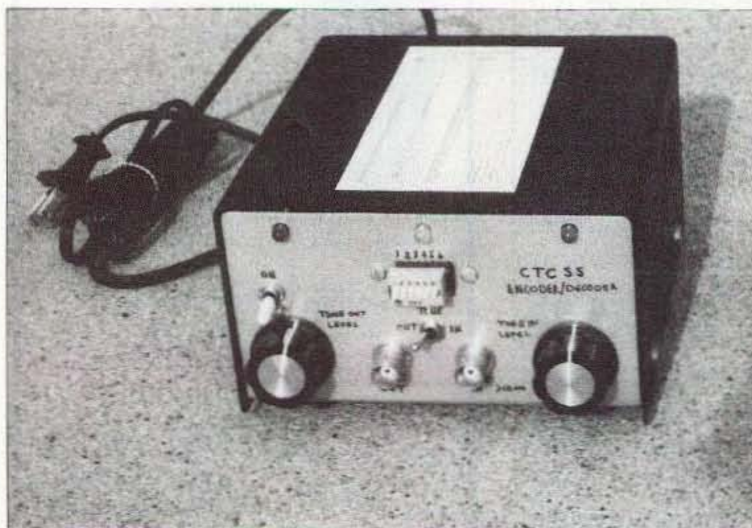
Photo A. This is the completed CTCSS Encoder-Decoder Test Device.
