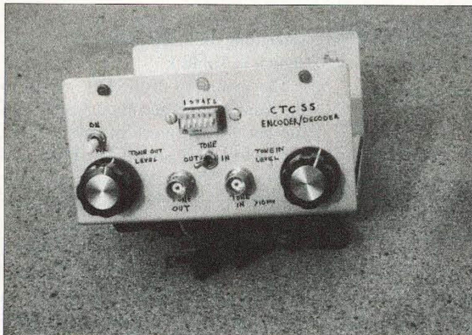
Photo C. This is the front panel showing parts placement. A 6-pin DIP switch is used for selecting one of 64 CTCSS frequencies.
