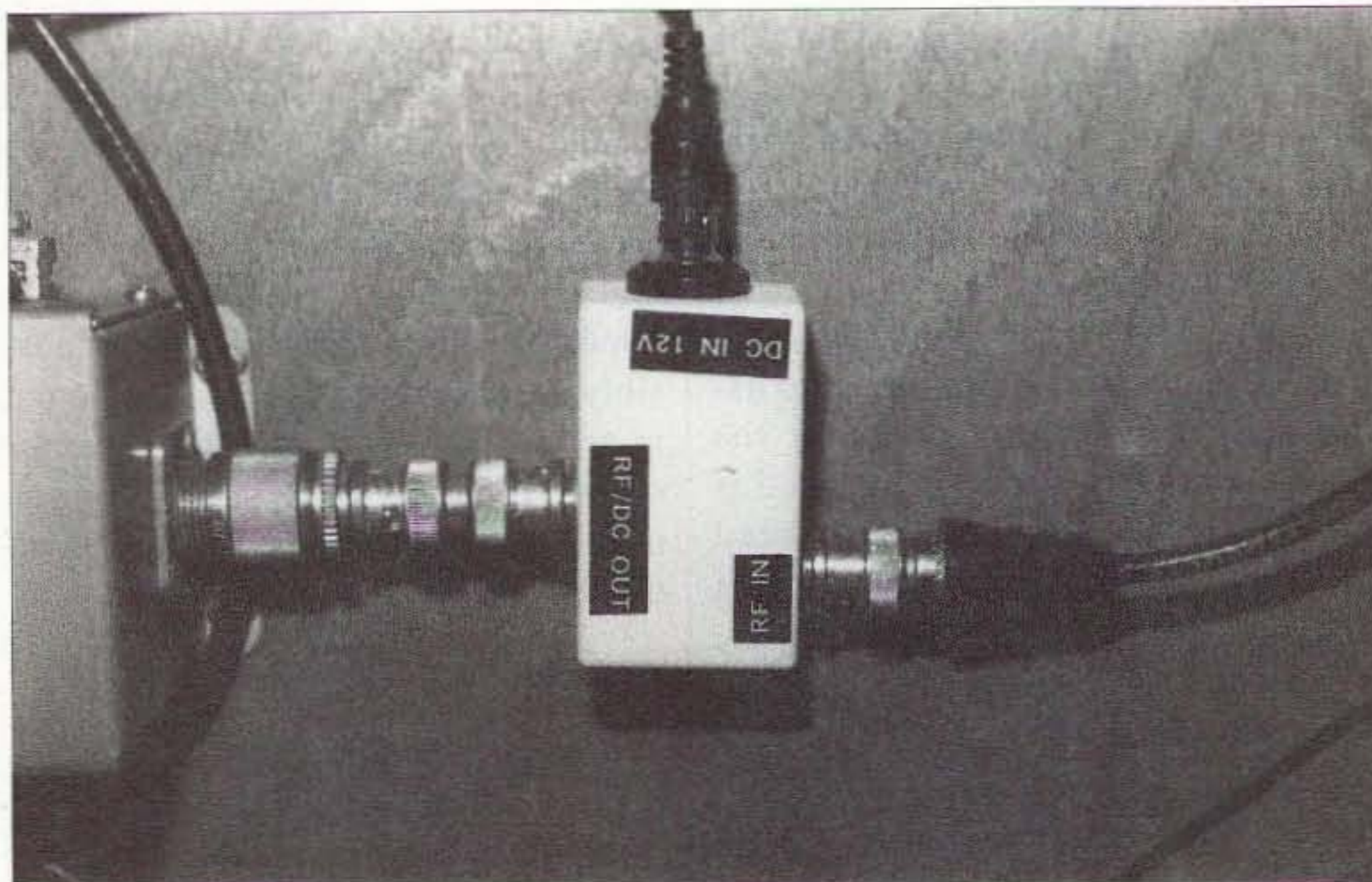
Photo A. The finished power injector. DC is derived from the HF transceiver but can be from any source. (Photos by author)
