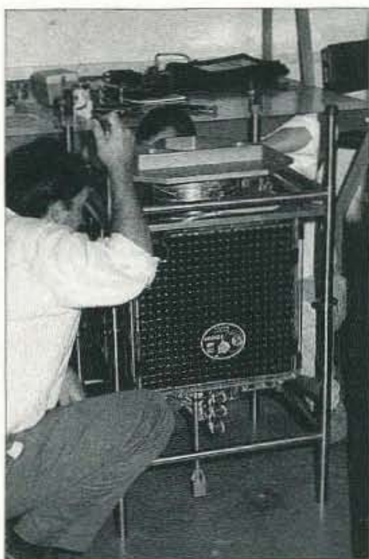
Photo D. In the lab at the University of Stellenbosch, SUNSAT gets a fit check with the Payload Adapter Assembly (PAA) and associated hardware.
