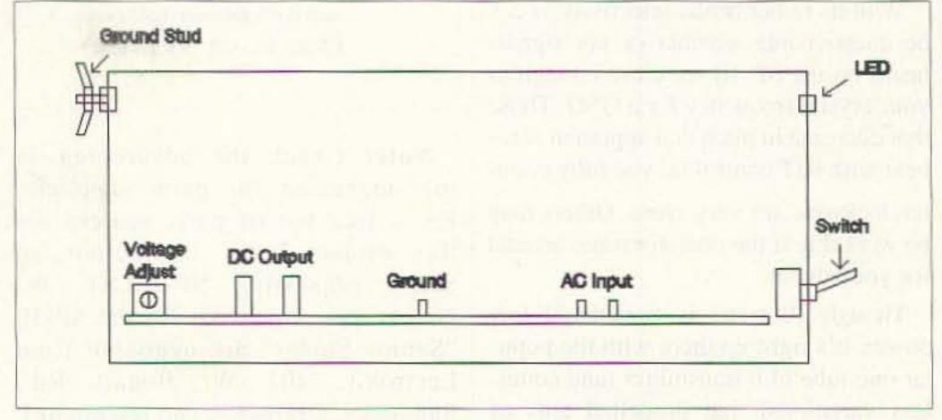
Fig. 1. Switching power supply side view.
