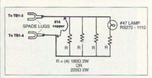
Fig. 5. Terminating RF detector.
