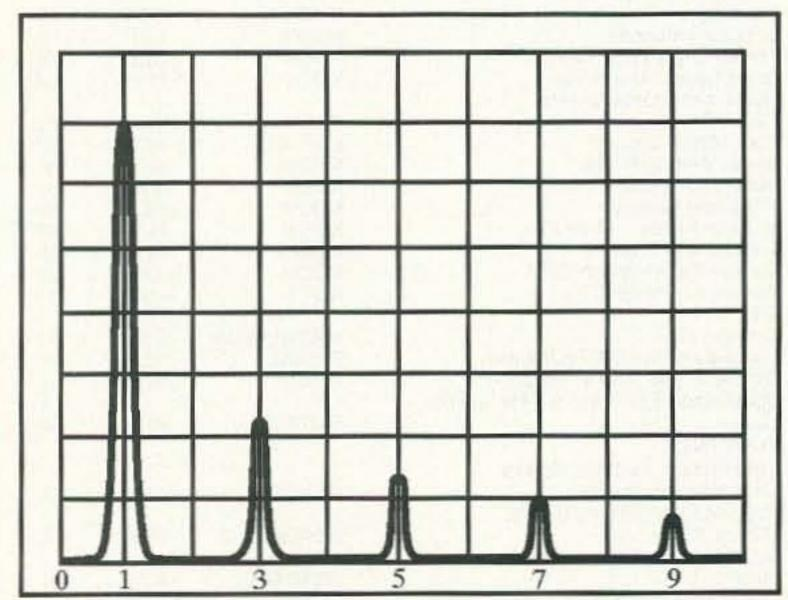
Fig. 12. Spectrum of a 1,000-Hz square wave.
