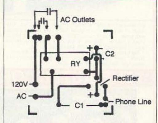
Fig. 2. The component side of the board, showing parts placement.
