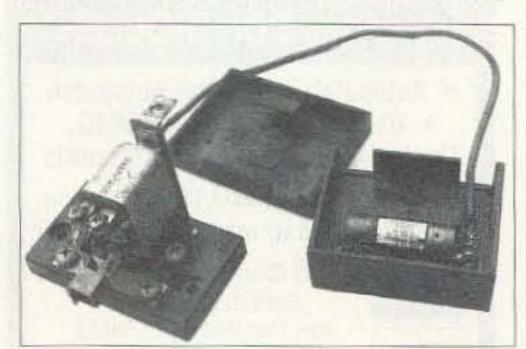
Photo A. Typical control relay and fuse block suitable for use with 100-watt mobile radios.
