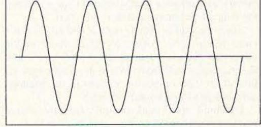
Fig. 5. Whistle waveform an octave higher than that in Fig. 4.
