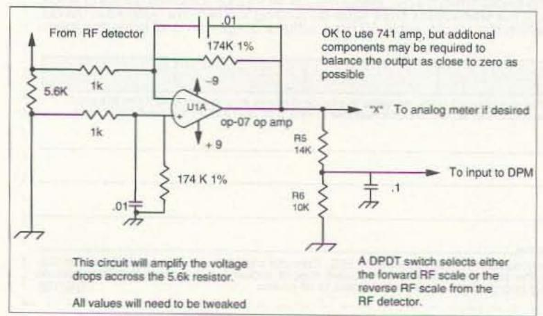
Fig.1. Schematic of the DPM.
