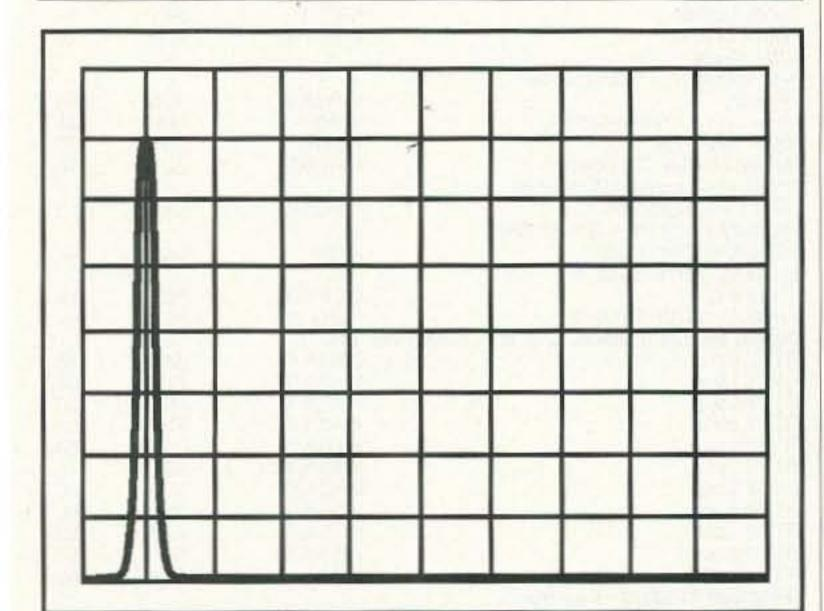
Fig. 11. Spectrum of a 1,000-Hz sine wave.
