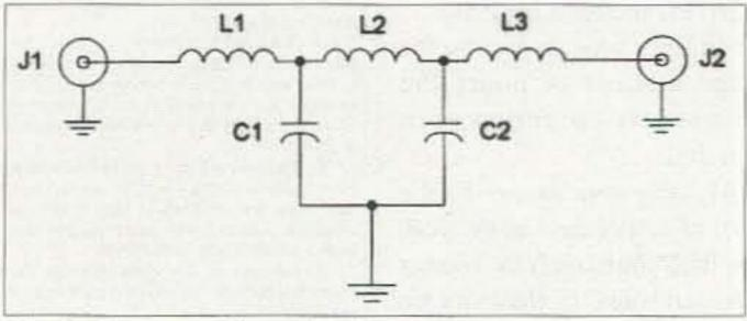
Fig. 2. Low-pass filter circuit.
