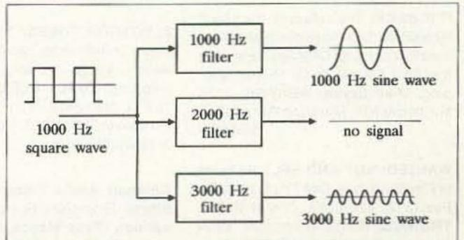
Fig. 9. Separating a square wave into components.
