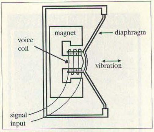
Fig. 3. A telephone-type earphone.
