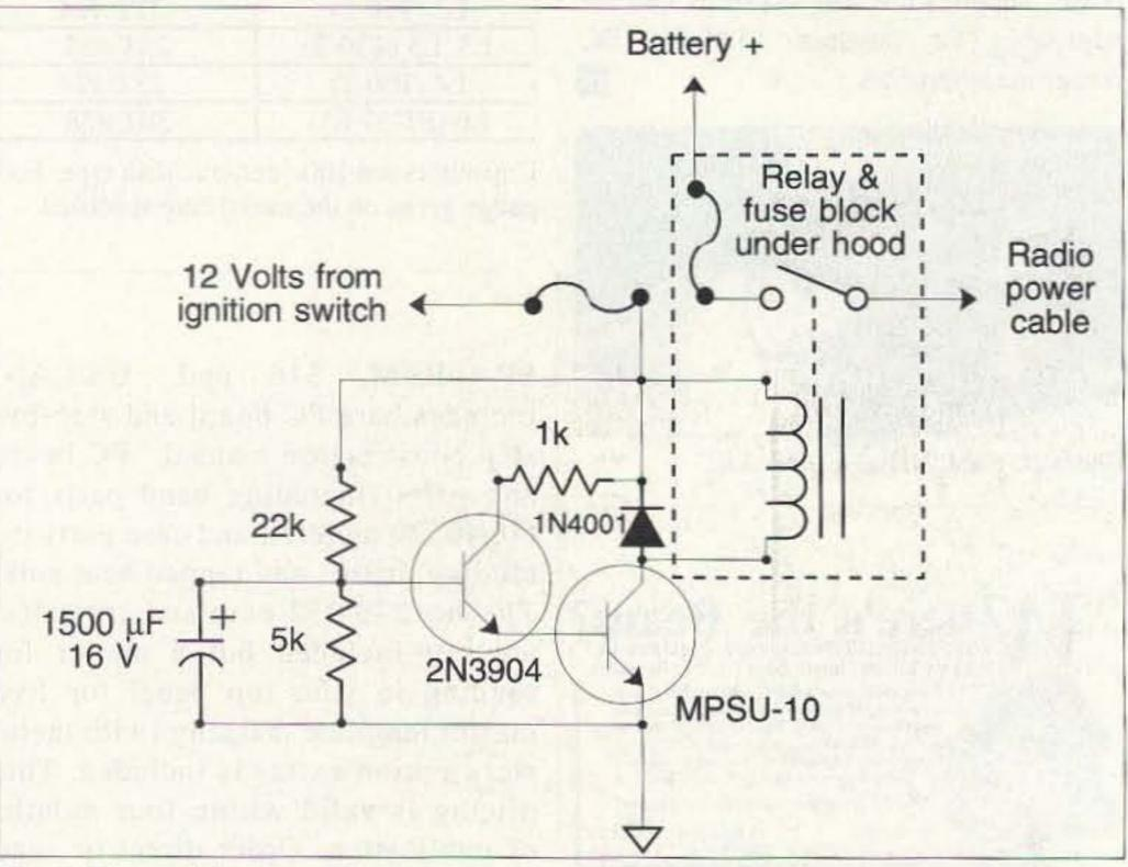
Fig. 1. The on-delay timer circuit.
