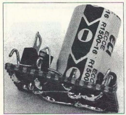
Photo B. The on-delay timer construction details.
