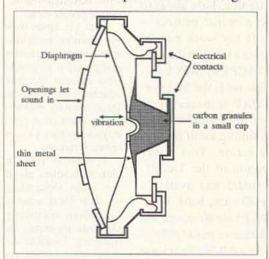
Fig. 1. Telephone-type carbon microphone.
