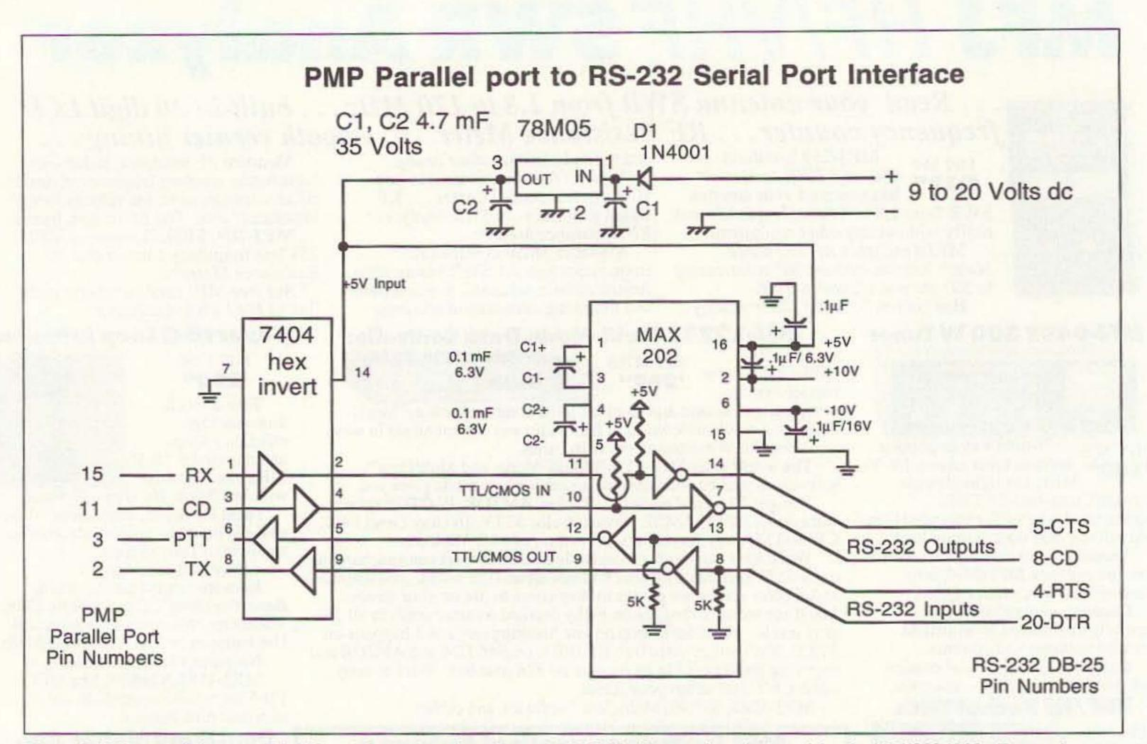
Figure 2. PMP parallel port to RS-232 serial port interface. Note: A MAX232 chip may be substituted for the MAX202 if 10 µF capacitors are used throughout.
