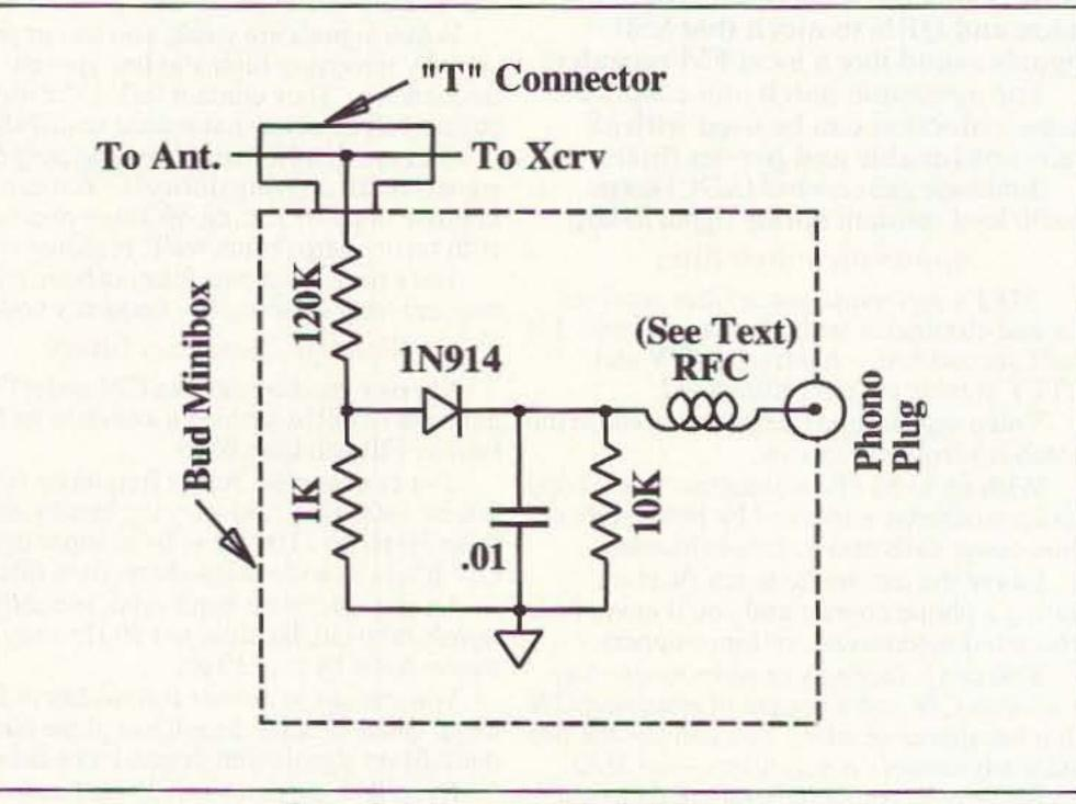
Figure 2. Schematic for the RF Sampler.
