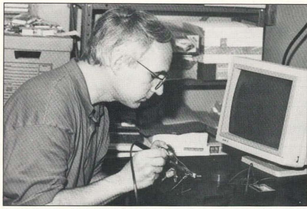
Photo A. Carefully wire the RS-232 lines between the modem and the computer. The wiring is different from standard modem communications.
