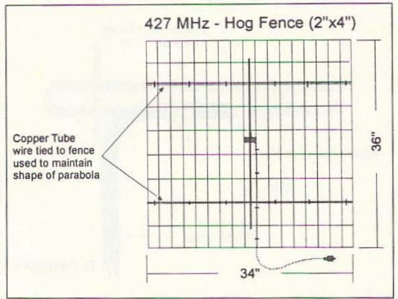
Figure 3. Final assembly of component parts of the Hog Fence antenna. The copper tubing is wire tied to the hog fence reflector to maintain parabolic shape.
