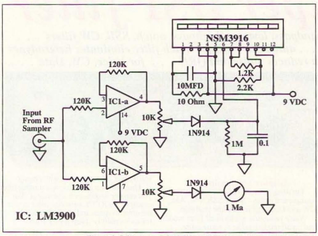
Figure 1. Schematic of the RF Power Meter.
