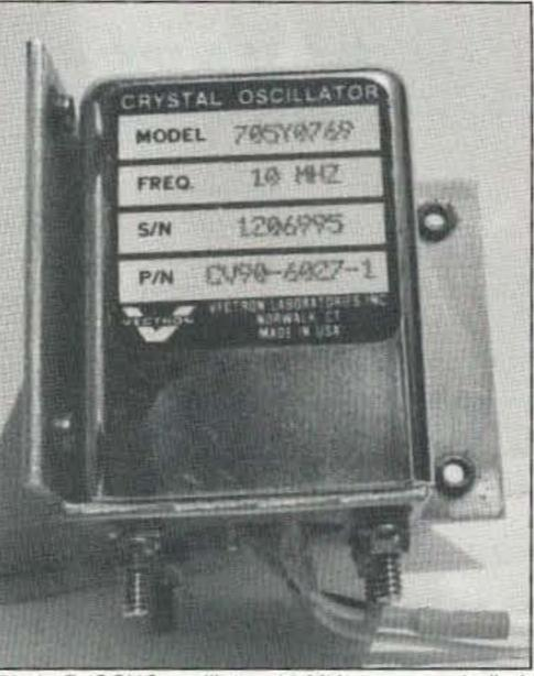
Photo B. OCXO oscillator: 10 MHz, oven controlled.
