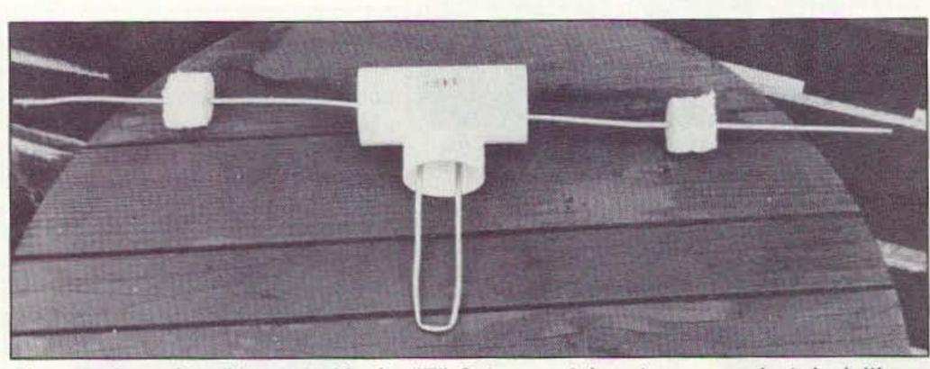
Photo B. Once the tubing is inside the "T" fitting, straighten it out to make it look like an antenna.
