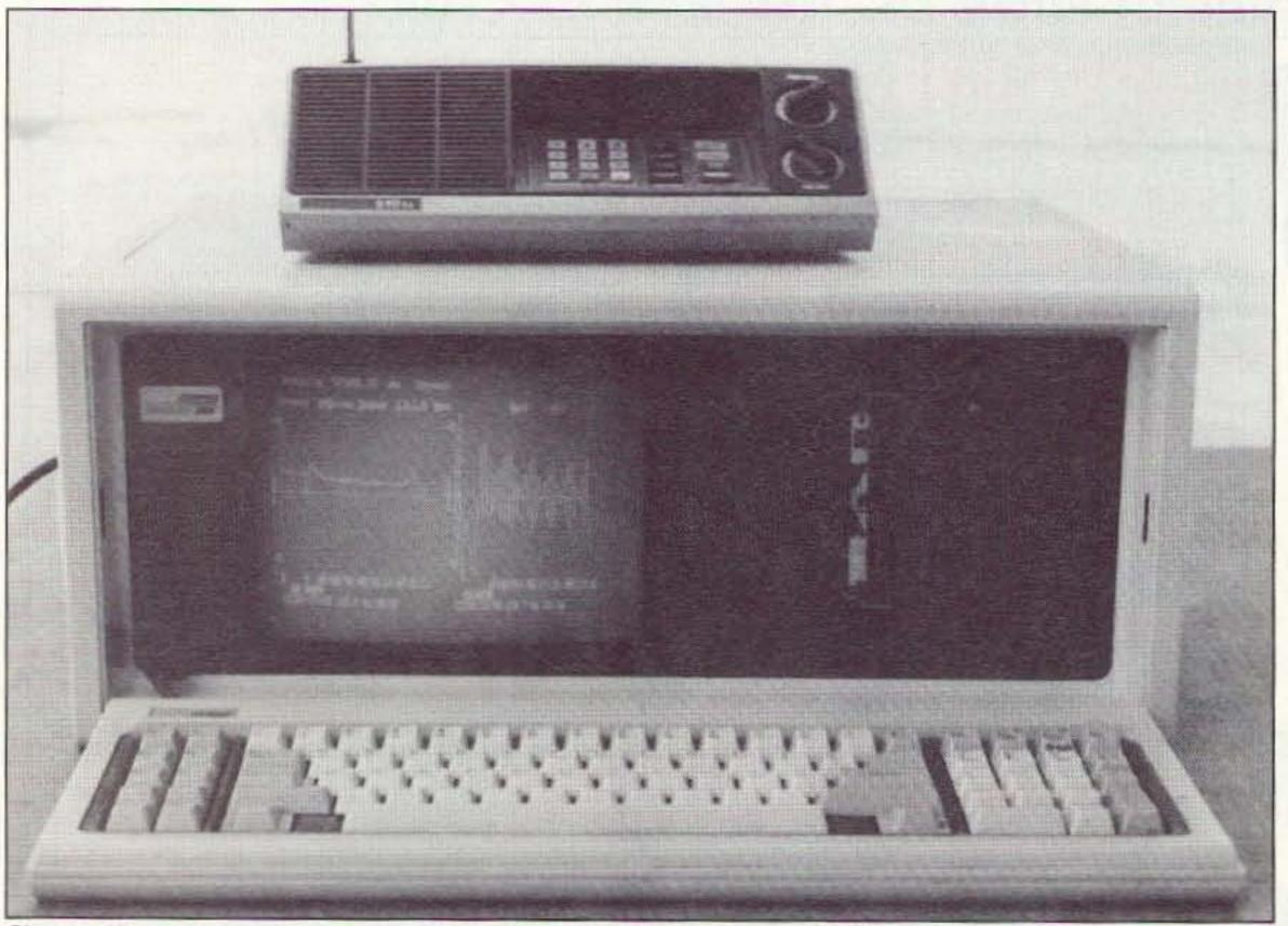
Photo A. All you need to take transmitter fingerprints is a suitable receiver and a computer with the TxID-1 hardware and software installed. Not shown is an optional tape recorder for documenting audio and fingerprints simultaneously.
