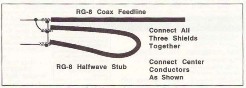
Figure 2. Half-wave phasing section detail.
