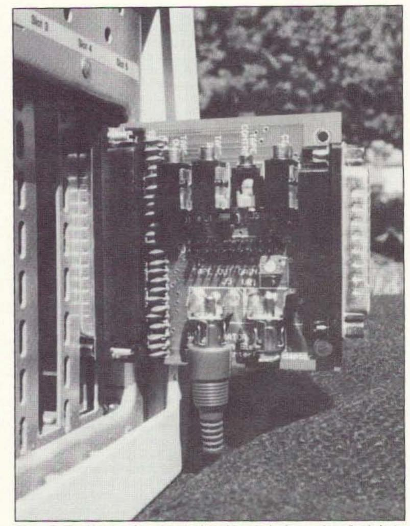
Photo B. The IA-1 Interface Adapter board has jacks for receiver discriminator and S-meter input, plus tape recorder on/off and audio. It attaches to the TxID-1
