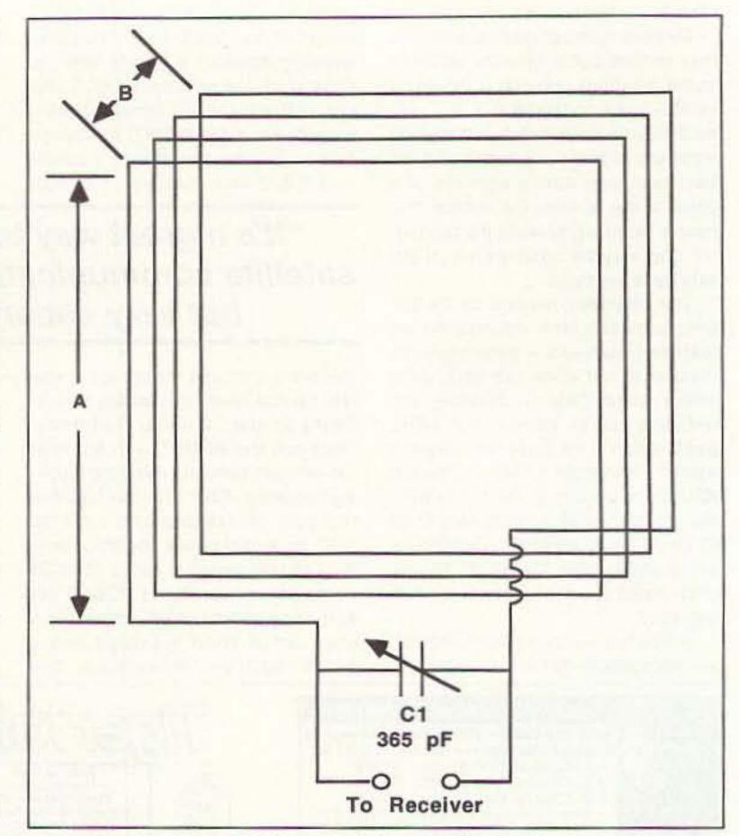
Figure 1. Schematic of the square loop antenna.
