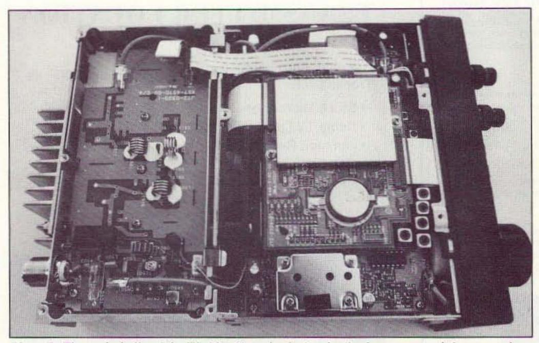
Photo B. The underbelly of the TS-60S. Note the fan's edge in the center, and the output lowpass filter and antenna T/R relay on the output board. The shiny round thing is a 3V battery used for memory backup.
