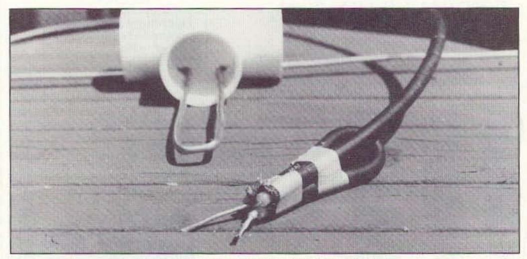
Photo C. Use coax to make the phasing section.
