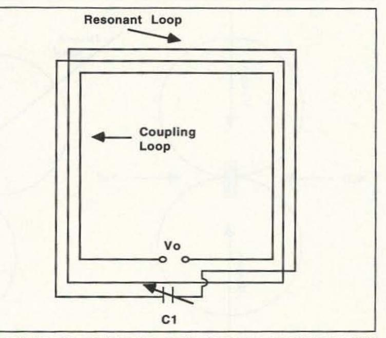
Figure 3. Use of a one-to-two-turn coupling loop improves performance of the loop antenna.
