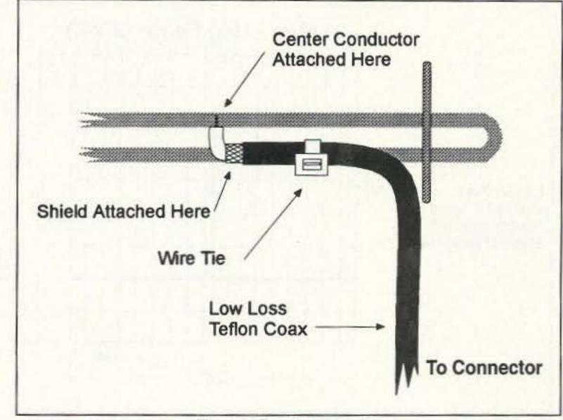
Figure 2. Feedline assembly.
