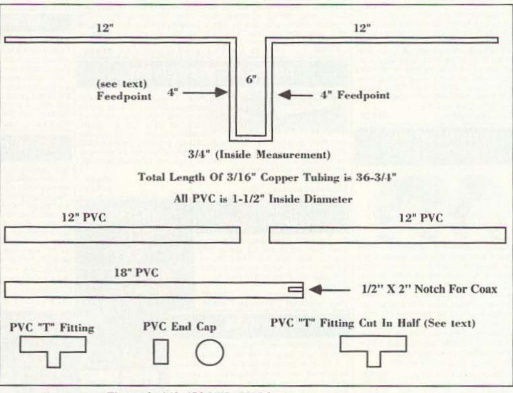
Figure 1. 440-450 MHz PVC base or repeater antenna.
