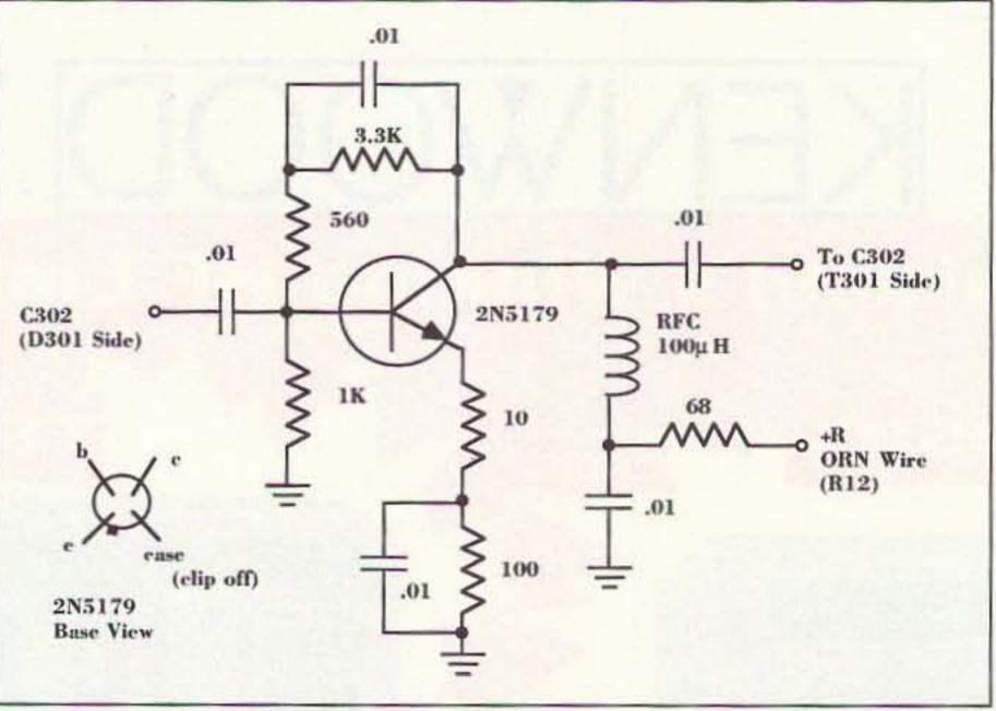
schematic. (See Figure 1.) You will find it standing on end, near T301. Now, carefully cut the lead of C302, leaving it long enough on both sides to tacksolder short wires to. (See Figure 2.) This will be your input and output connection to install the preamplifier. Figure 1 is the schematic for the preamp. Use a 2N5179 or any other low noise high frequency NPN transistor you may have. The circuit is small and lightweight. I just used point-to-point wiring on a 1" x 1-1/2" piece of perf-board.
