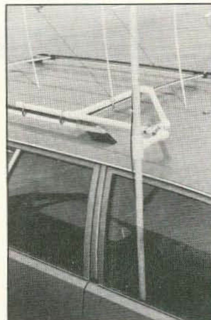
Photo B. WAØRWS devised this roof rack mount because the rigid headliner in his wagon eliminated the possibility of a through-roof hole. Note the plastic panel to keep weather out.
