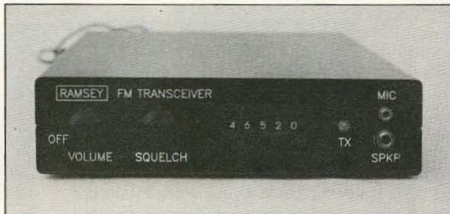
Photo A. Modified front panel of the Ramsey FX-146 2 meter FM transceiver showing the thumbwheel frequency switches.
