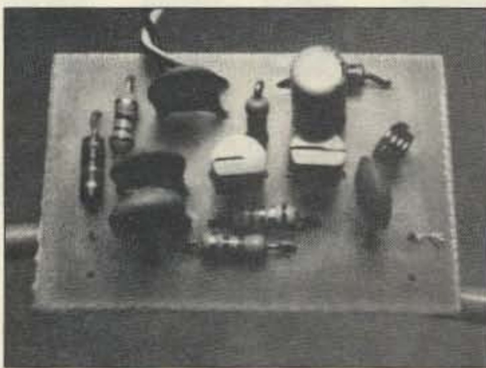
Top view of the assembled Ramsey SA-7 broadband RF amplifier.
