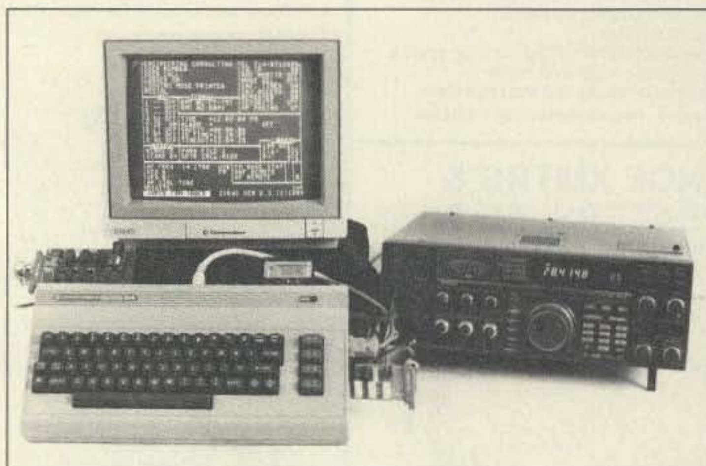
Photo B. The Ultra ComShack 64, with the software on the cartridge, installed in the Commodore 64. The program Main Menu is displayed on the monitor. The IC-761 is the remote HF base (not yet entered as remote #1 on the Main Menu).
