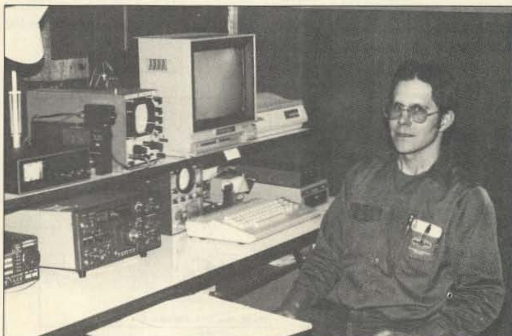
Photos C,D. Greg KE0UV getting ready to to spot some DX on 10m using the $10 Spectrum Analyzer. Photo D is a close-up of the system, comprised of the o'scope, the scanning receiver (the DX-360) and the interface, which sits atop the DX-360.
