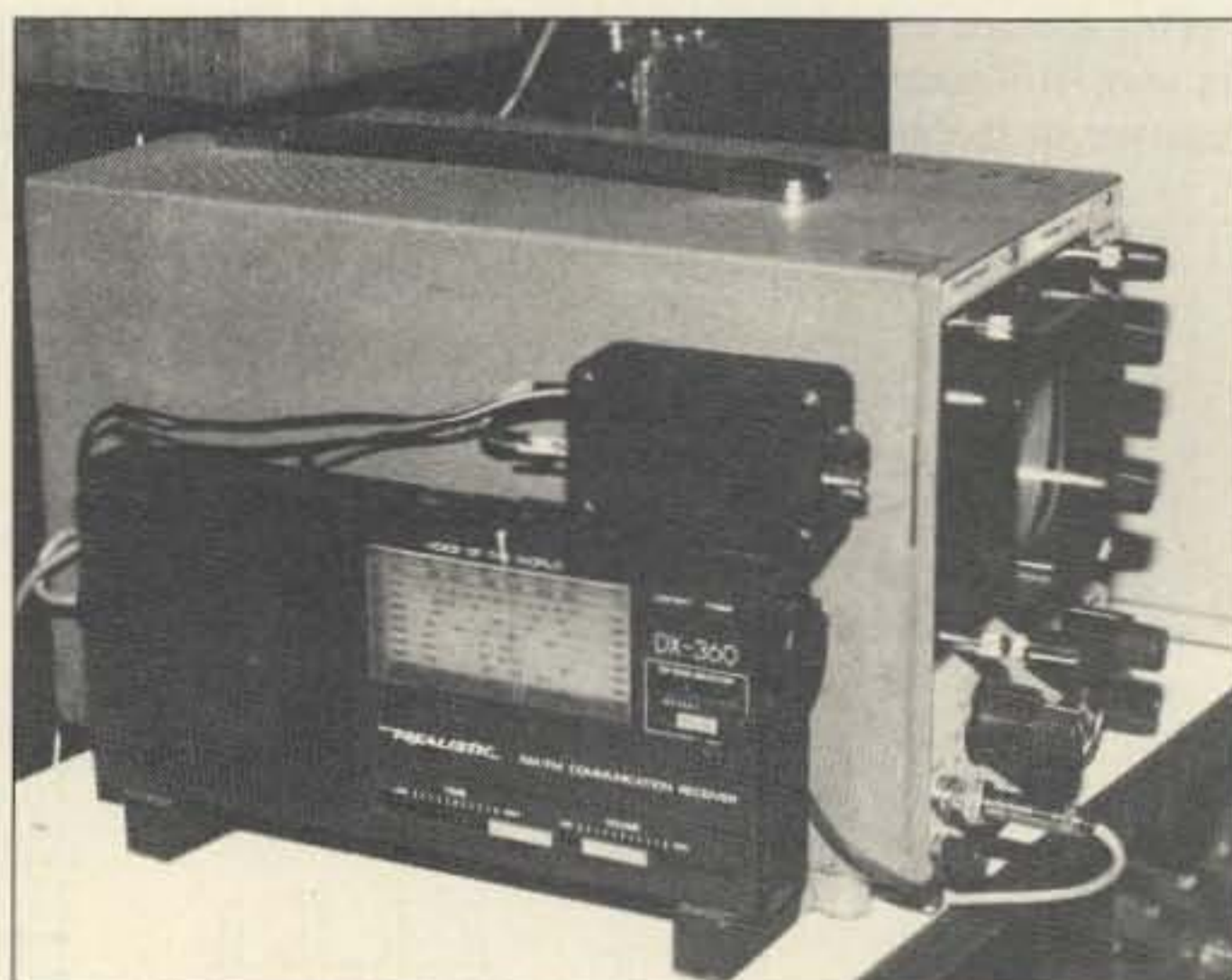
Photos C,D. Greg KE0UV getting ready to to spot some DX on 10m using the $10 Spectrum Analyzer. Photo D is a close-up of the system, comprised of the o'scope, the scanning receiver (the DX-360) and the interface, which sits atop the DX-360.
