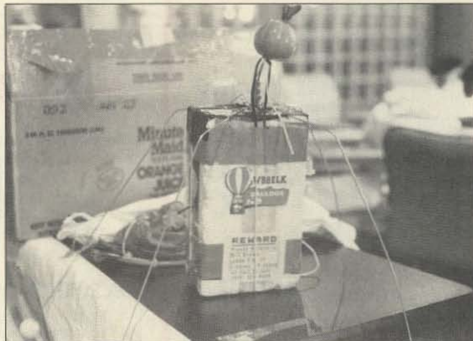
Photo C. Bill Brown WB8ELK's micro-balloon experiment included a 2m transmitter with internal batteries and attached ground plane antenna.
