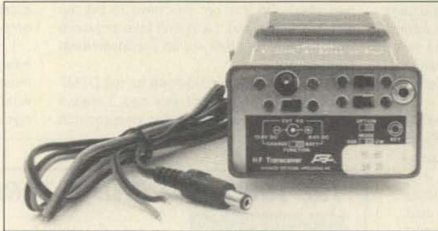
Photo A. Front and top panel of the DX Handy. This 5 1/2" x 2 1/2" x 1 1/2" 6m 1 Watt SSB/CW transceiver weighs less than 2 pounds!
