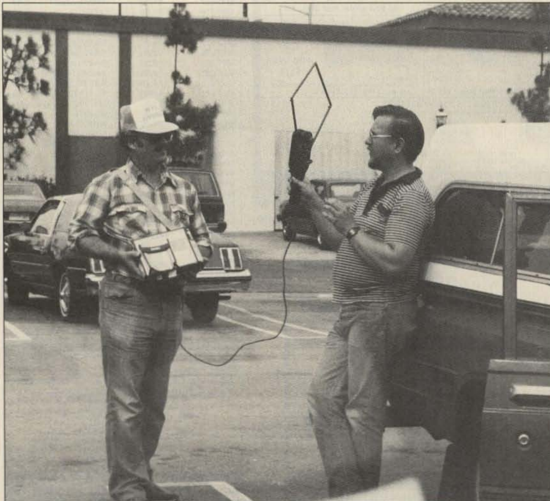
The surplus AT-339/PRC loop and a portable receiver make a nice mobile or hand-carried RDF system for 6 meters. George Stokes WT6U and Bob Miklos K6LPF are ready to hunt.
