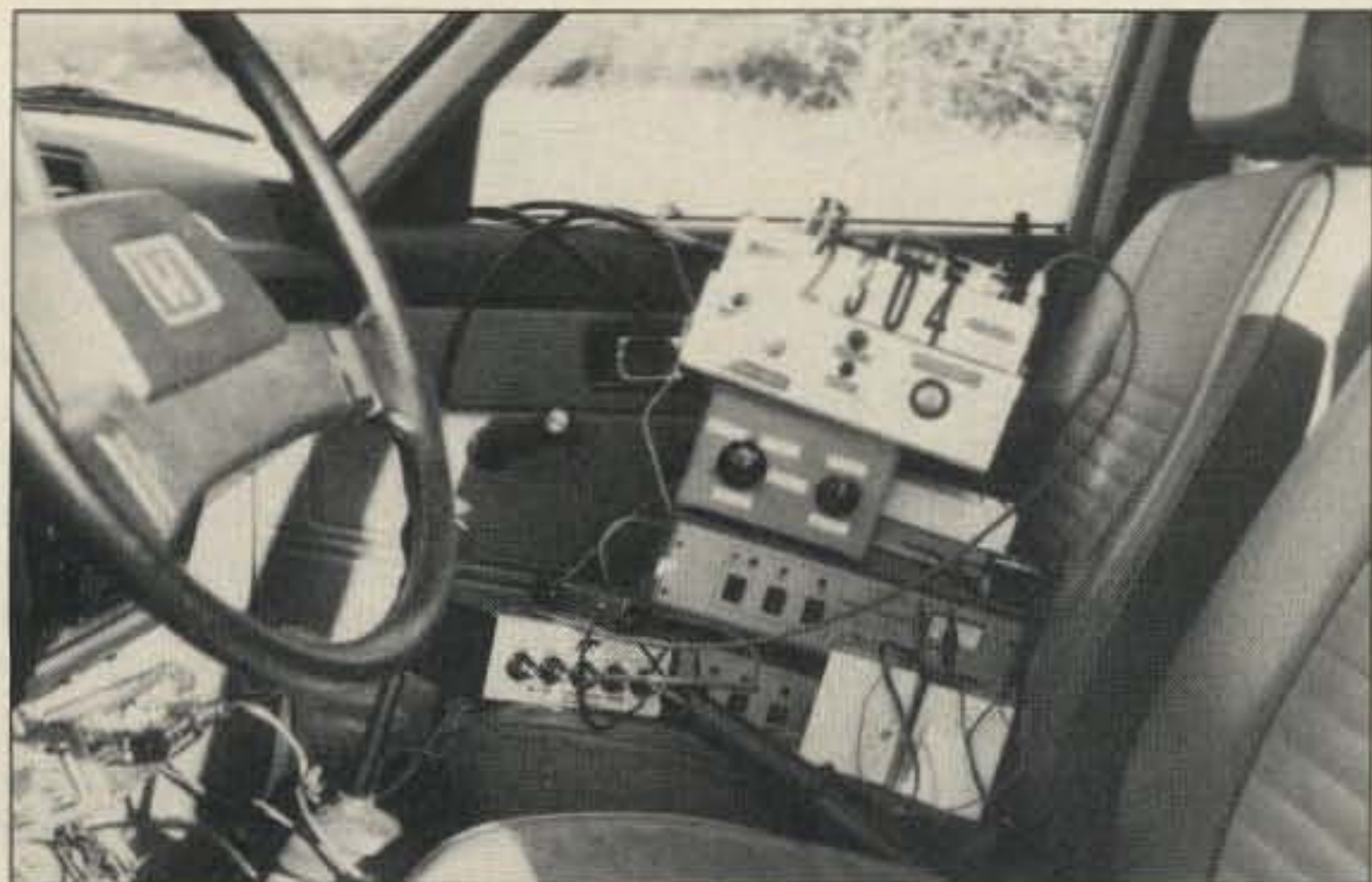
Photo A. The Honda Civic's front seat set up for 903, 1296, and 2304 MHz operation.
