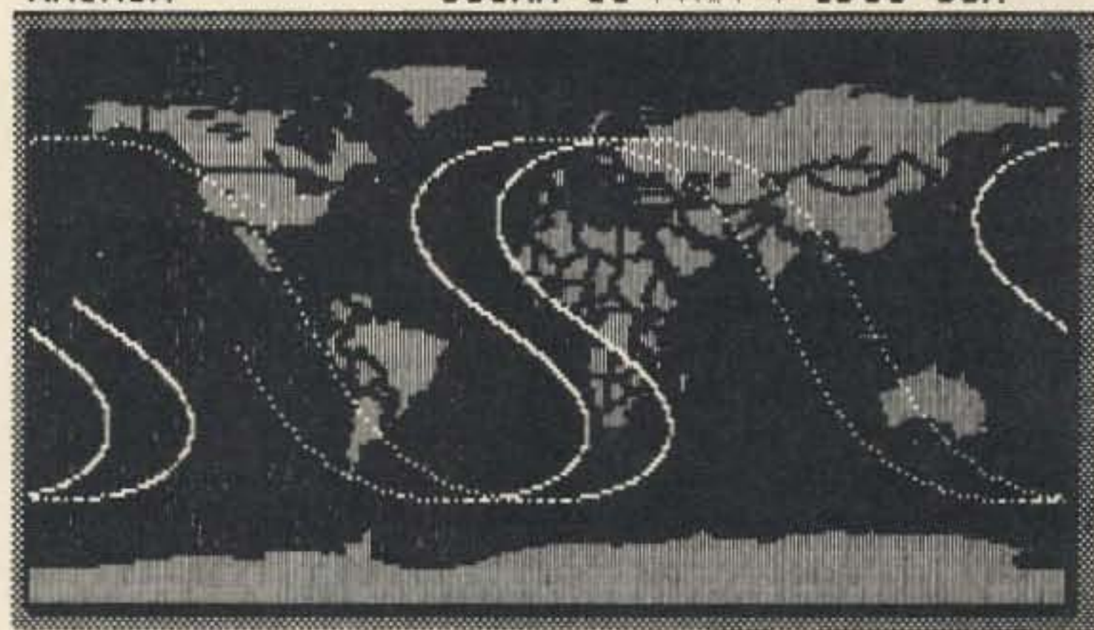
Figure 1. Final orbit after last kick motor burn. Apogee is over the equator, drifting toward the north.
