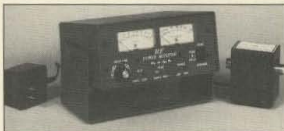
Photo A. The front panel of the RFM-003 and RF coupler.
