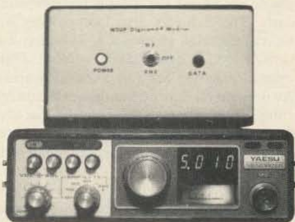
Photo E. The HF/VHF modem with a self-contained power supply. A DPDT switch was used with the center position for power off. The VHF with Equalizer mode was not used.
