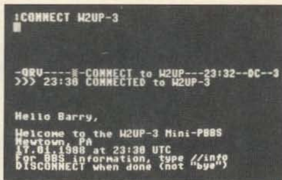
Photo B. Digicom > 64 can perform unattended BBS operation. The bulletin board can be used for file transfers or as a personal mail drop.
