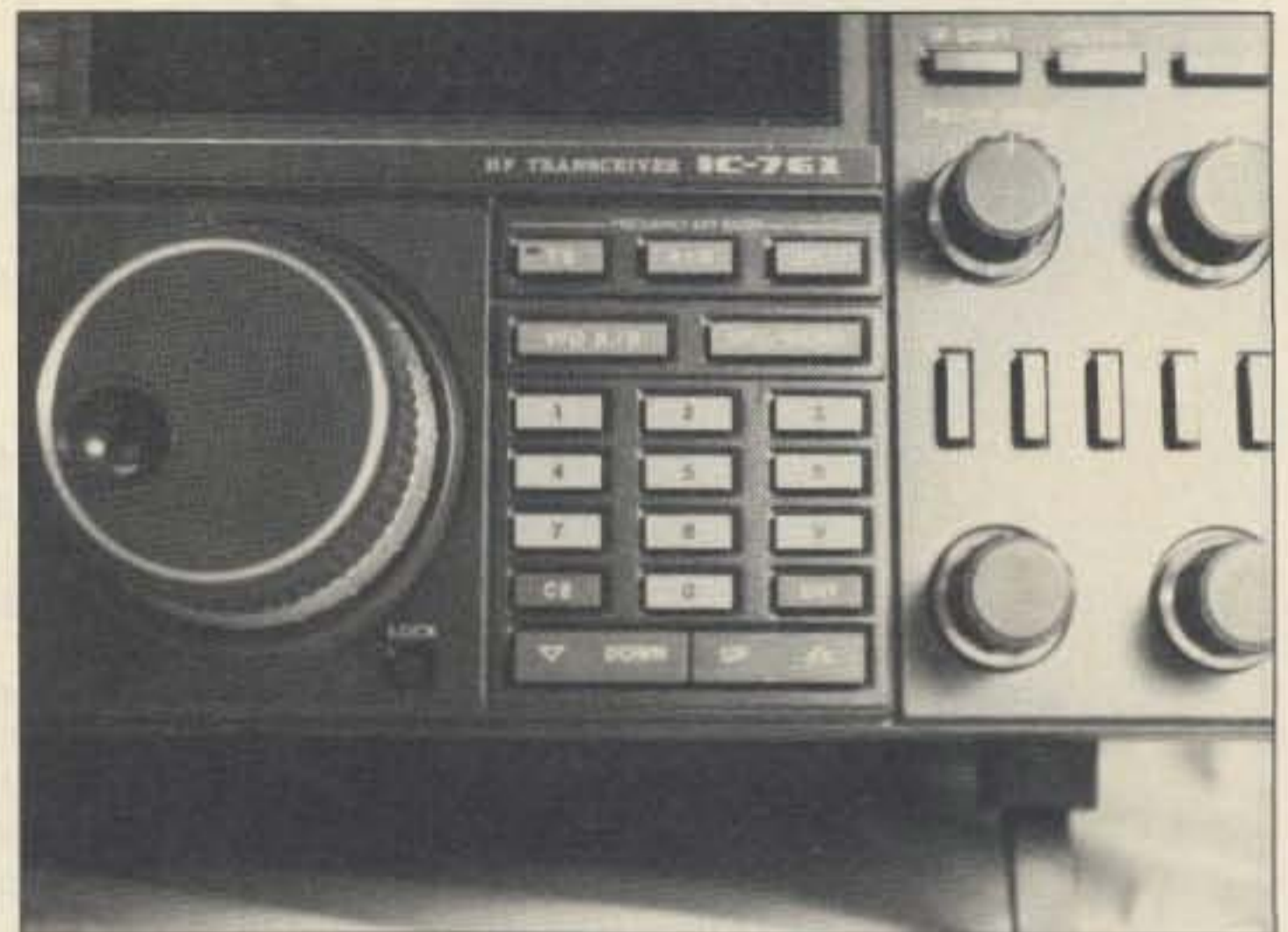
Photo B. The ICOM-761's keypad is responsible for my interest in direct keyboard frequency entry.
