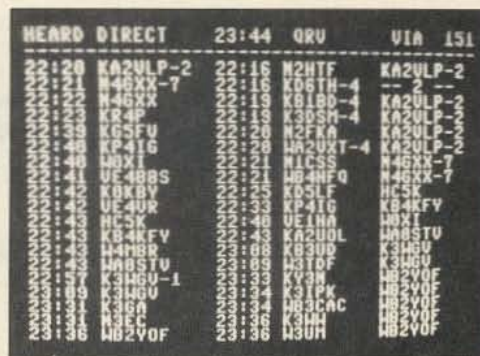
Photo C. The MHEARD screen (displayed by hitting the F7 key) shows recent packet activity. This screen is from actual operation on 20 and 2 meters. Other stations can retrieve this information to see what signals have been heard recently.
