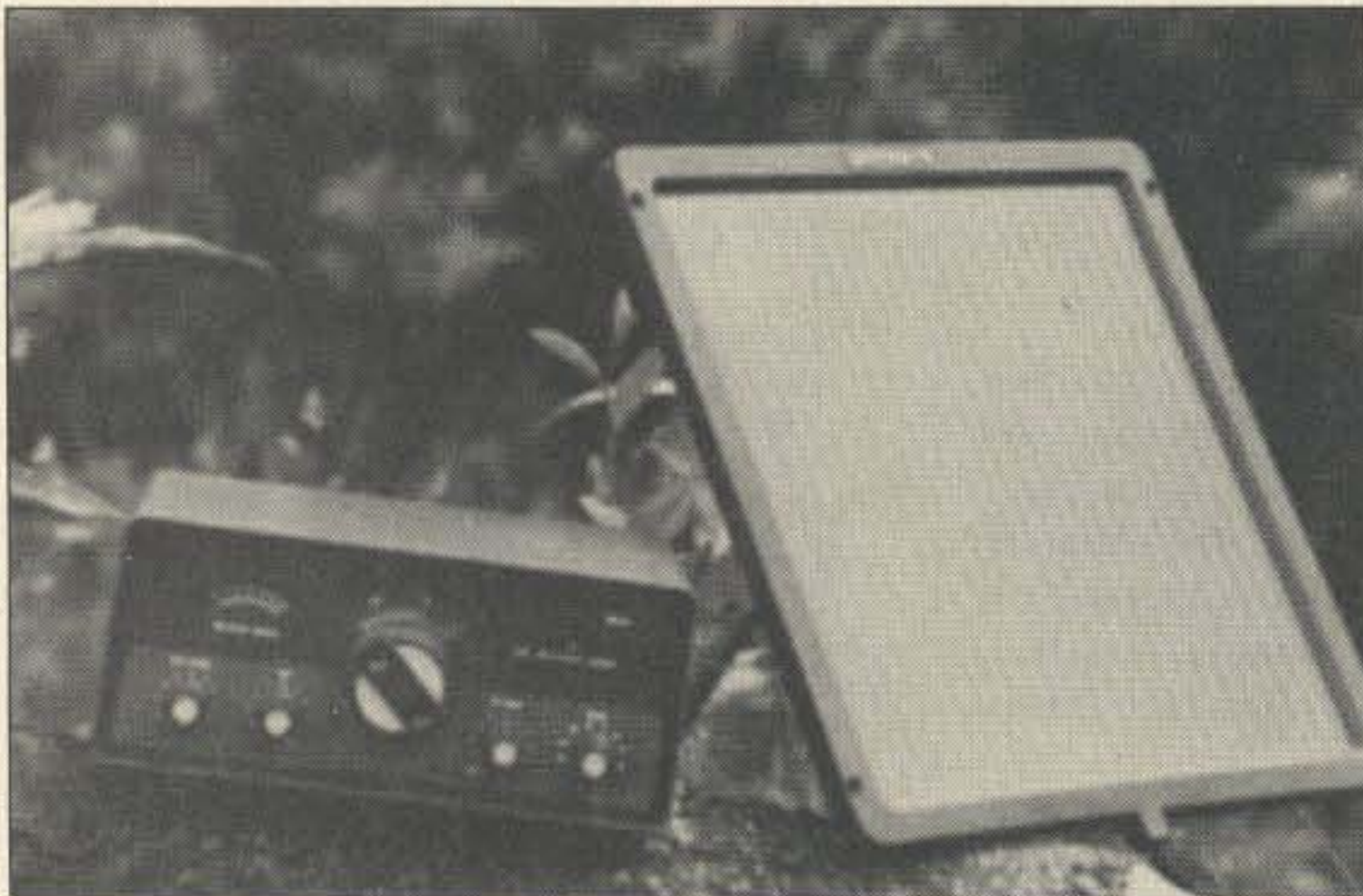
Photo A. This small five watt panel will supply all the power needed for the HW-9.
