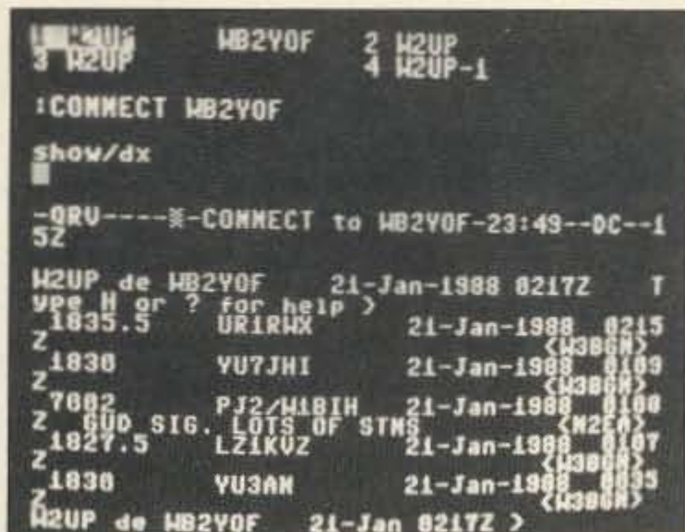
Photo A. The main screen illustrates a connection between port 1 and the Frankford Radio Club's DX spotting Packet Bulletin Board. Split screen operation allows viewing of both transmitted and received data simultaneously.
