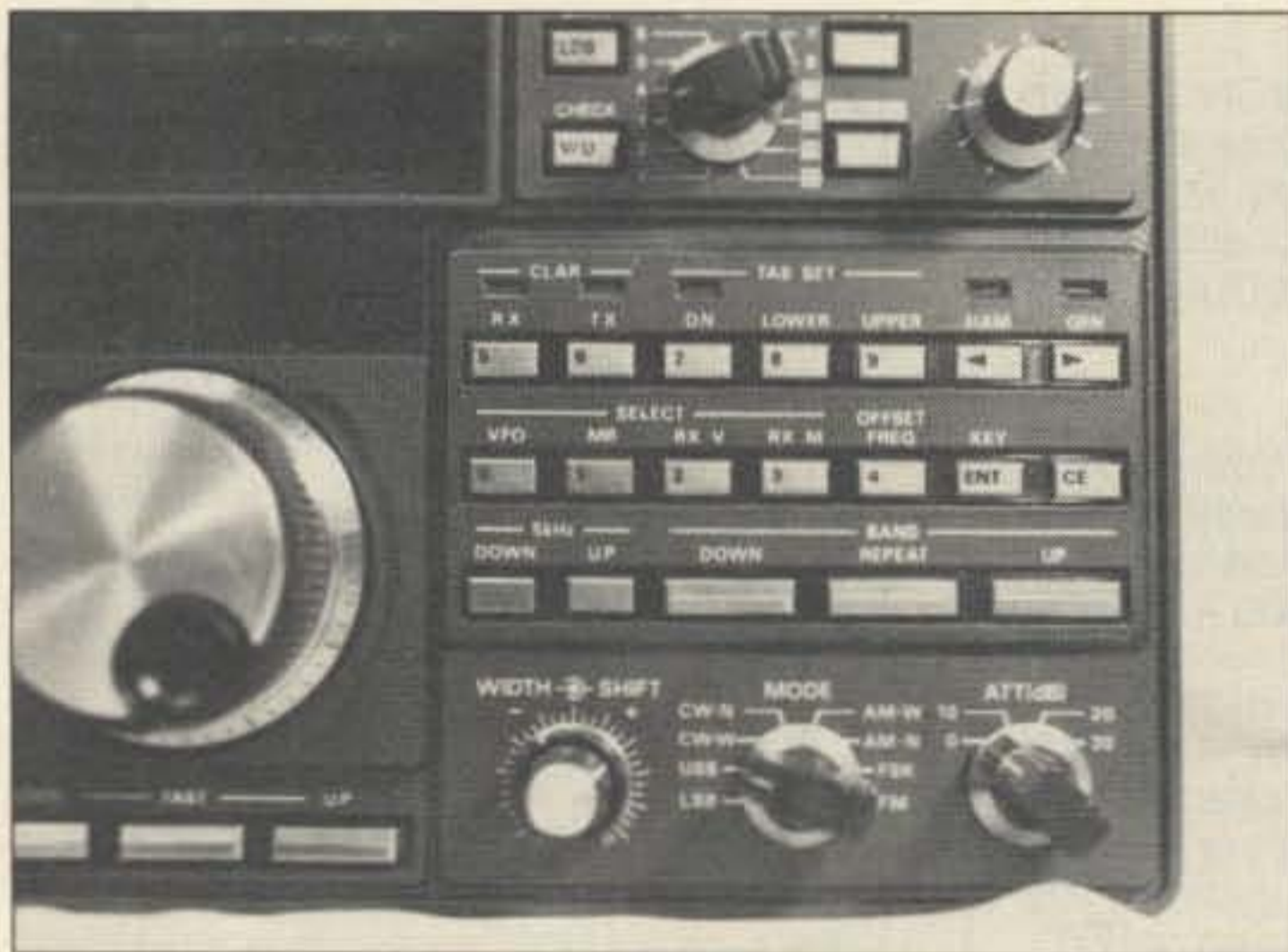
Photo A. The keyboard used for frequency entry on the Yeasu FT-980.
