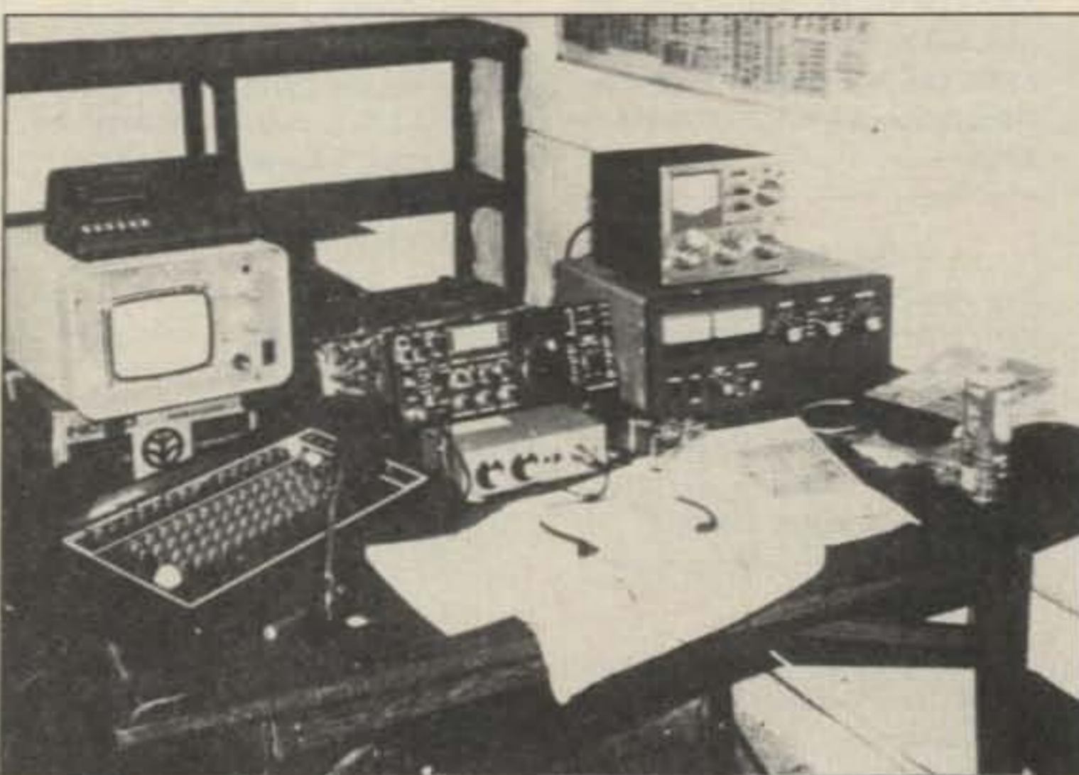
The VK9YS operating position, with ICOM 740, Yaesu FL2100, and RTTY gear.
