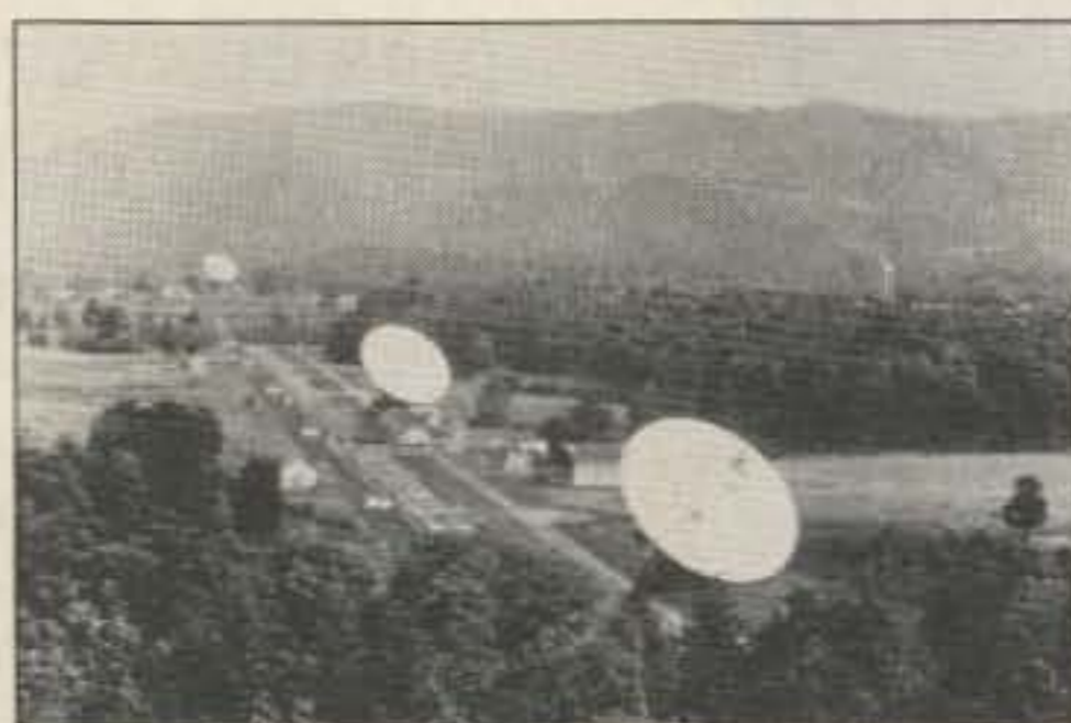
Photo C. The three-element interferometer at Green Bank. The center element has been dismantled; the two remaining are part of a four-element interferometer dedicated to astronomy.
