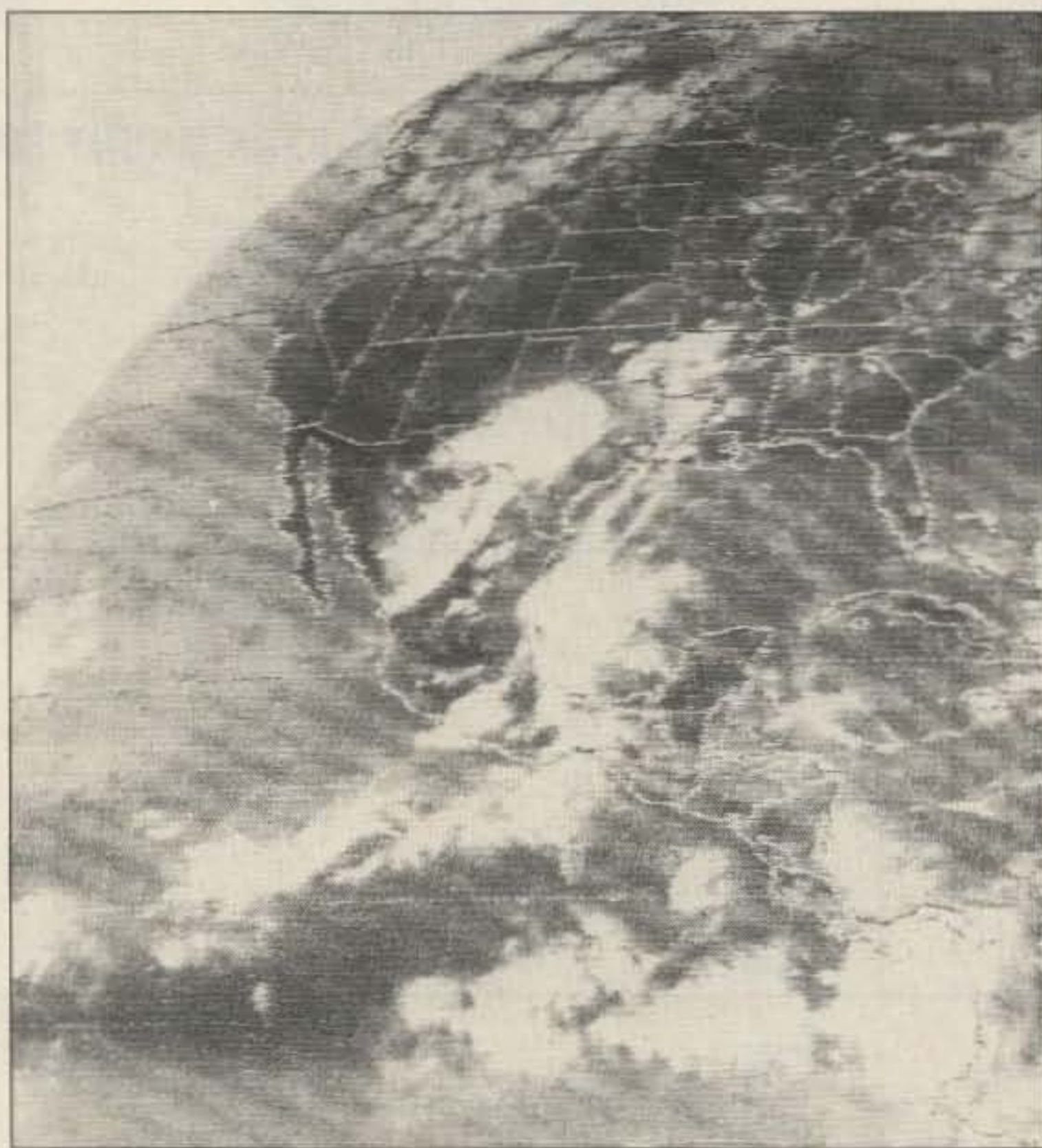
Figure 1. GOES E IR quad, transmitted through the GOES C spacecraft. The image was acquired live using the WSH scan converter and a 512K CoCo 3. This particular print was made directly from the high-resolution image in the computer memory (380K of image data) and printed to the simplified SMARTFAX recorder to be described next month.
