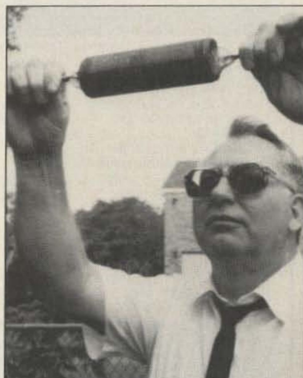
Photo. Joe Plesich holding a finished loading coil.
