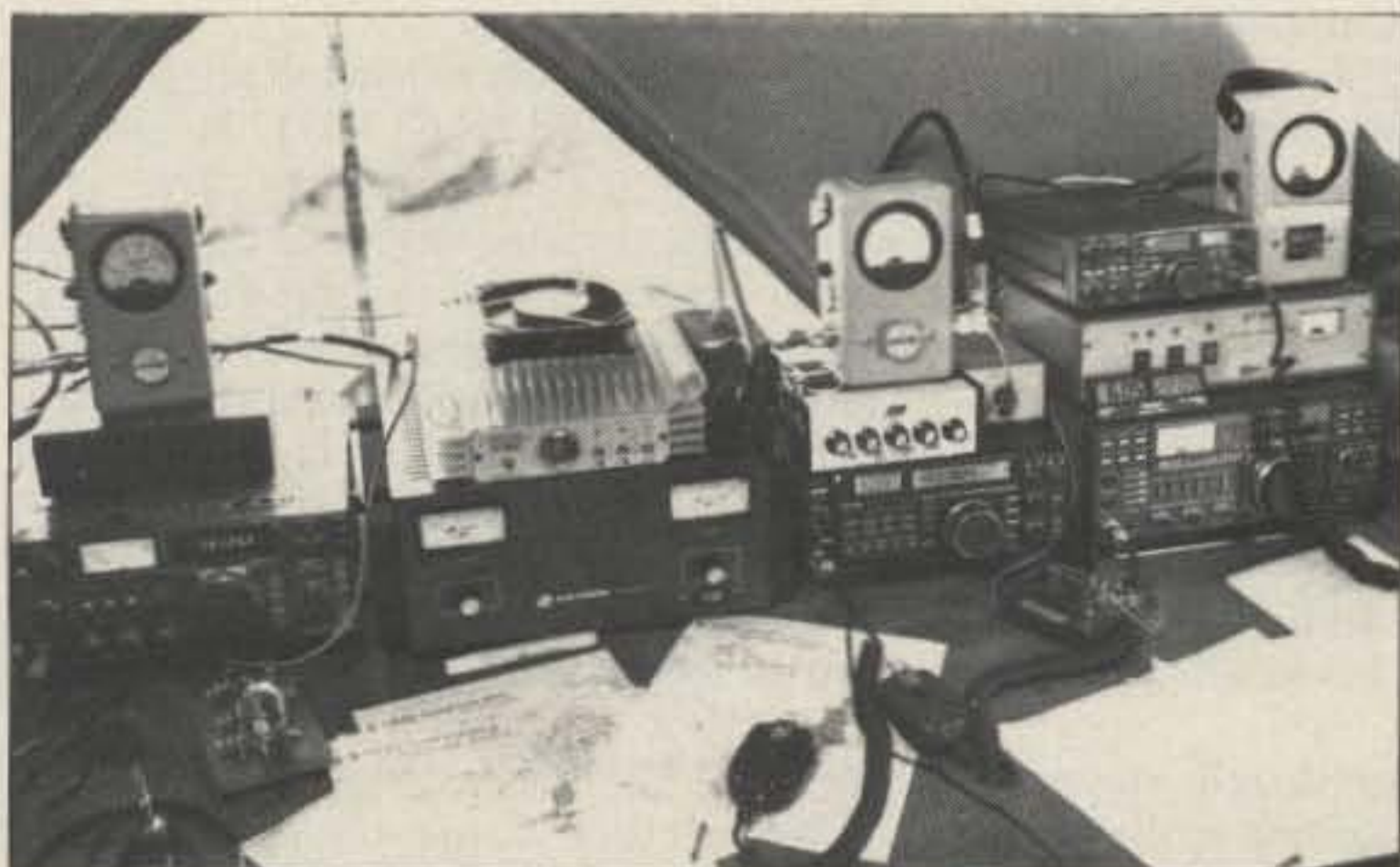
Photo A. The UHF station at WB2WIK/4. From left to right are the 220-, 432-, 902-, and 1296-MHz stations.
