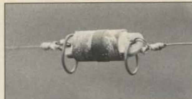
Photo C. Trap installed in antenna.
