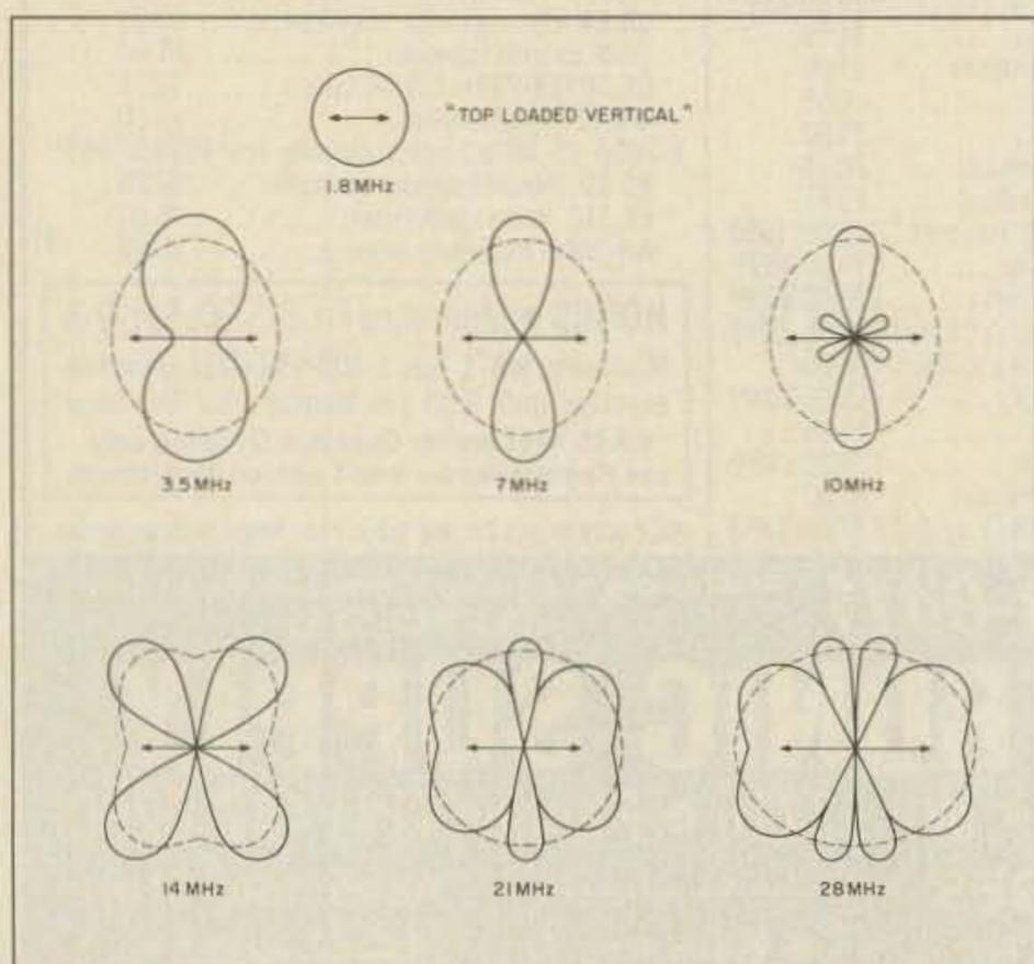
Fig. 1. Approximate directional patterns for antenna number one (66 feet each side of the center). The dotted lines show the patterns when the antenna is in the form of an inverted vee.
