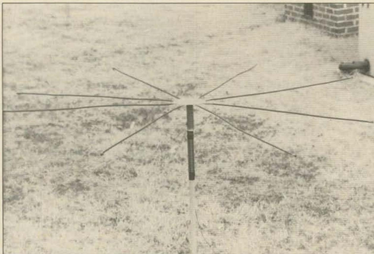
Photo A. Bird's-eye view of the quarter-scale top hat and loading coil.
