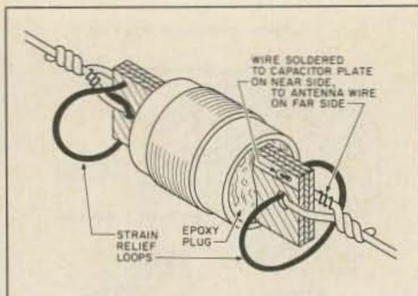
Fig. 6. Connecting the trap to an antenna.
