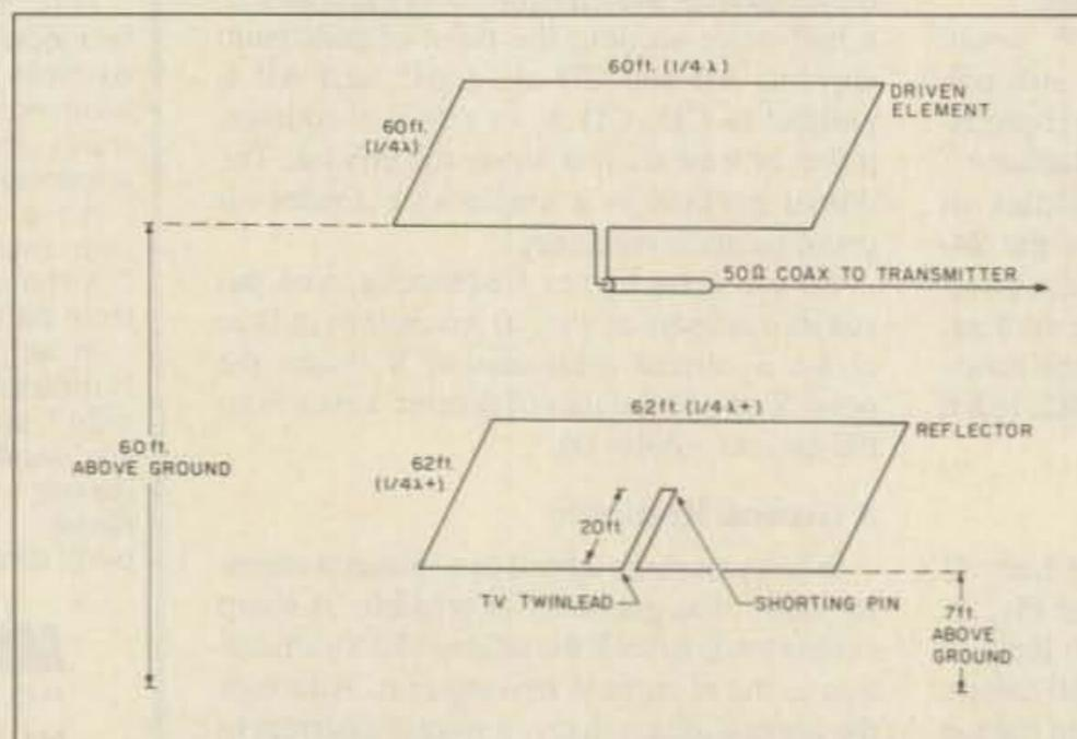
Fig. 1. The 75-meter laid-back quad.
