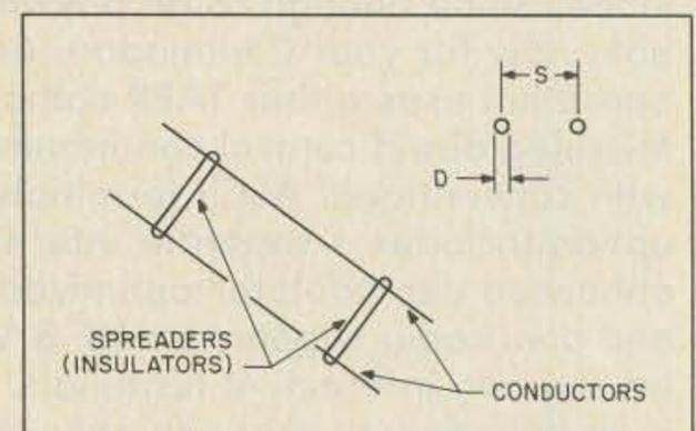
Fig. 3. A parallel feeder.
