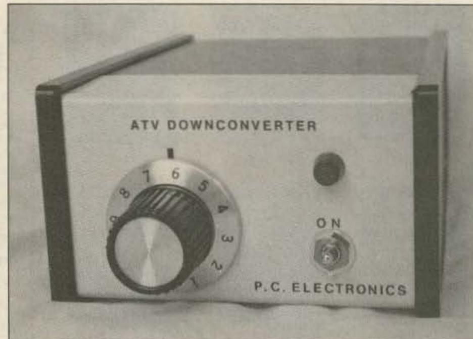
900-MHz ATV downconverter available from P.C. Electronics.
