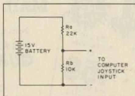
Fig. 2. Voltage divider for reducing battery voltage to a value within the range of the A/D.
