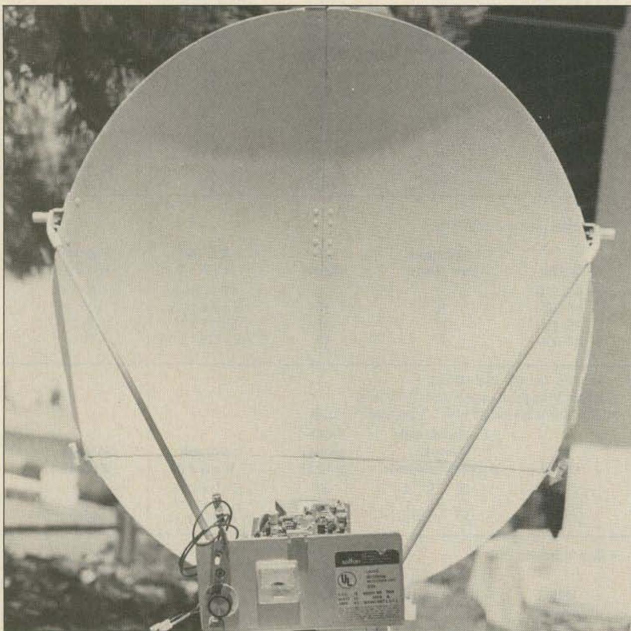
Photo A. Off-center-feed 10-GHz dish with original transceiver mounted at focus. Used for Mount Soledad to Mount Helix contacts.
