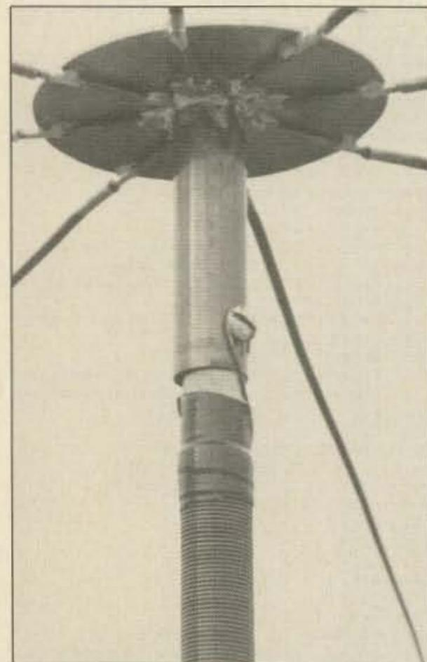
Photo B. Construction details of the quarter-scale top hat.
