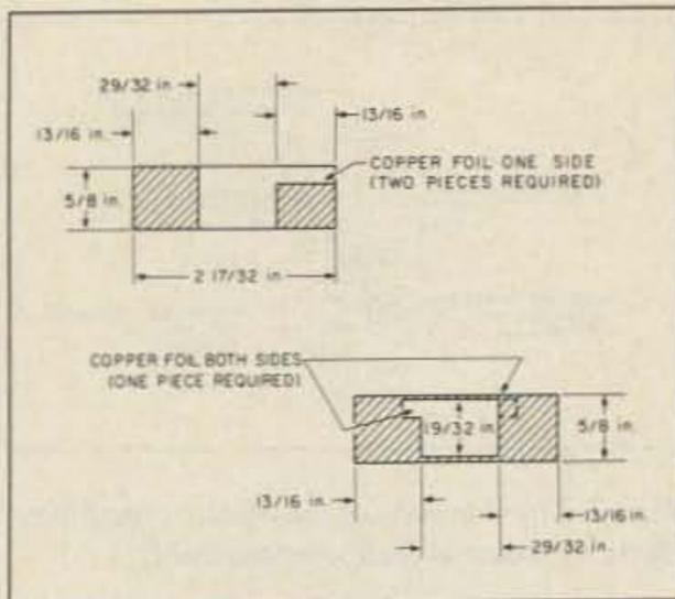
Fig. 2. Plates for 50-pF capacitor assembly.
