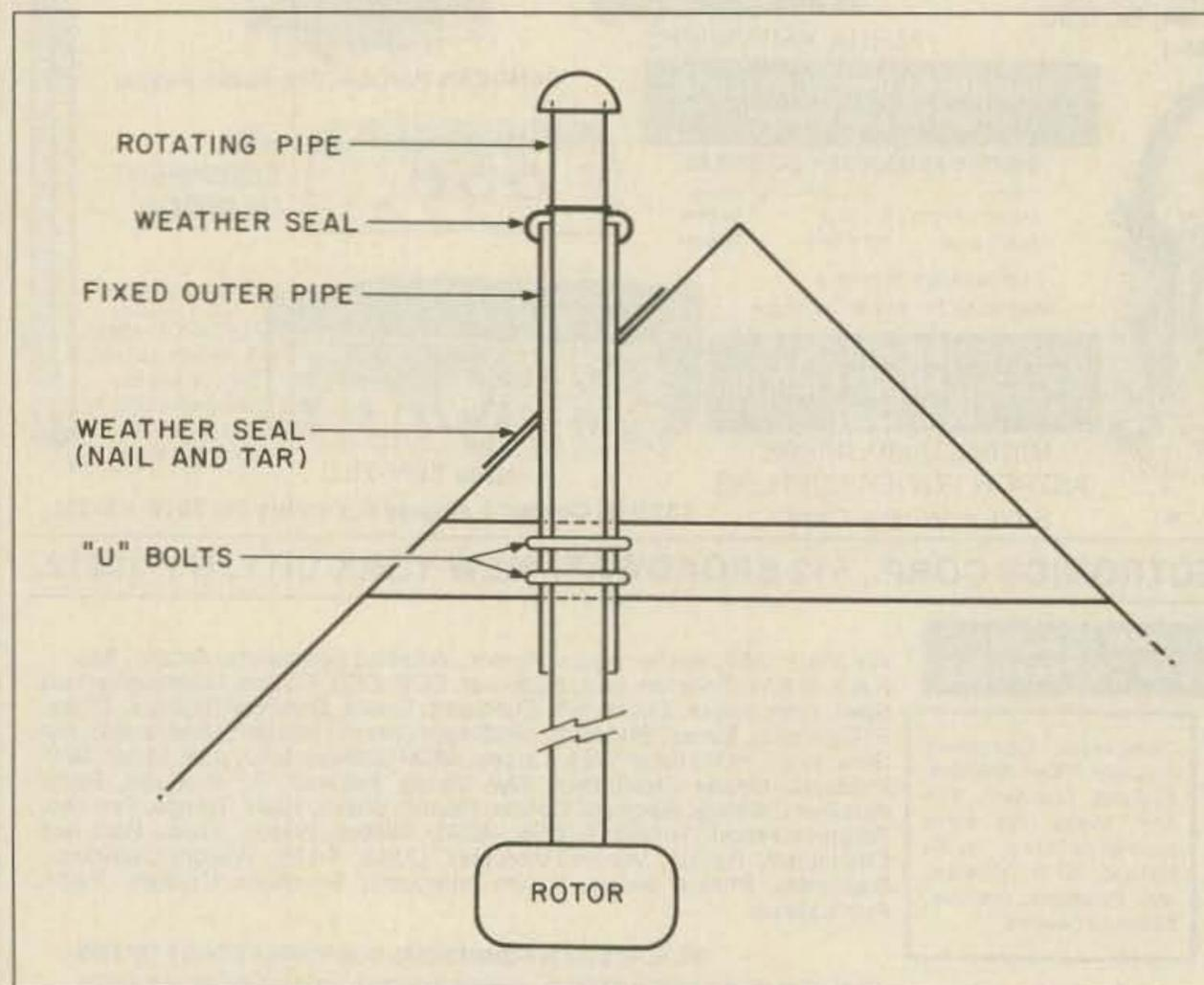
Fig. 1. WA2OLZ's through-the-roof mounting system protects your rotator from the elements and circumvents restrictive tower ordinances.
