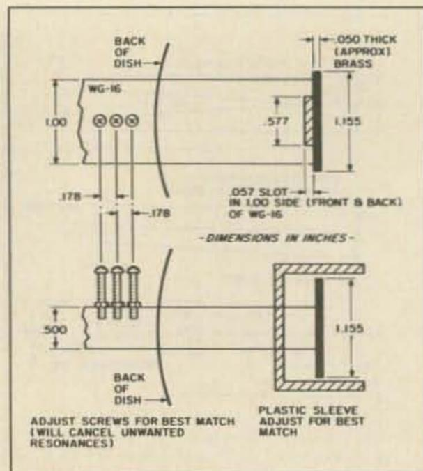
Fig. 2. A slot-feed method for 10 GHz.
