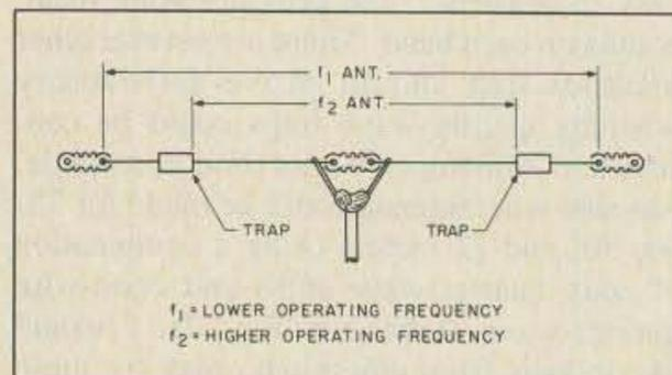
Fig. 1. Trap-tuned dipole antenna.
