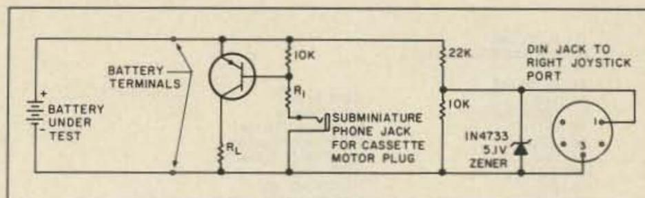
Fig. 4. Modified circuit for higher discharge current.
