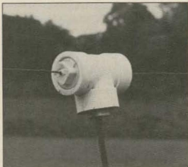
Photo E. Feedline protection using plastic pipe fitting.
