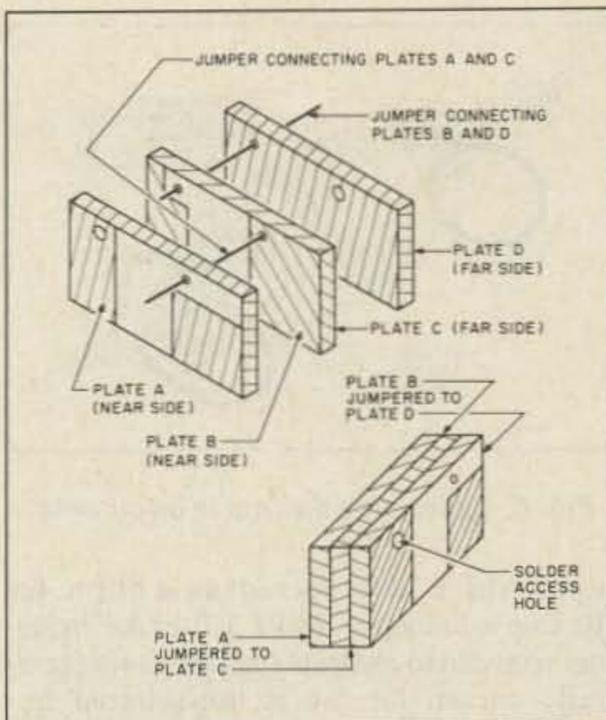
Fig. 3. Capacitor assembly detail.
