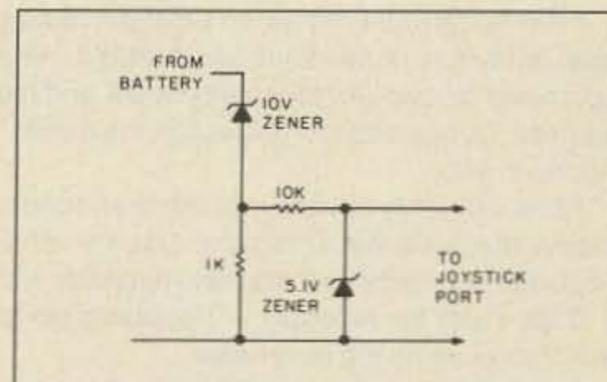
Fig. 7. Scale Expander Circuit.
