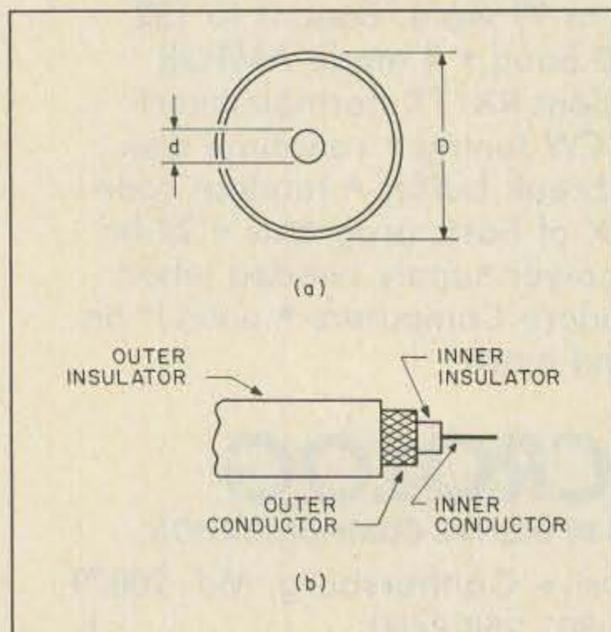
Fig. 1. Coaxial cable.
