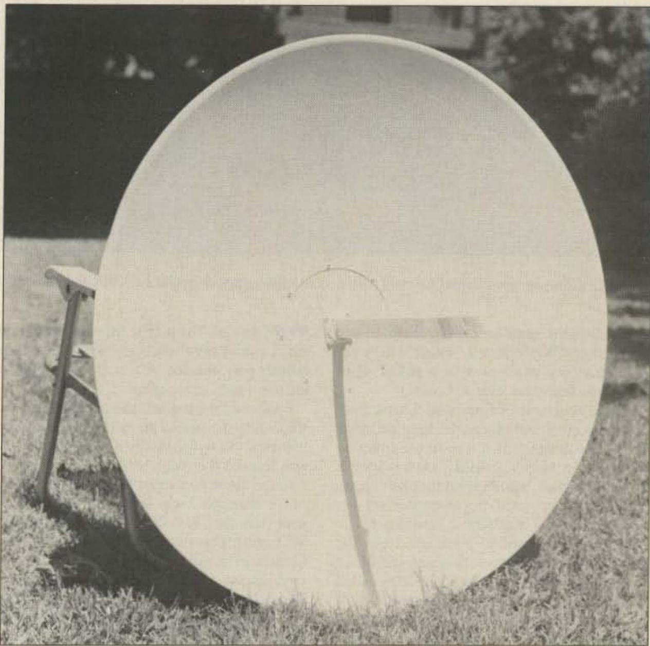
Photo B. 10-GHz dish antenna with dipole feed and dielectric resonator (plastic bag) in place.
