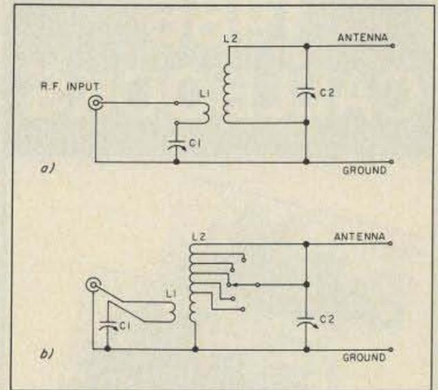
Fig. 5. Circuits of simple tuners suitable for feeding rf voltage to one end of a resonant-length antenna wire. The tuner in a) utilizes plug-in coils, while the circuit shown in b) uses a more convenient tapped coil. (These tuners will not work with a random-length antenna wire.)
