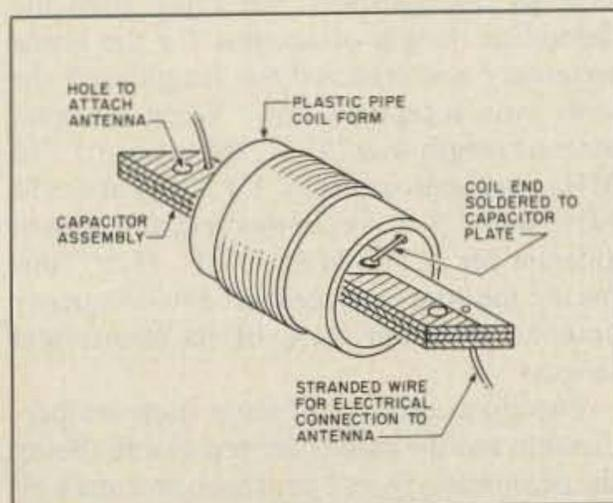
Fig. 4. Trap assembly.
