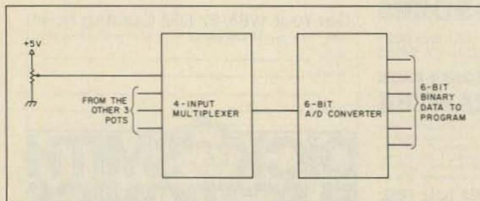
Fig. 1. Joystick connections in the CoCo.
