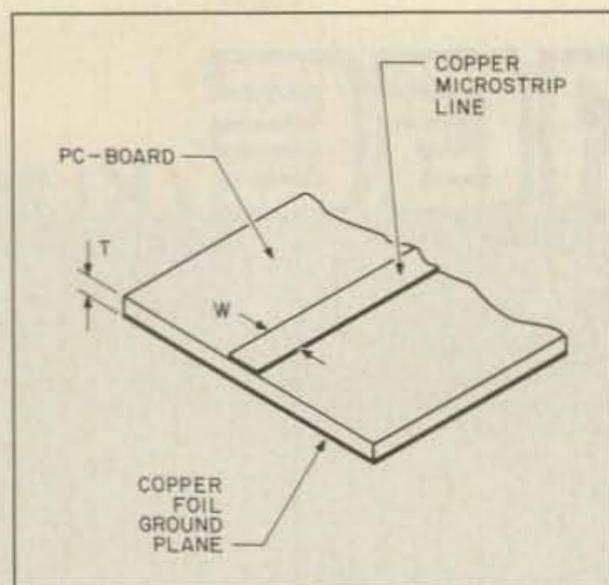
Fig. 4. A common microstrip configuration.
