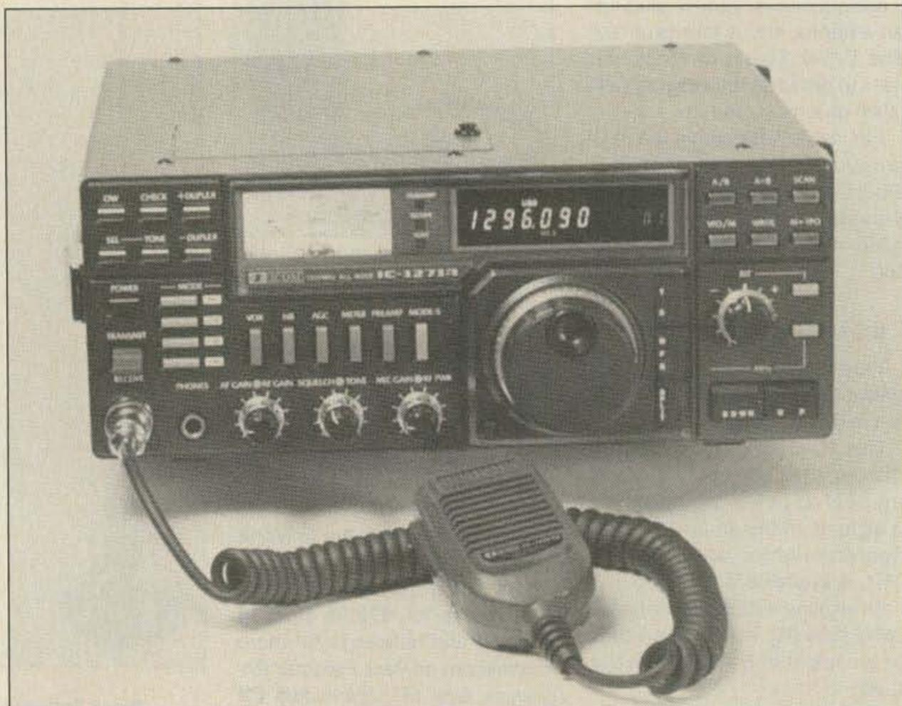
Photo A. The ICOM IC-1271A 23-cm multimode transceiver.
