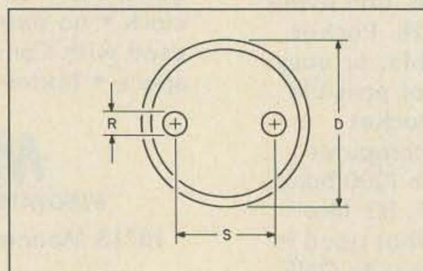
Fig. 2. Shielded parallel line.
