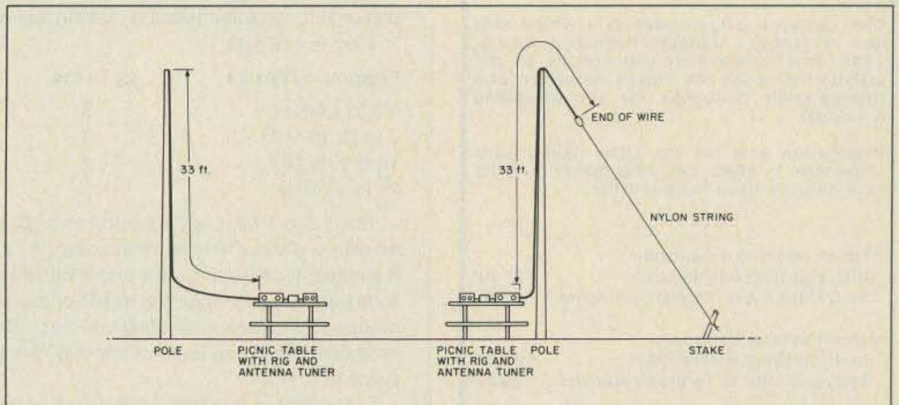
Fig. 6. Twenty-meter vertical resonant-wire antennas.
