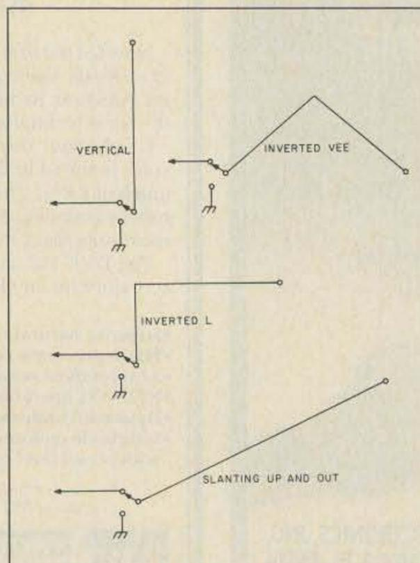
Fig. 3. *Some endfed-antenna configurations.*
