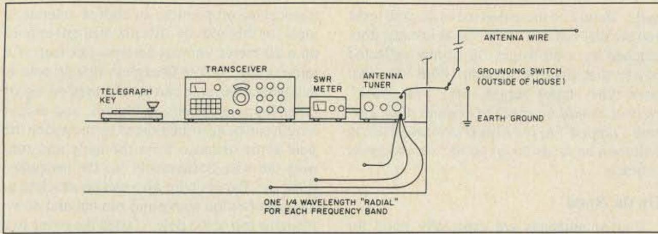
Fig. 4. Protect your station against lightning damage with a grounding switch mounted outside of the house.
