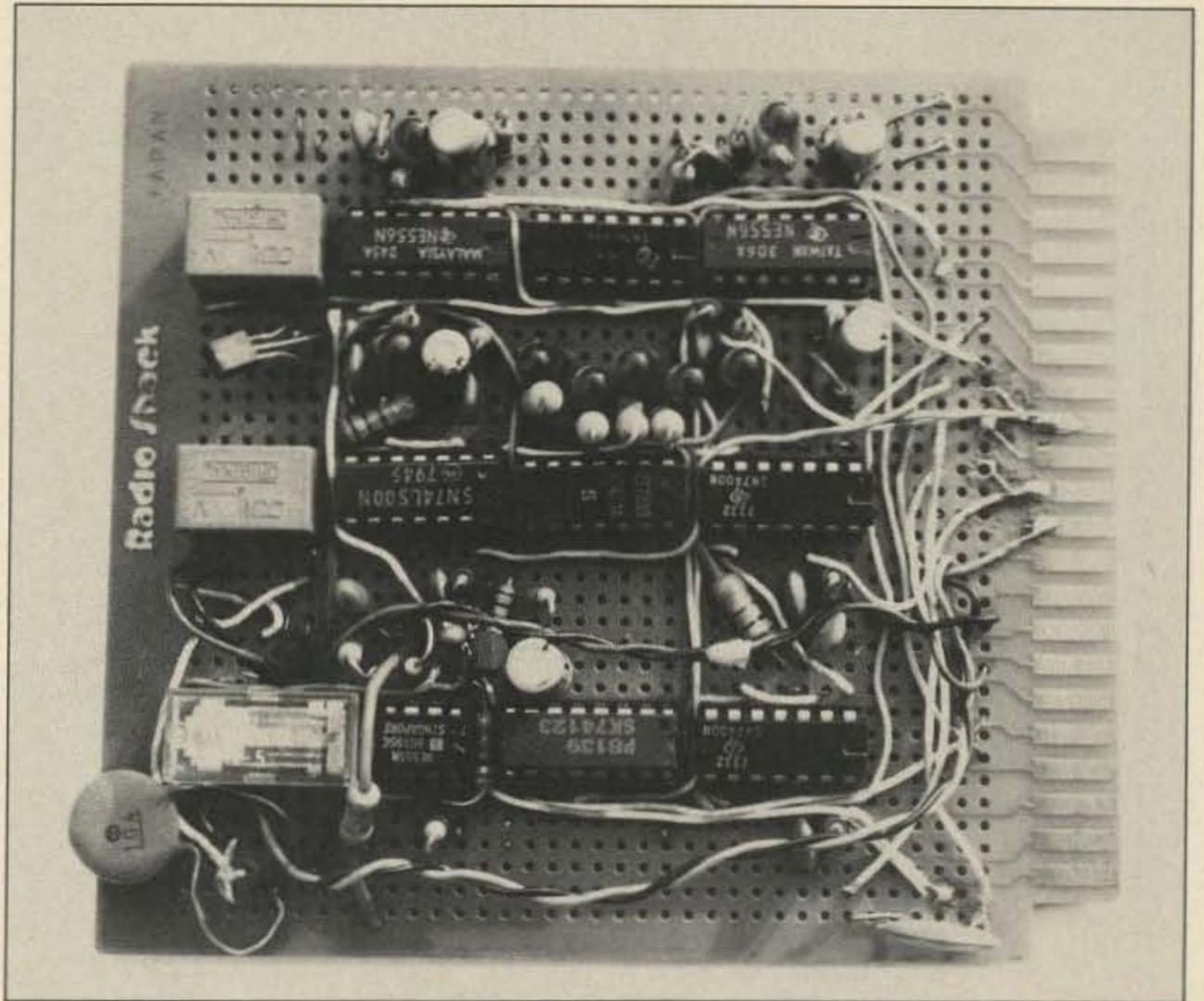
Photo A. A complete simplex link on one tiny board.
