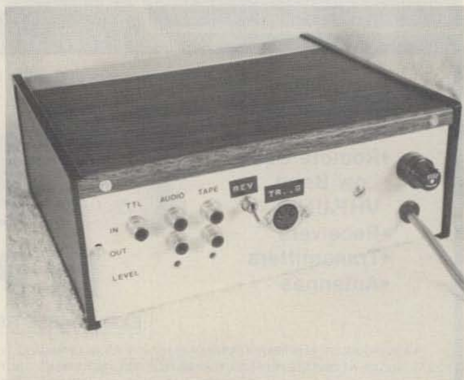
Photo B. The rear panel with the multitude of connectors for the various inputs and outputs. The 5-pin DIN connector is used for the hookup to the serial port. The label indicates the 3 pins used: transmit data, receive data, and ground. The switch is for reversing the "sense" of the RTTY signal via the exclusive OR gates on the serial board. The audio-level trim pots are visible below the audio and tape outputs. The "audio" input and output are used for the connections to the rig.
