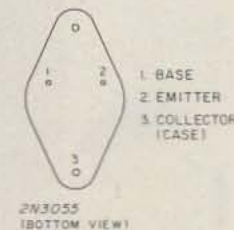
Fig. 3. Base diagrams. Note that the pin connections for the two voltage regulators are different.
