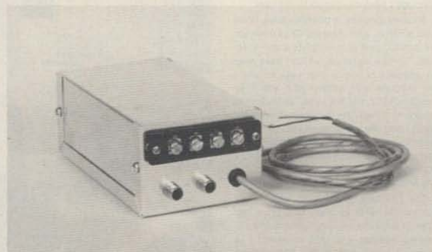
Photo A. The ARR sequencer. The two RCA jacks bring in the PTT line and key the bias for the amplifier. Additional closures are available through the terminal strip.
