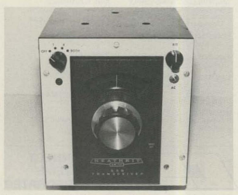
Photo A. A duplication of the HW-101's internal vfo is installed in a recycled Heath VF-1 cabinet. The original vfo in this 25-year-old box could drift through most of a band in one evening. Perfect for gradual QSY in a contest.
