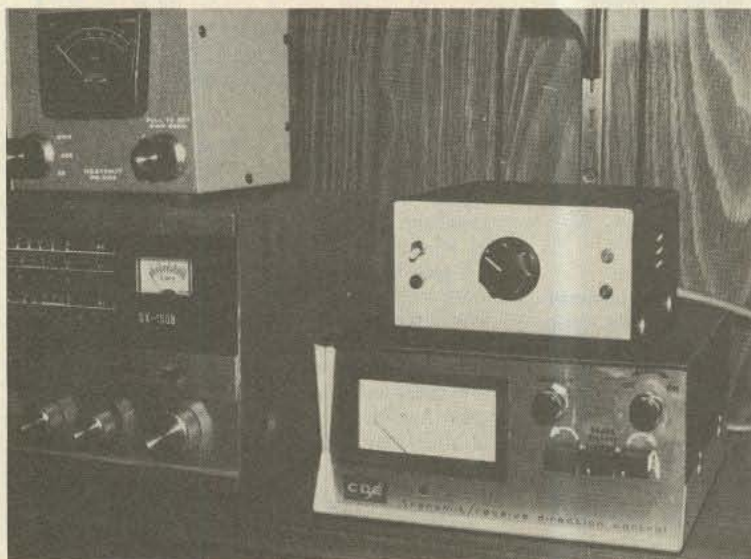
Photo A. The completed beam aimer sits atop the rotator control box at the W4RNL operating position. The ac switch and power LED are to the left and the clockwise and counterclockwise LEDs are to the right. The center knob is the direction control prior to the addition of calibration markings.
