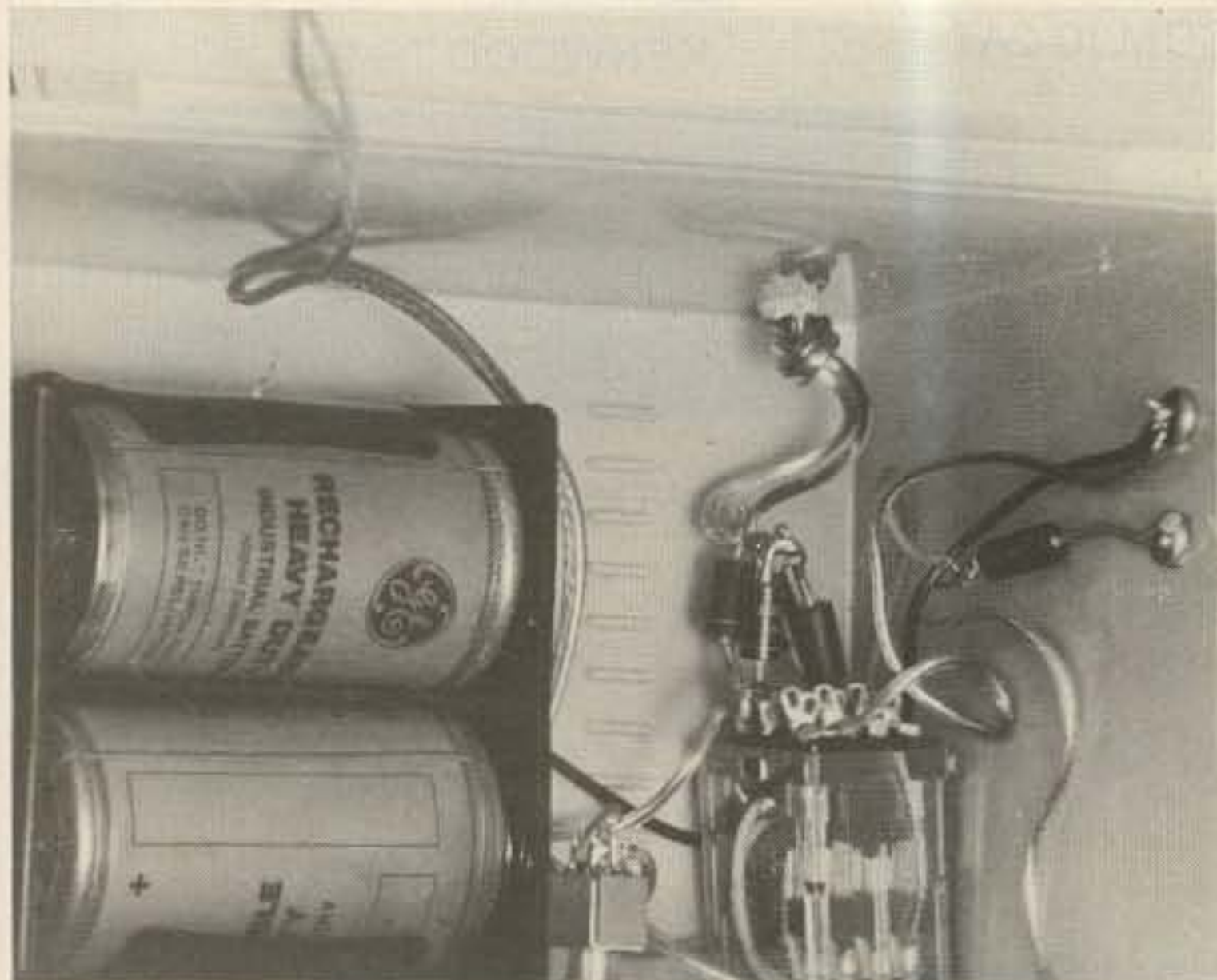
Parts placement. The four diodes at the relay form a bridge, allowing use of a 6-volt relay and a cheap ac low-voltage game module. The diode near the top of the box ensures proper polarity of the recharging current.
