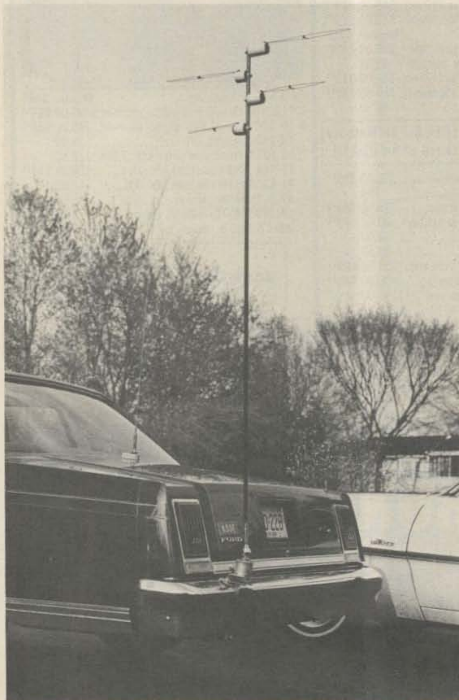
Fig. 2. Resonator positioned at 90^\circ (vertical polarization retained).
