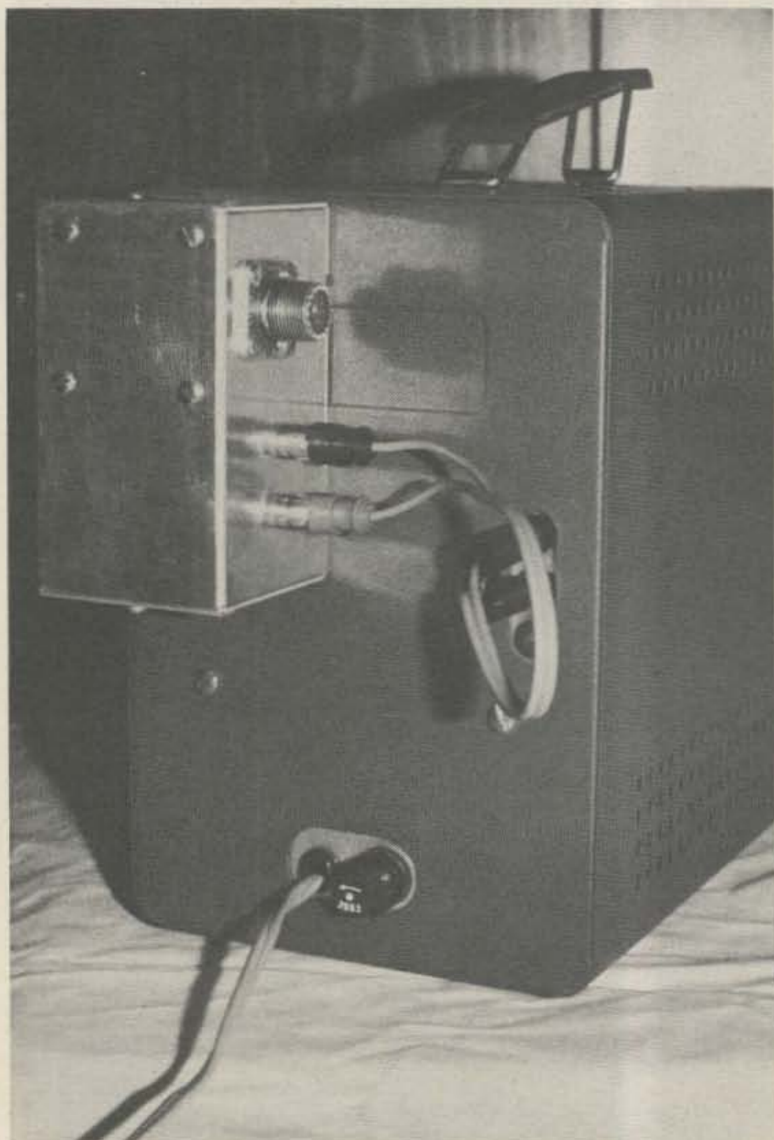
An external view of the adaptor shown in Fig. 8, with shielded connections to the rear of the scope and onward to the vertical deflection plates.
