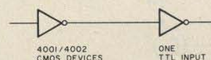
Fig. 2(b). 4001/4002 CMOS will drive one regular TTL load.
