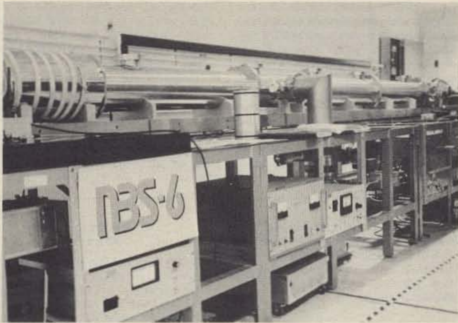
Photo A. NBS-6, the cesium-beam atomic clock at the National Bureau of Standards in Boulder, Colorado. This clock is the most accurate timepiece in the world!
