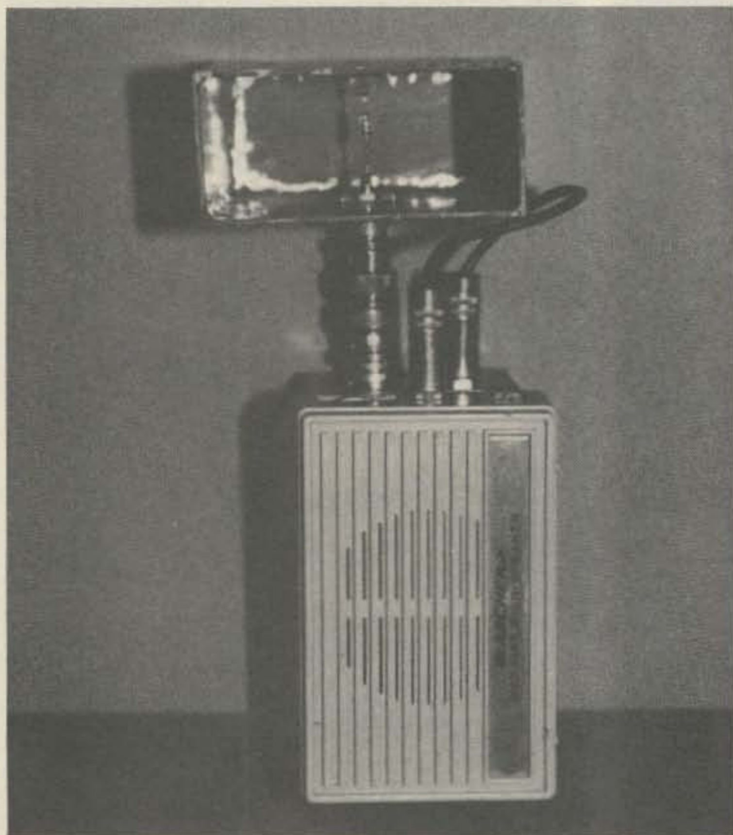
Front view of S-band unit showing diode placement.
