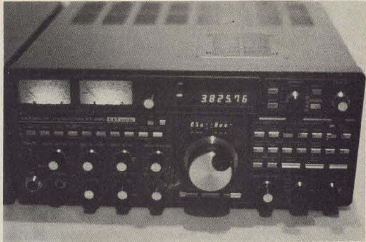
Operating side of the FT-980. The curious pseudo-analog display is right above the main tuning control (more on this in the text and Fig. 2).
