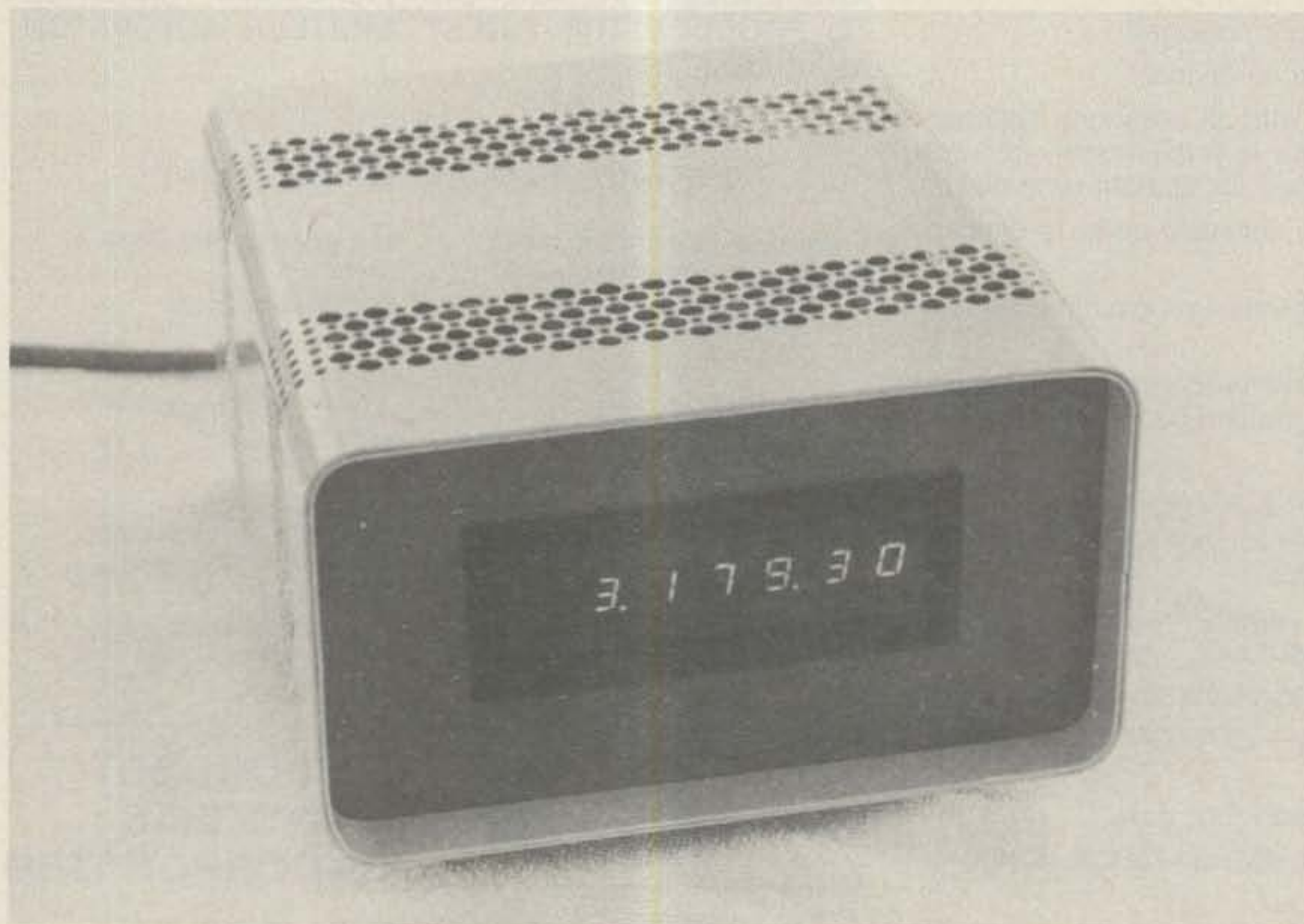
Photo A. Front view. Note that many ventilation holes were drilled oversize for more effective convection cooling of the internally-mounted LM323K voltage regulator and heat sink (photo by R. Campbell).
