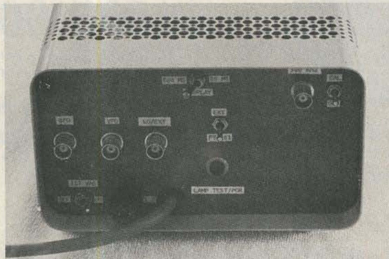
Photo B. Rear view. Shown are the FT-101 inputs, the 500-kHz CAL output, and the operating controls. For frequency counter use, the toggle switch is set to EXT and the signal of interest connected to the LO/EXT input (photo by R. Campbell).
