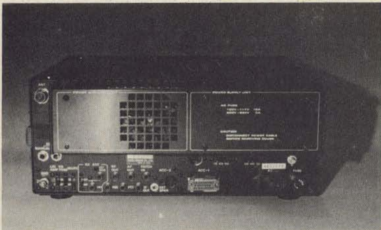
Rear panel of the FT-980 has almost as many switches as the front panel. The projecting module holds the power amplifier (left) and the power supply (right).
