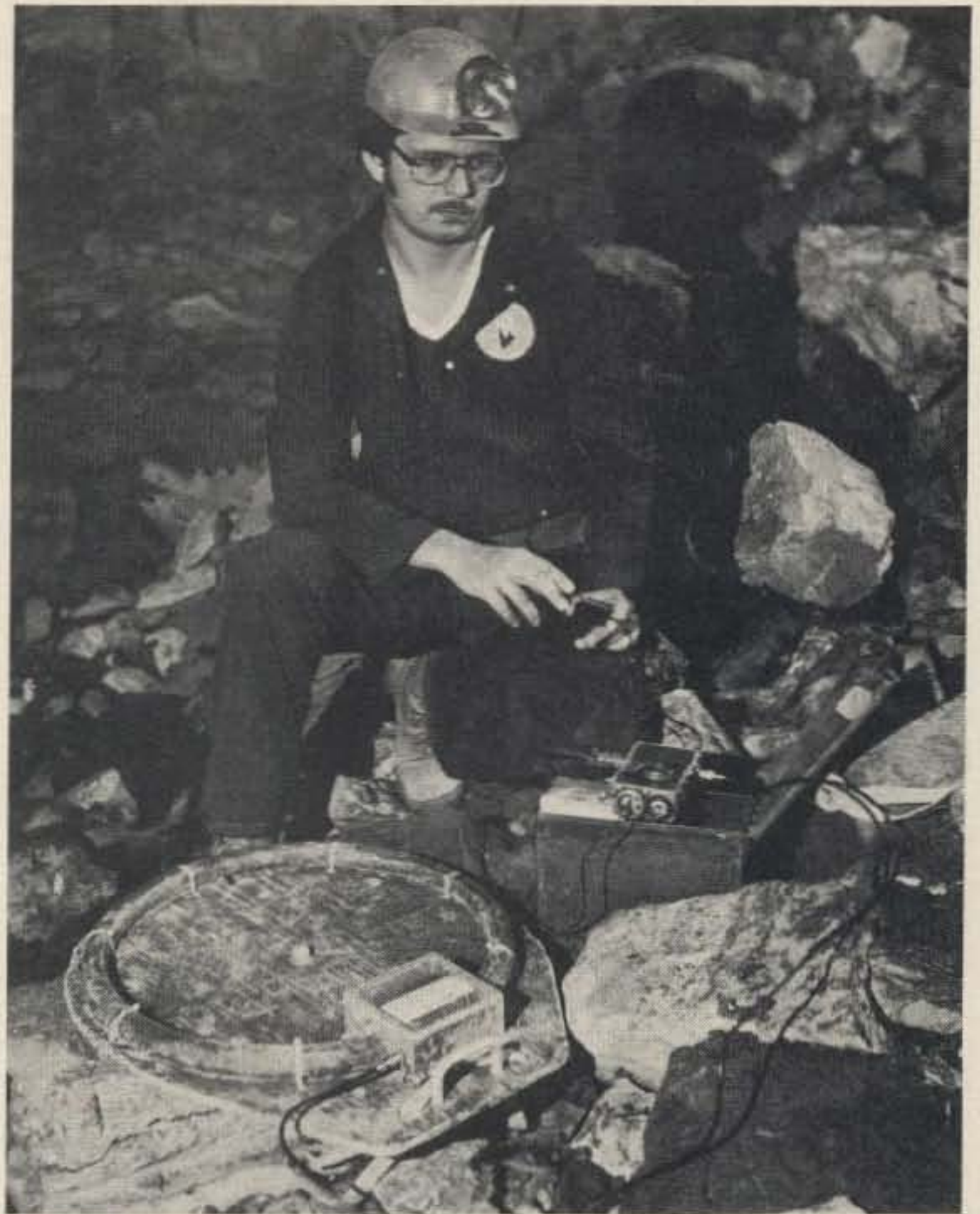
WB9TLH operates underground transmitter on 3500-Hz CW, using microswitch for telegraph key.
