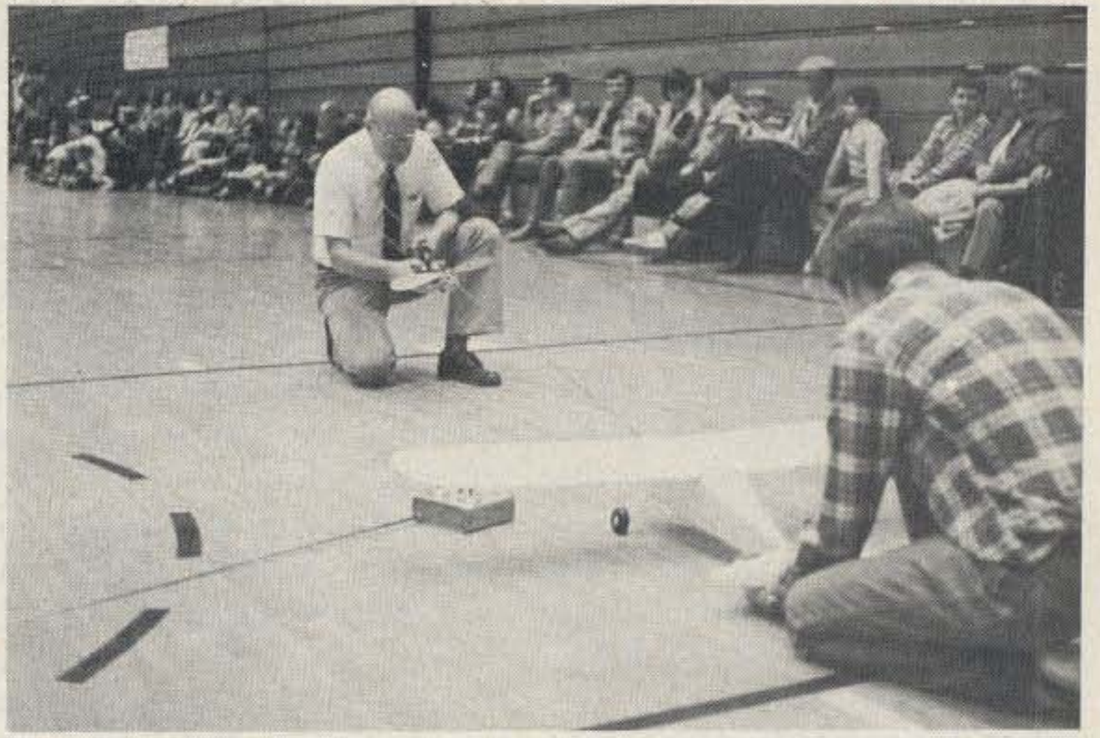
A one-inch-per-foot scale model of a Porterfield Collegiate is powered up. A small hand drill and hook are used to wind up the large rubber band to full power.
