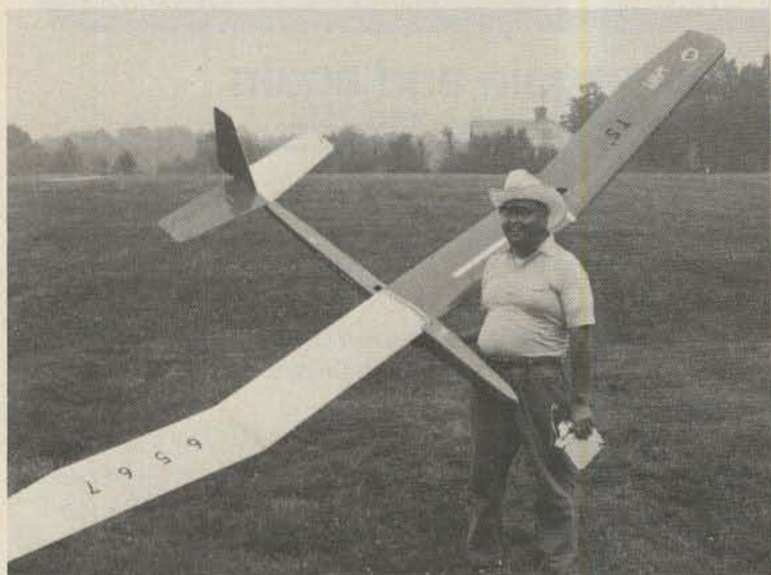
The PennFli, an unlimited class sailplane of fourteen-foot wingspan, weighs about five pounds. Made of balsa and plywood, the plane is covered with a plastic film which shrinks and sticks to the wood when heated with a common clothes iron. Controls are rudder, elevator, spoiler (airbrakes), and releasable tow hook.
