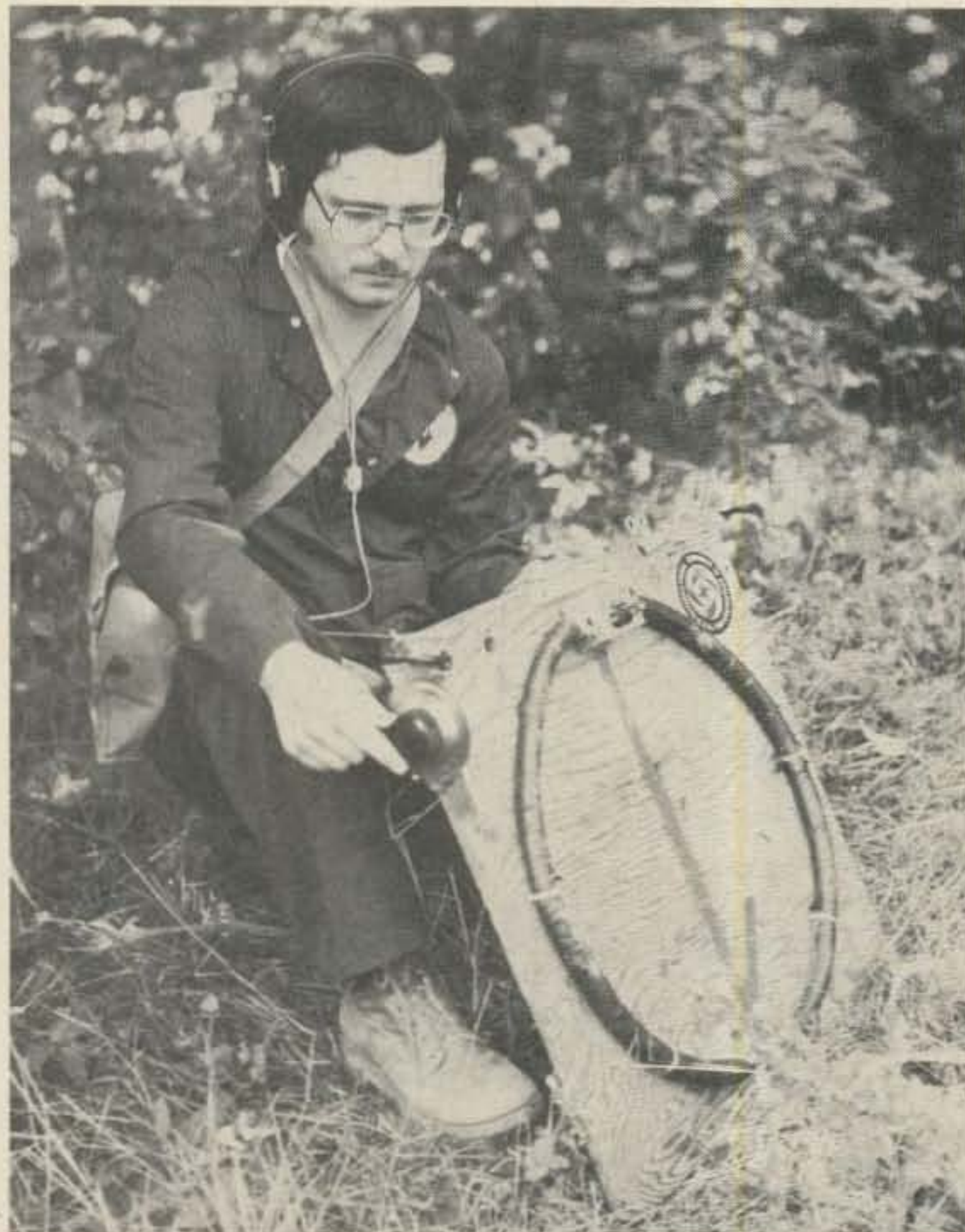
Surface location and depth of transmitter are found by null-seeking with directional antenna and by measuring shape of magnetic field.
