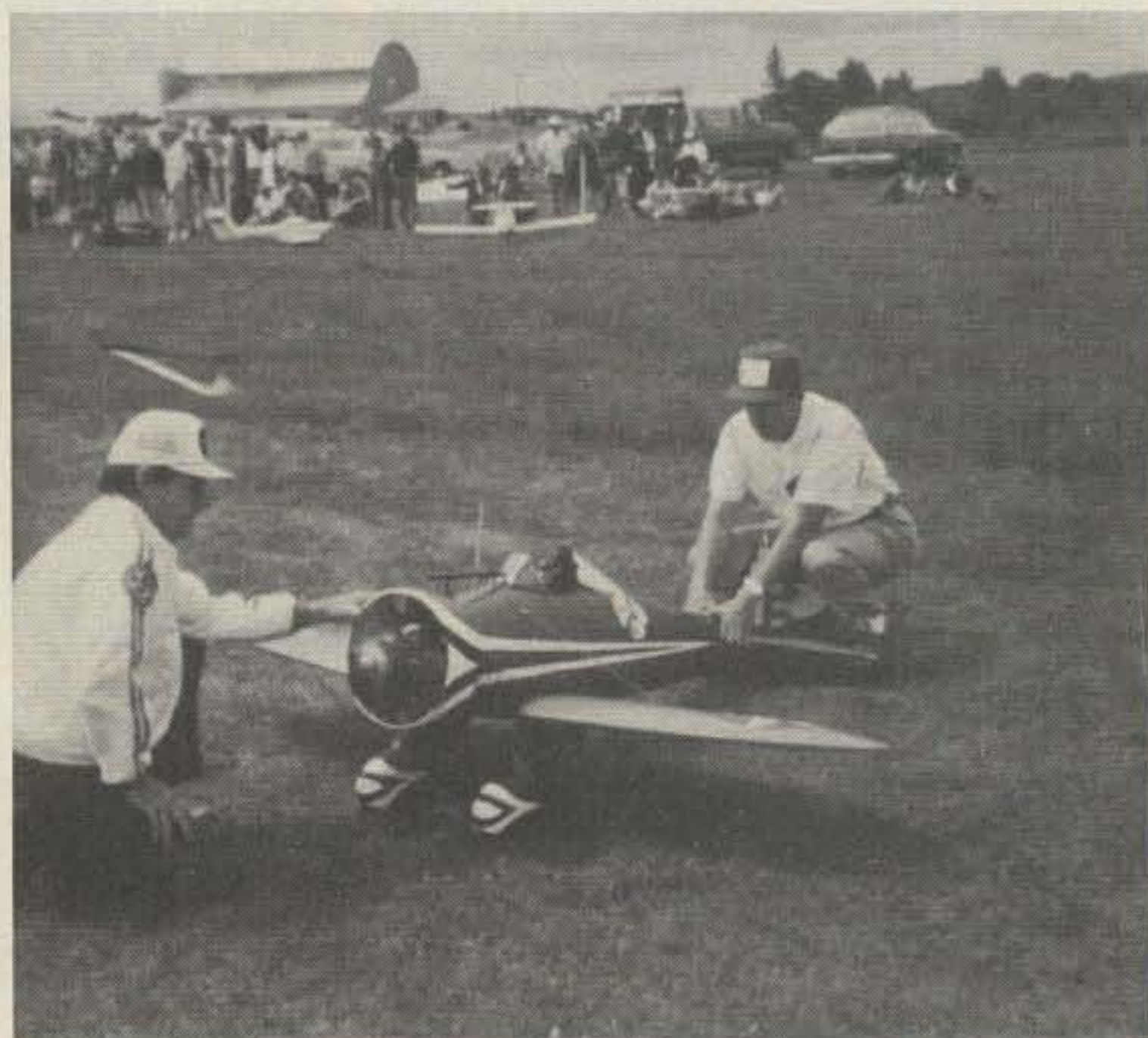
A one-fourth full-sized model of a WWII fighter is started up. Constructed of balsa, plywood, and thin aluminum and covered with fabric, the plane uses a chain-saw engine and two-cycle mix fuel for power. A four-channel R/C rig controls ailerons, rudder, elevator, and engine speed.
