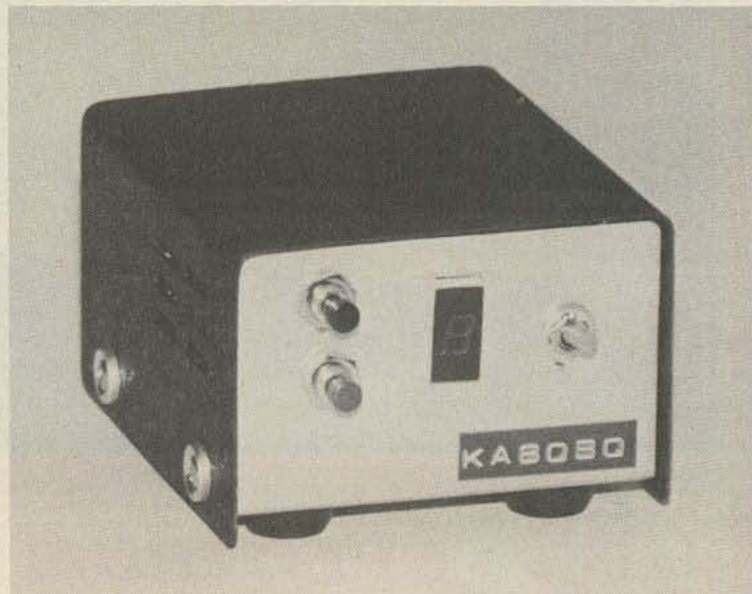
Photo B. Front panel and cabinet for the ID timer.
