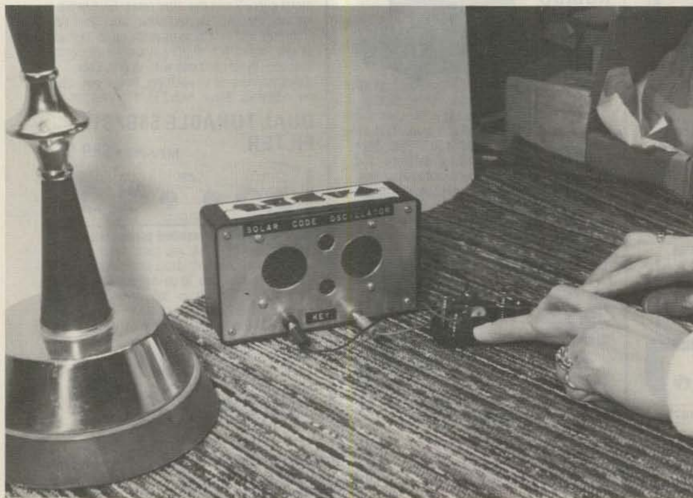
Photo A. This little solar code oscillator may be operated in the sun or under a regular reading lamp. Sufficient volume is obtained from a small 8-Ohm PM speaker.
