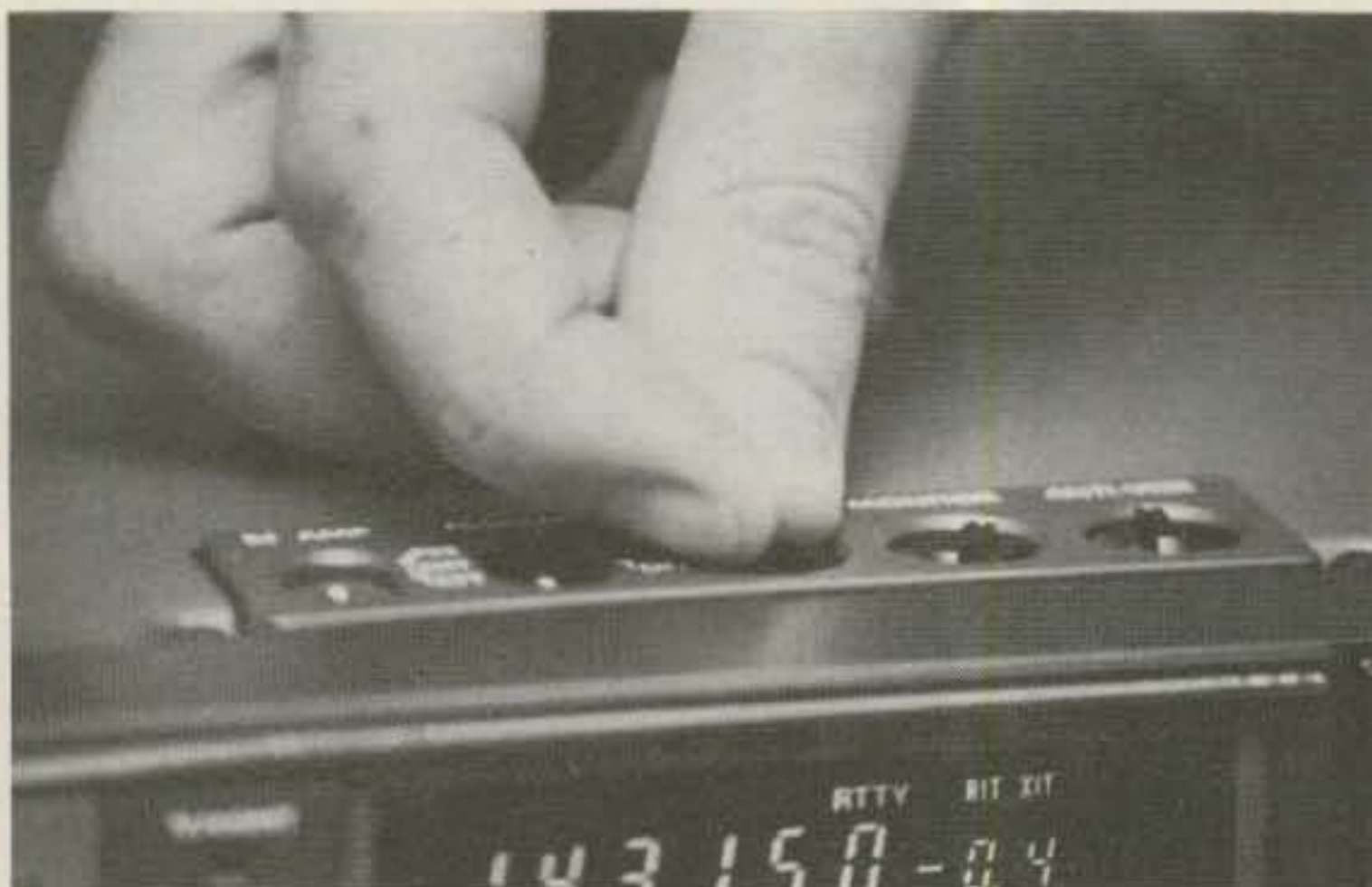
The non-ergonomic top-panel controls. Perhaps they are recessed because Icom knows hams love to stack equipment to the ceiling. But if you cover them up, how do you get to them?
