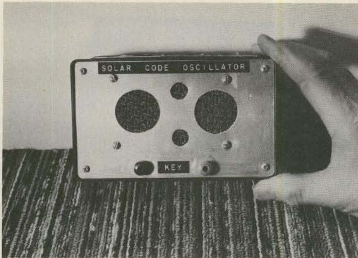
Photo D. Close-up view of the small oscillator. In this model, a metal front panel was used. The speaker holes may be drilled out with a small bit or with a circle cutter.
