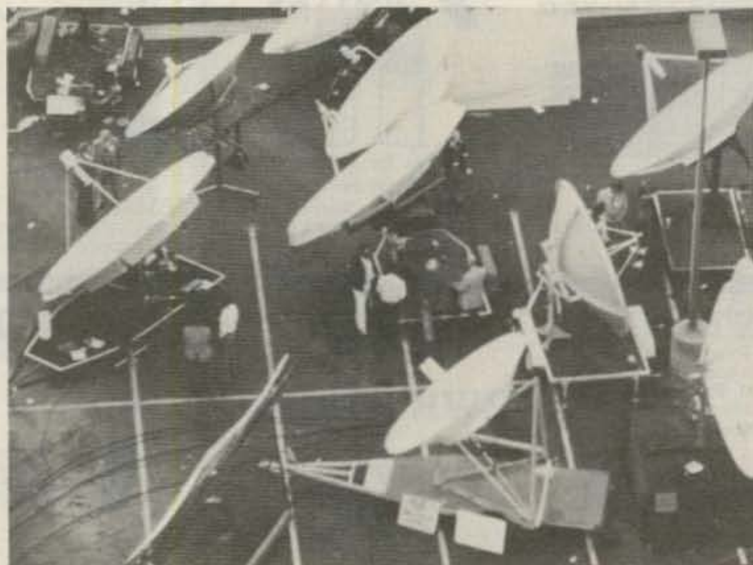
Photo A. Follow the crowd and point your antenna in the same general direction as everyone else. Be sure to include declination in your azimuth calculation.
