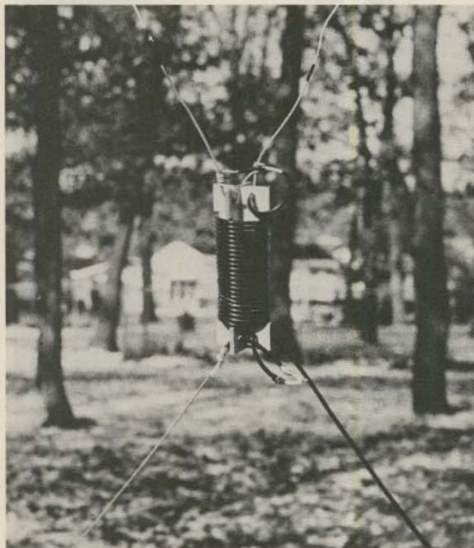
Photo C. The Helix hanging from the delta loop, the antenna wires and feedline attached but not yet taped.
