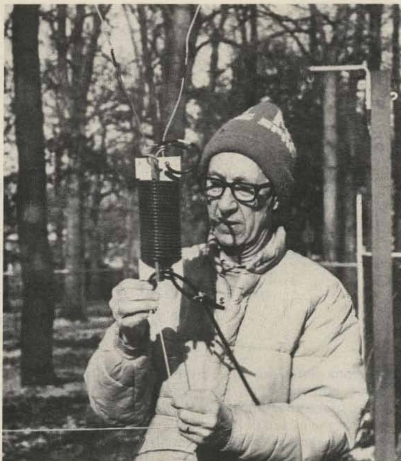
Photo D. The author tying on light nylon anchor line before hauling the delta loop skyward. At K9AZG, the Helix hangs about 10 feet off the ground, with excessive wind sway prevented by the "anchor," a brick lying on the ground beneath the antenna.
