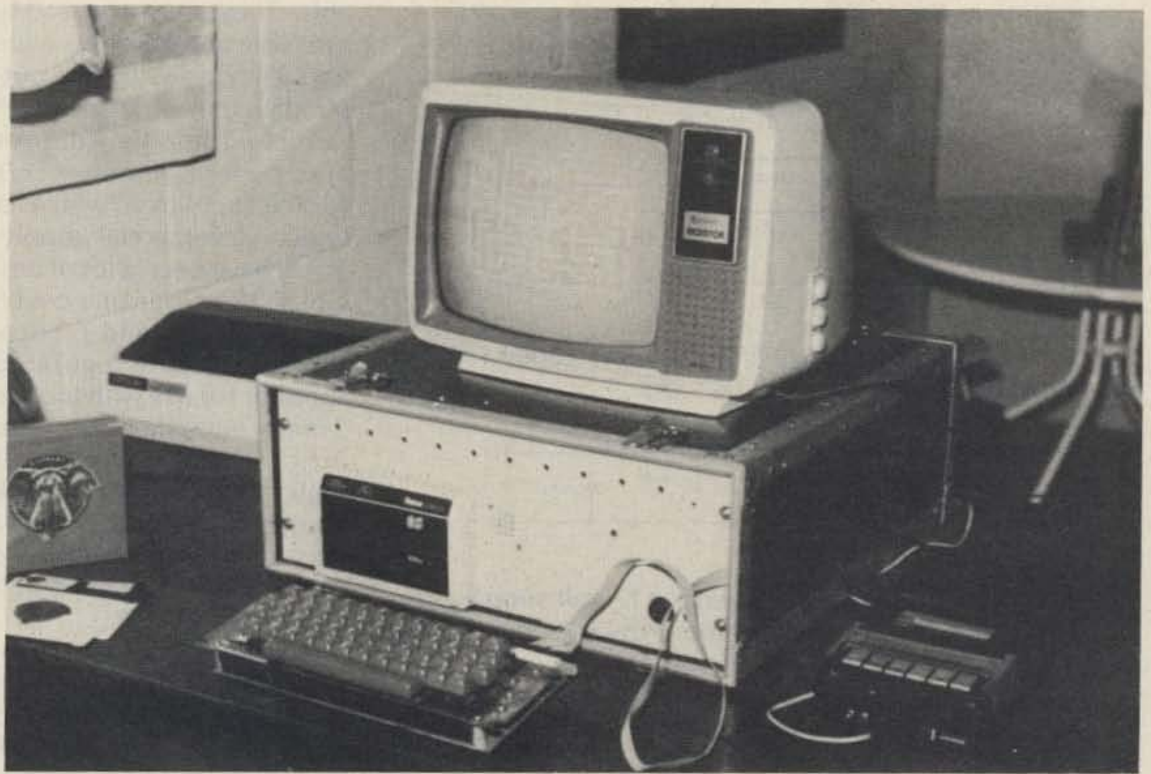
Photo A. Front view of the case with the system in operation. The hole pattern to the right of the disk drive is for the speaker.
