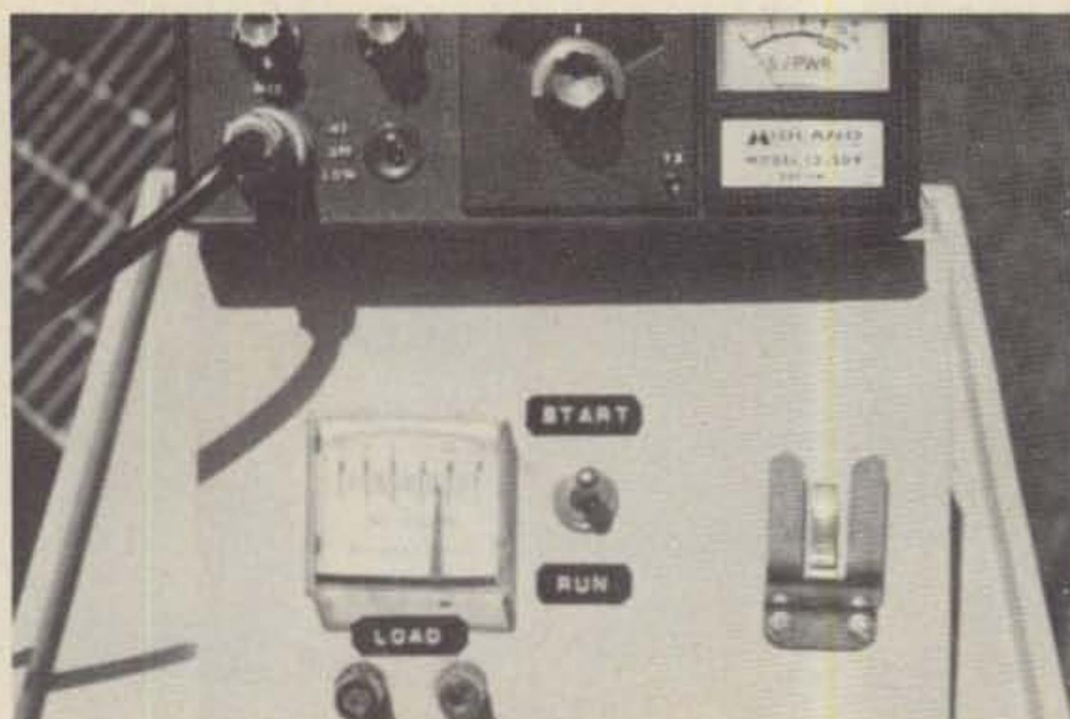
Photo B. The operator's control panel. The transceiver is running directly off the solar panel (see text).
