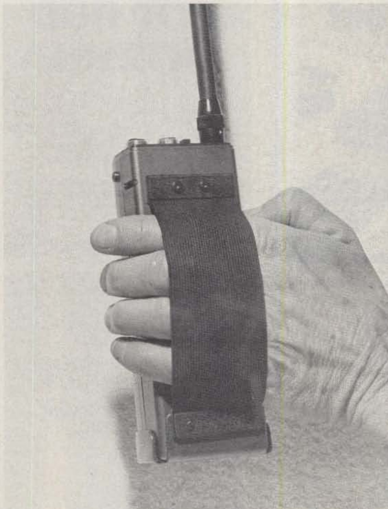
Photo A. Rear view of HT, showing attachment of elastic band to metal clip at base.
