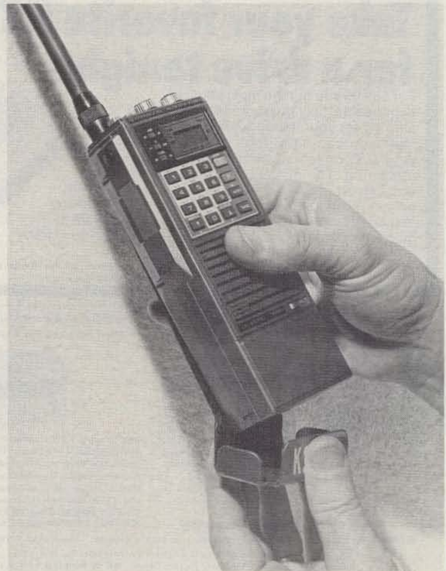
Photo B. The felt-lined metal clip is easily removed for battery pack changing or charging.
