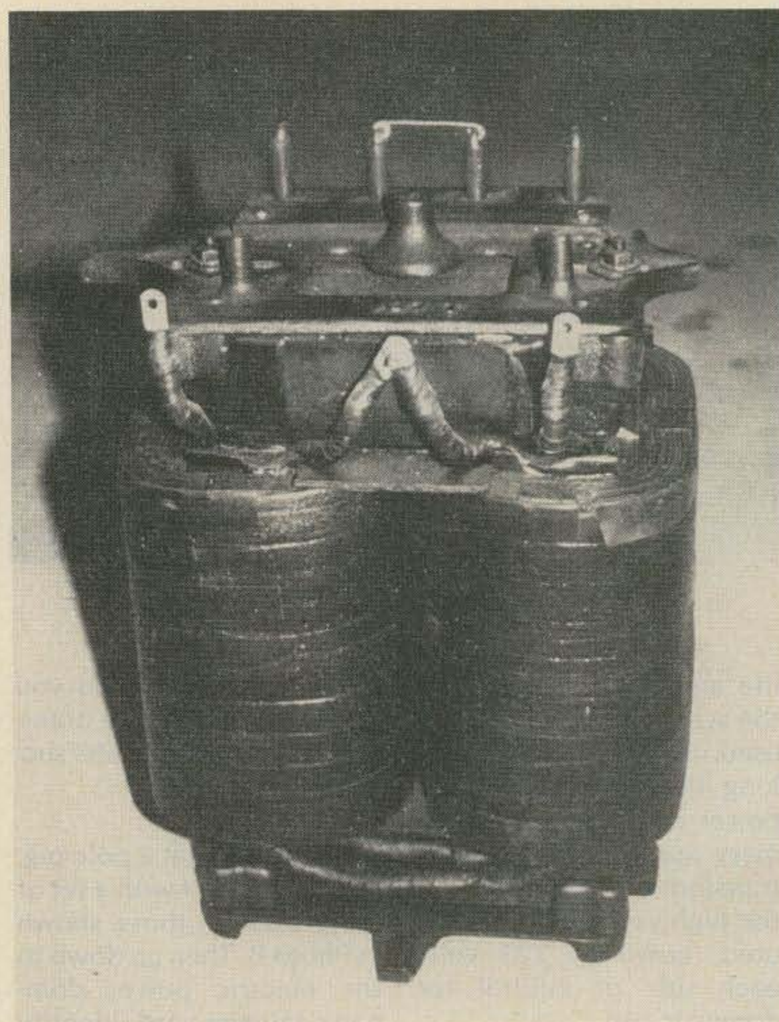
Photo E. View showing 240-volt terminals.
