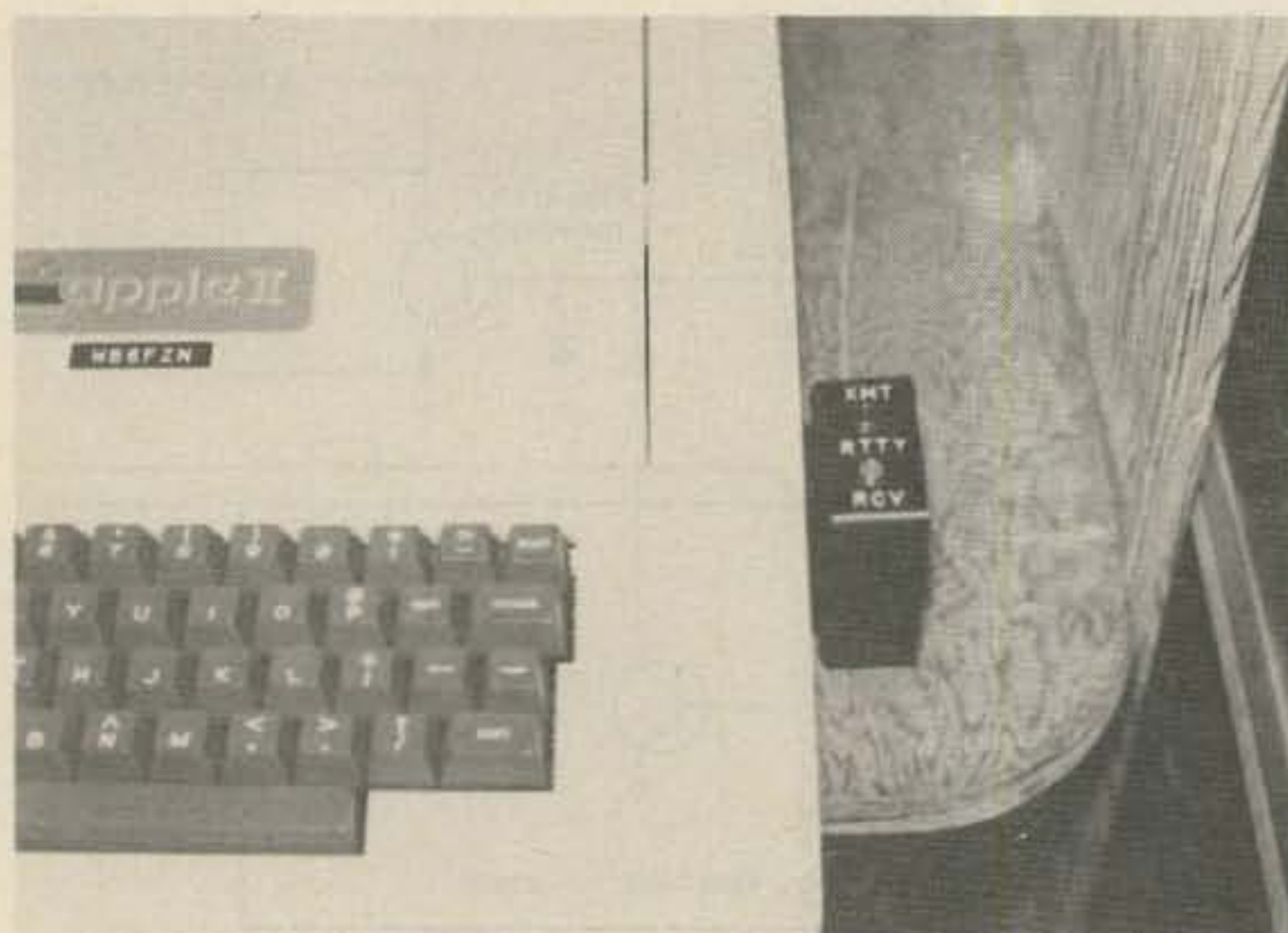
Fig. 5. LEDs box attached to the Apple's case with Velcro.
