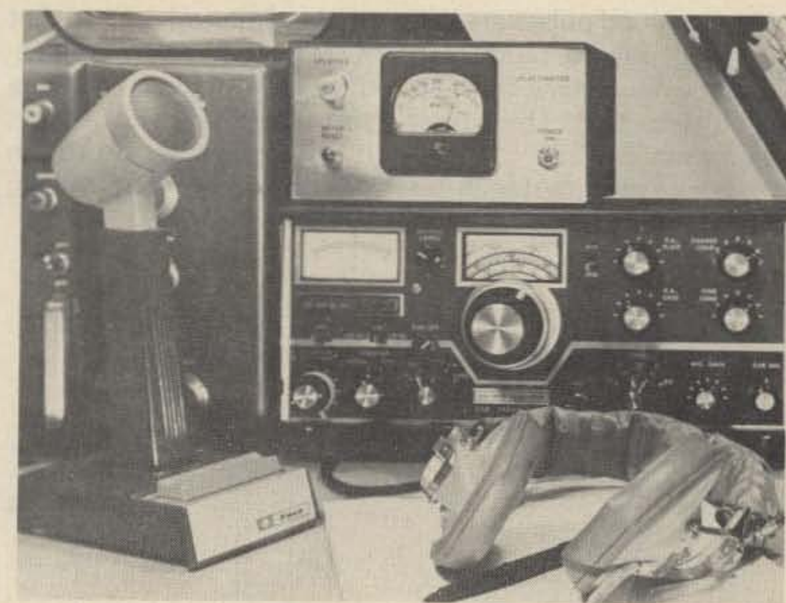
Photo D. Although it fits nicely on top of the transceiver, the Splattometer can be placed anywhere within the operator's field of view. It doesn't need constant attention; when you splatter, it lets you know with a bright flash.
