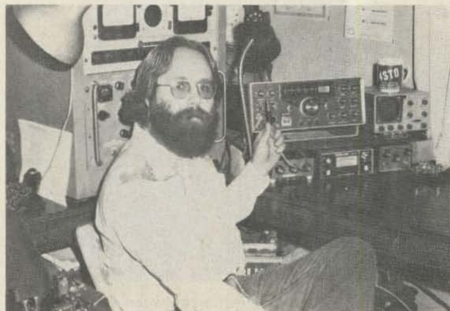
Photo D. Transmitting RTTY is simplicity itself. Just plug the AFSK output from the TU into the mike jack of the transceiver, and enjoy!
