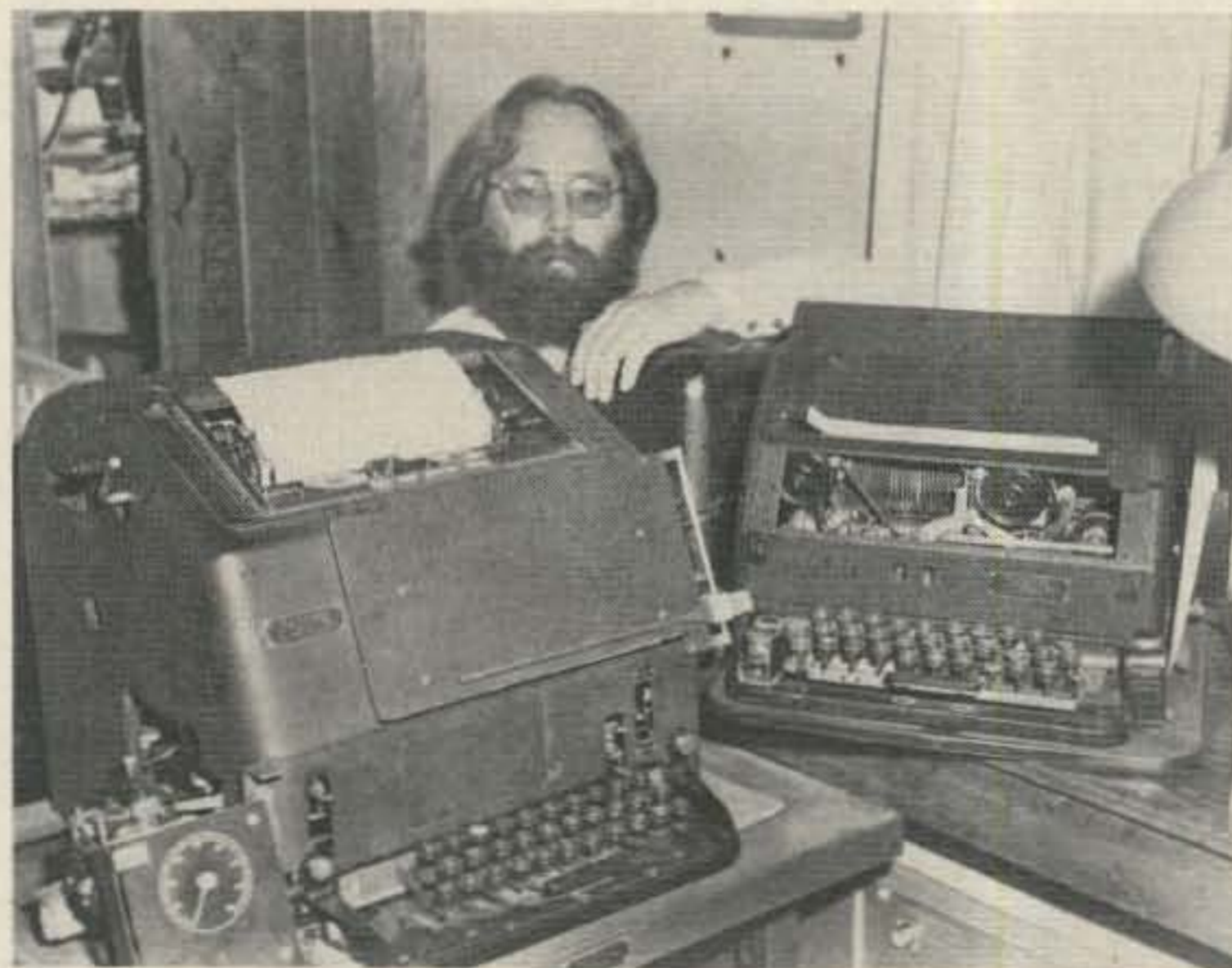
Photo A. On the left is the Model 19 printer, with the Model 14 tape reperf. to the right. The sour look on my face is representative of how you will feel after lifting your first printer! But remember, the price is right.
