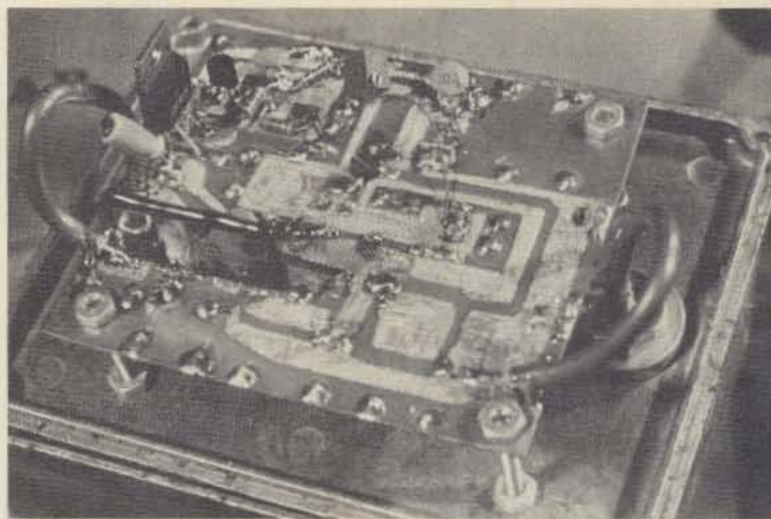
Fig. 3. The mixer, MRF-901 oscillator, and broadband amplifier fit on a homemade PC board.
