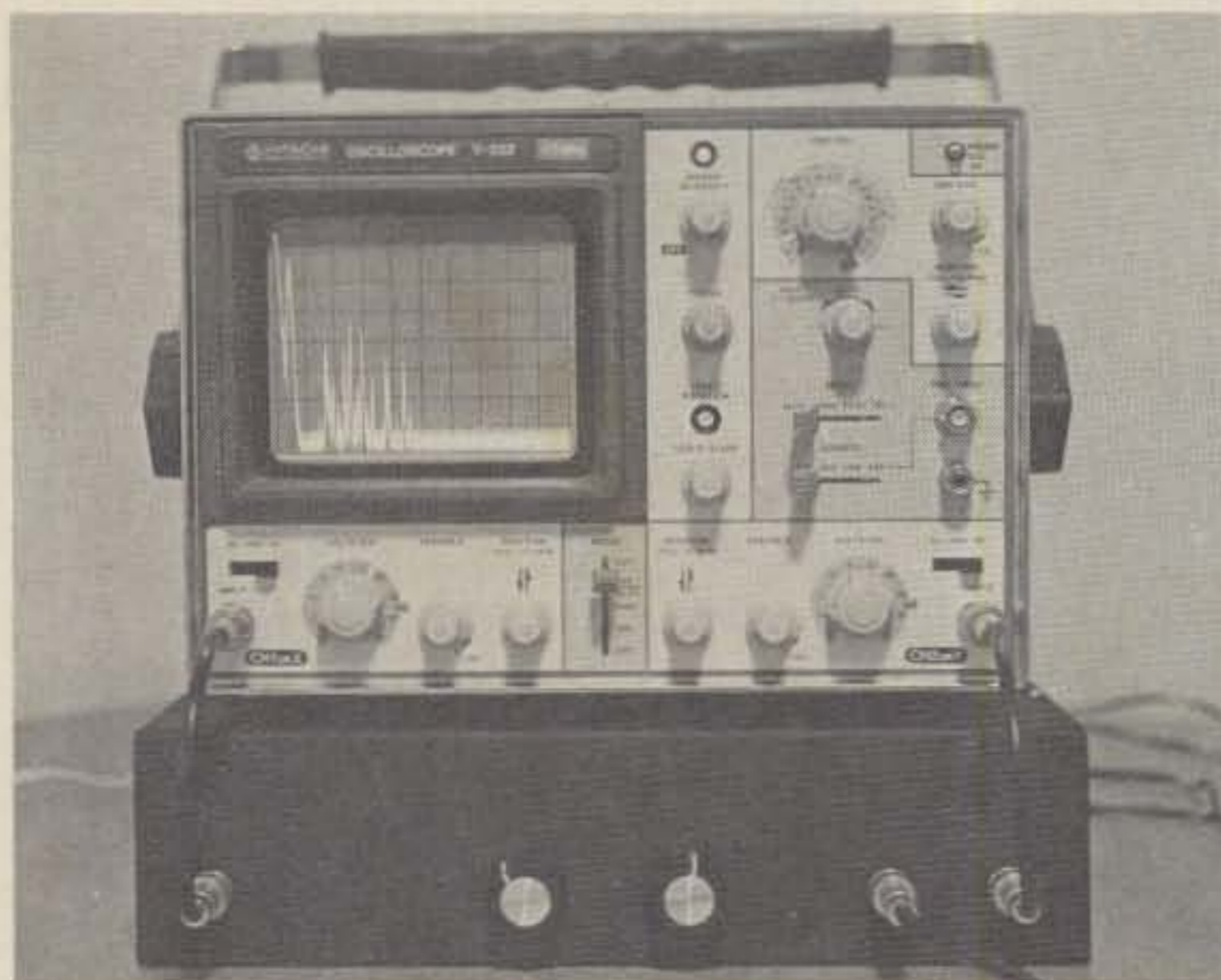
Photo A. High frequency spectrum analyzer covers 0 to 60 MHz.
