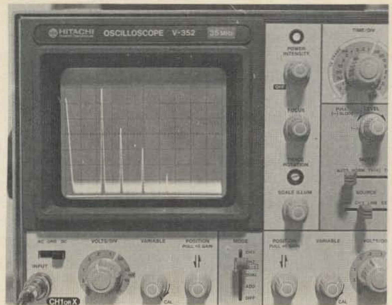
Photo C. Same rf signal on the spectrum analyzer. Second harmonic is only 26 dB below the fundamental. Don't put this signal on the air!
