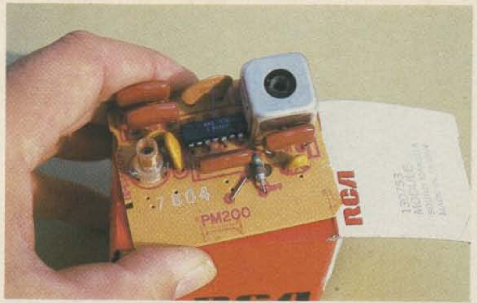
Fig. 4. Known by TV servicemen as the PM200, this small card holds nearly an entire TV-set sound section. It's a natural for cheap satellite audio recovery.
