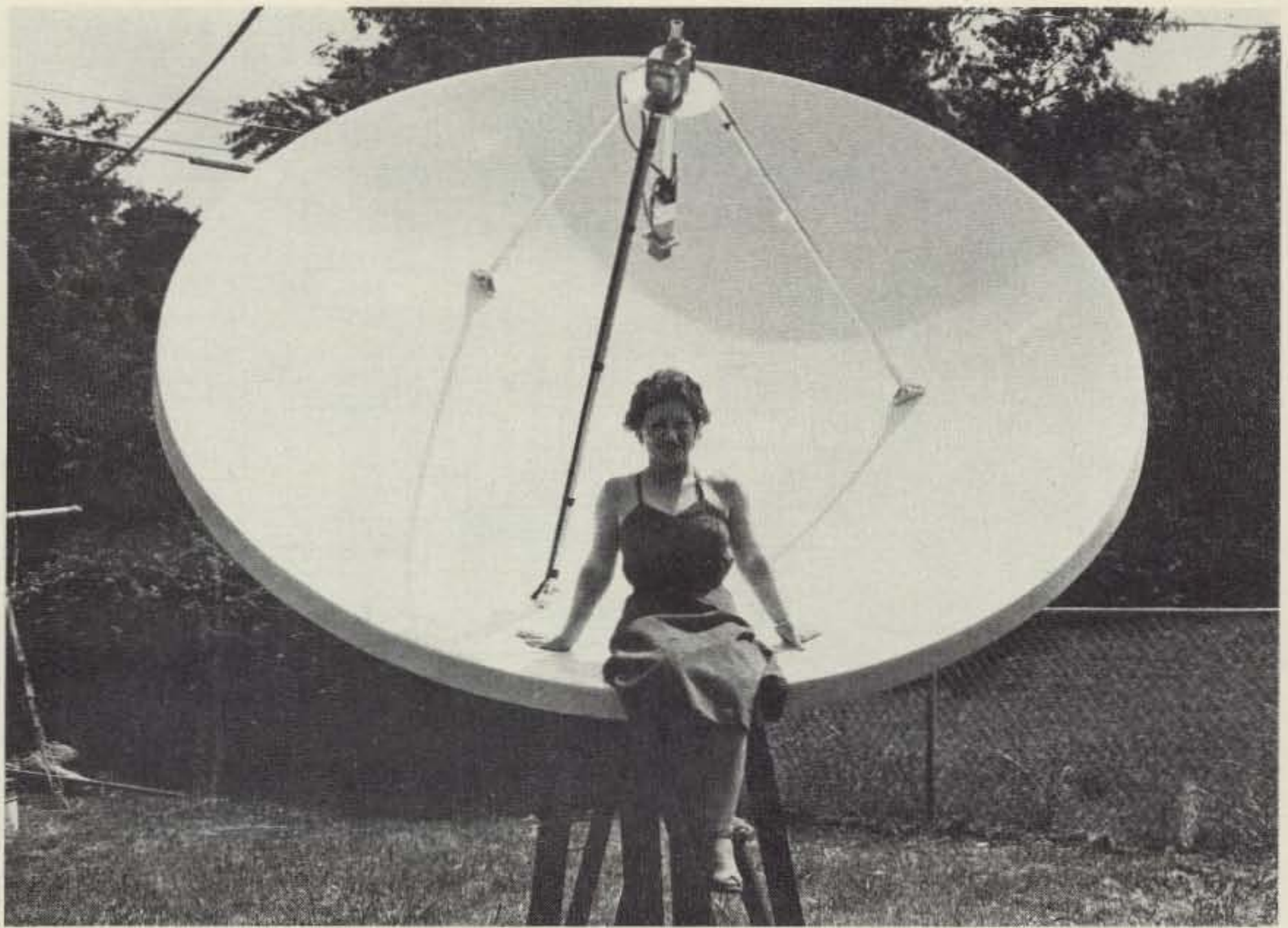
Deborah Franklin tries on a 10' parabolic dish fitted with an Avantek LNA and 3.7-to-4.2-GHz downconverter described in the text.
