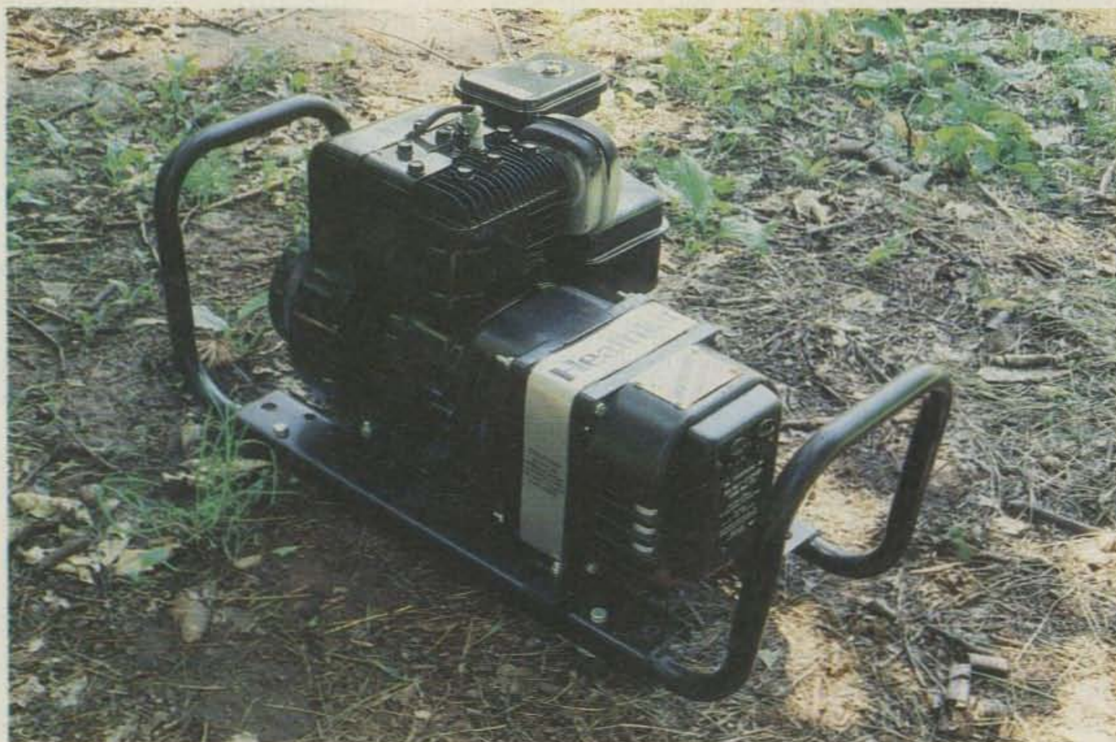
Heath's GU-1820 ac generator.
