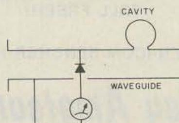
Fig. 2. Cavity wavemeter circuit diagram.
