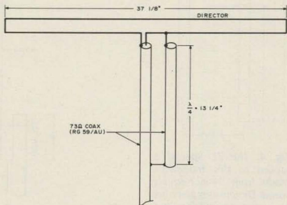
Fig. 3. Dimensions given for the 1-to-1 balun are for 146.5 MHz using coax with a velocity factor of .66. For other frequencies, balun length in inches is calculated from  $2952 \times .66 \div \text{MHz}$ .
