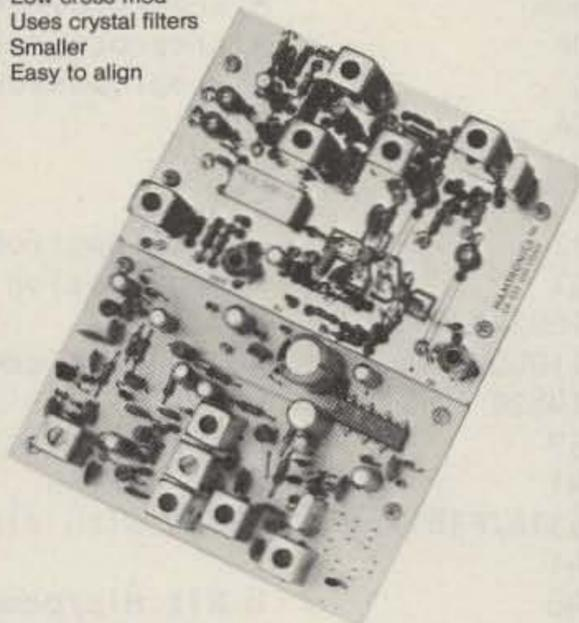
R75A\* VHF Kit for monitor or weather satellite service. Uses wide L-C filter. -60dB at ± 30 kHz..... \$69.95
