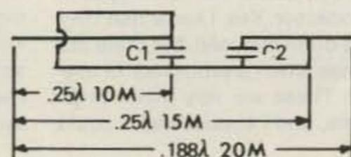
3. Extend element to 1/4 wave on 15M. Fold back and decouple tip with C2.
