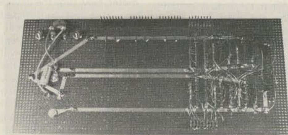
Photo B. Bottom view of the I/O board. The  $2 \times 20$  header is at the right. The electrolytic and ceramic capacitors for the regulator circuit are at the left. Power buses are  $1/8$ "-wide adhesive copper strips made by Circuit-Stik™. Small white spots are paint used to mark correct positions for the sockets and headers. Terminating resistors (input port) were added after the photograph was taken.
