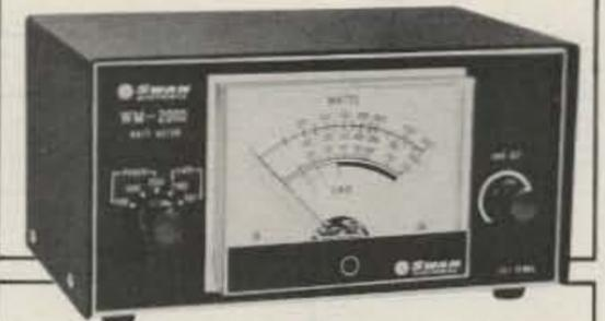
**MOBILE WATT METER HFM-200** with remote directional coupler reading 20 or 200 watts. 3.5-30 MHz. Illuminated, with VSWR scale.
