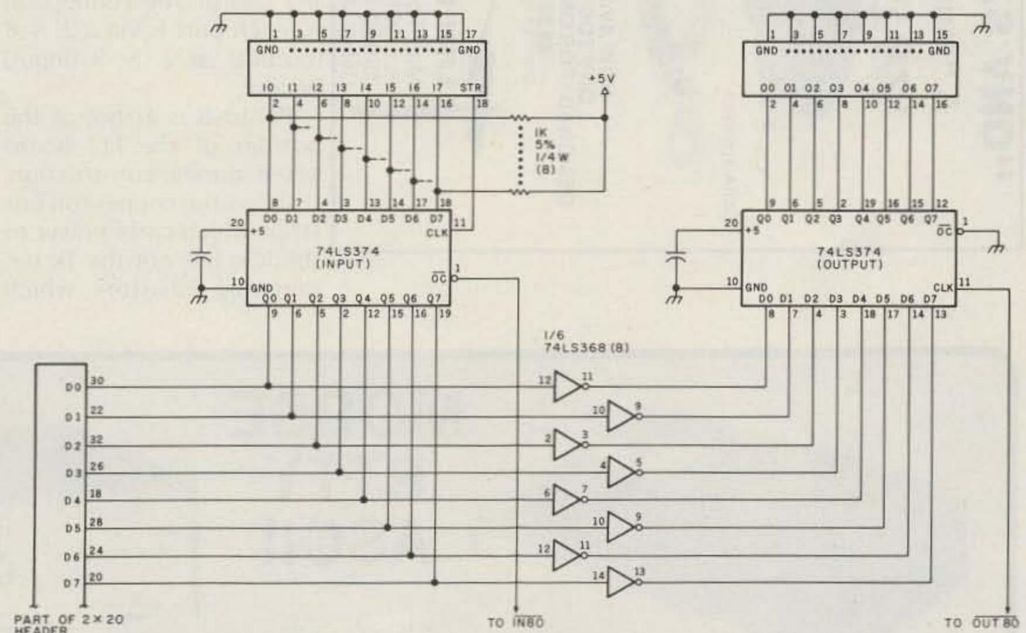
Fig. 2. Schematic of port function circuit. Unmarked capacitors are 0.1-uF, 25-volt disc ceramic. Tie enable inputs (pins 1 and 15), unused data inputs (pins 2, 4, and 6), and ground pin (8) of the 74LS368s to ground. Tie +5-volt pin (16) of each 74LS368 to +5 volts and bypass to ground via a 0.1-uF, 25-volt disc ceramic capacitor.
