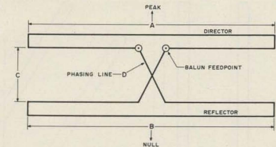
Fig. 2. The ZL Special is composed of two phased driven folded dipoles made from 300-Ohm twinlead. The driven director is 4.4% shorter than a half-wave element and the reflector 1.7% longer. Formulas for dimensions in inches:  $A = 5446 \div \text{MHz}$ ;  $B = 5794 \div \text{MHz}$ ;  $C = 1266 \div \text{MHz}$ ;  $D = 1266 \div \text{MHz}$ . Dimensions for 146.5 MHz are:  $A = 37\text{-}1/8''$ ;  $B = 39\text{-}1/2''$ ;  $C = 8\text{-}5/8''$ ;  $D = 8\text{-}5/8''$ .
