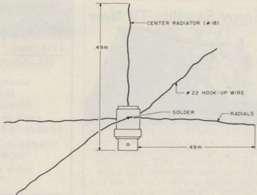
Fig. 1. The Flexi-Plane with BNC connector.
