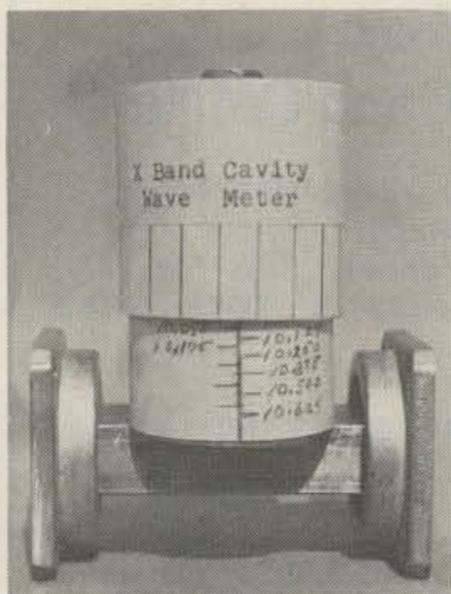
Photo A. Cavity wavemeter for X-band.
