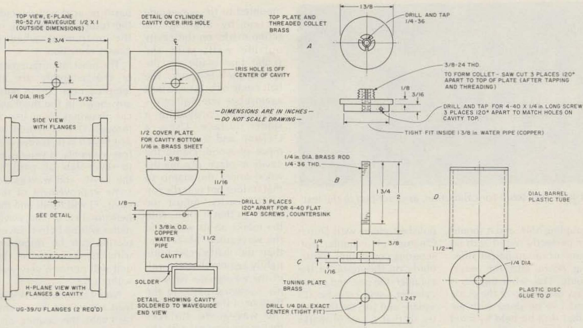
Fig. 3. Construction details for cavity wavemeter.
