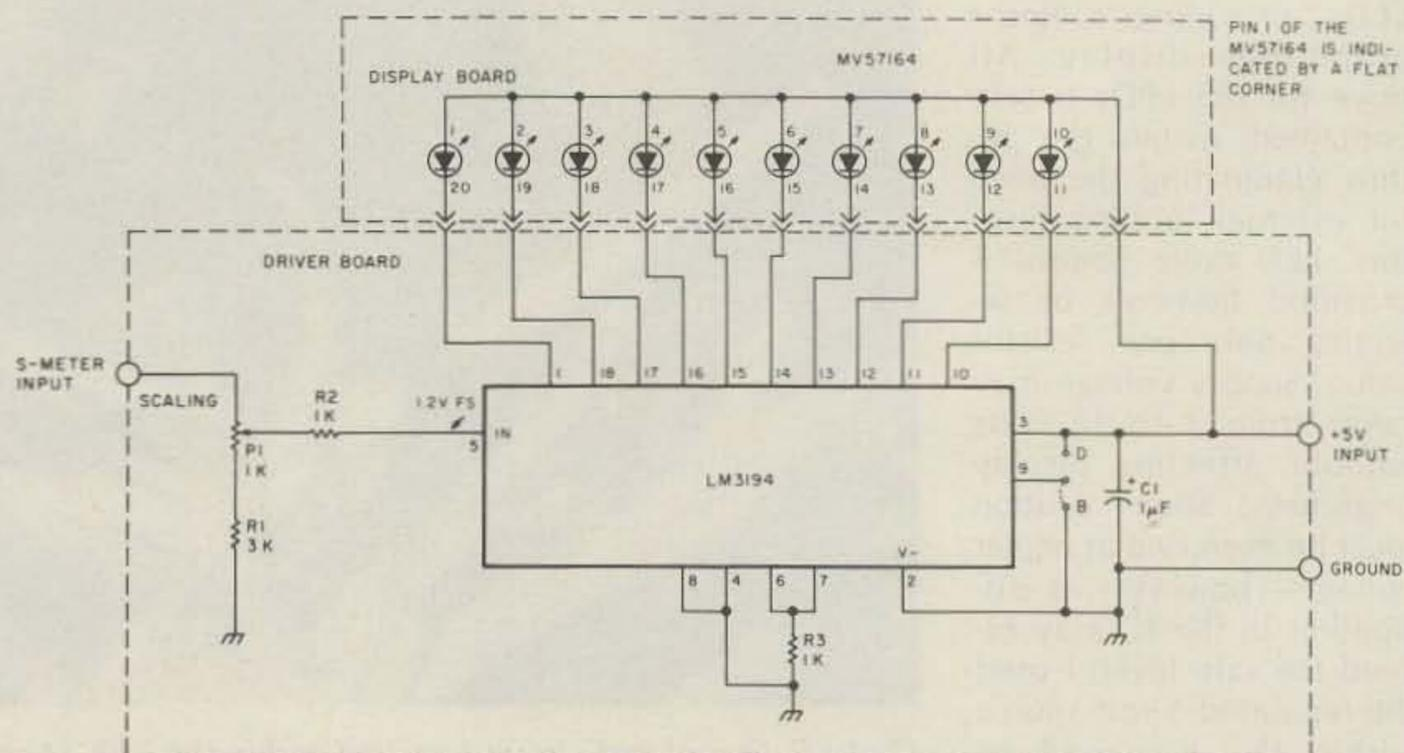
Fig. 1. Schematic of bar-graph S-meter.
