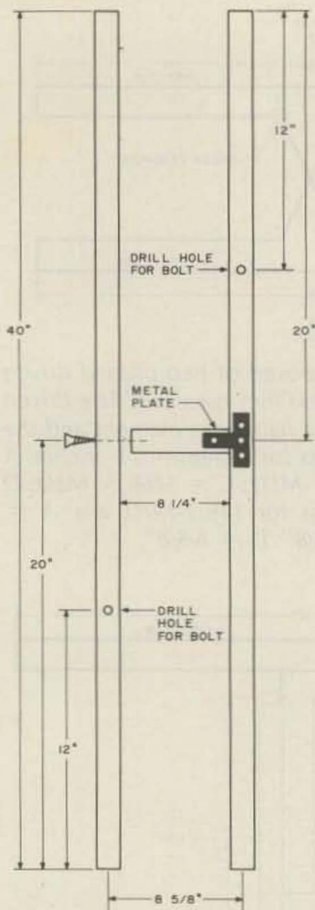
Fig. 4. The ZL Special is tacked to this framework made from 3/4-inch-square wood. Dimensions given are for an antenna cut for 146.5 MHz.
