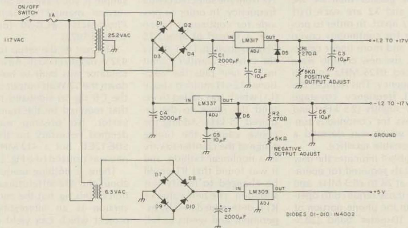
Fig. 1. Tri-voltage power supply schematic.
