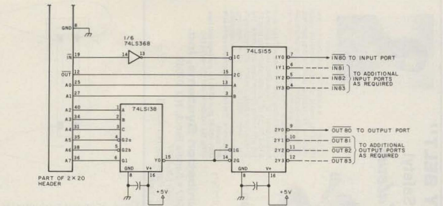
Fig. 1. Schematic of strobe generator circuit. Unmarked capacitors are 0.1-uF, 25-volt disc ceramic.
