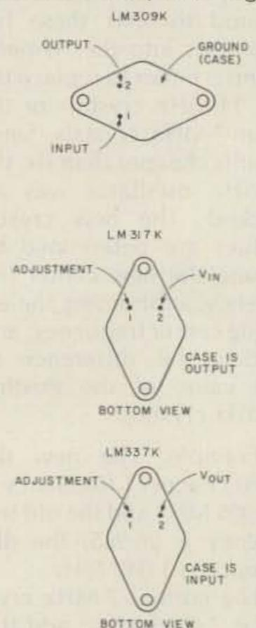
Fig. 2. Pin connection for the LM309, LM317 and LM337 voltage regulators (TO-3 packages).
