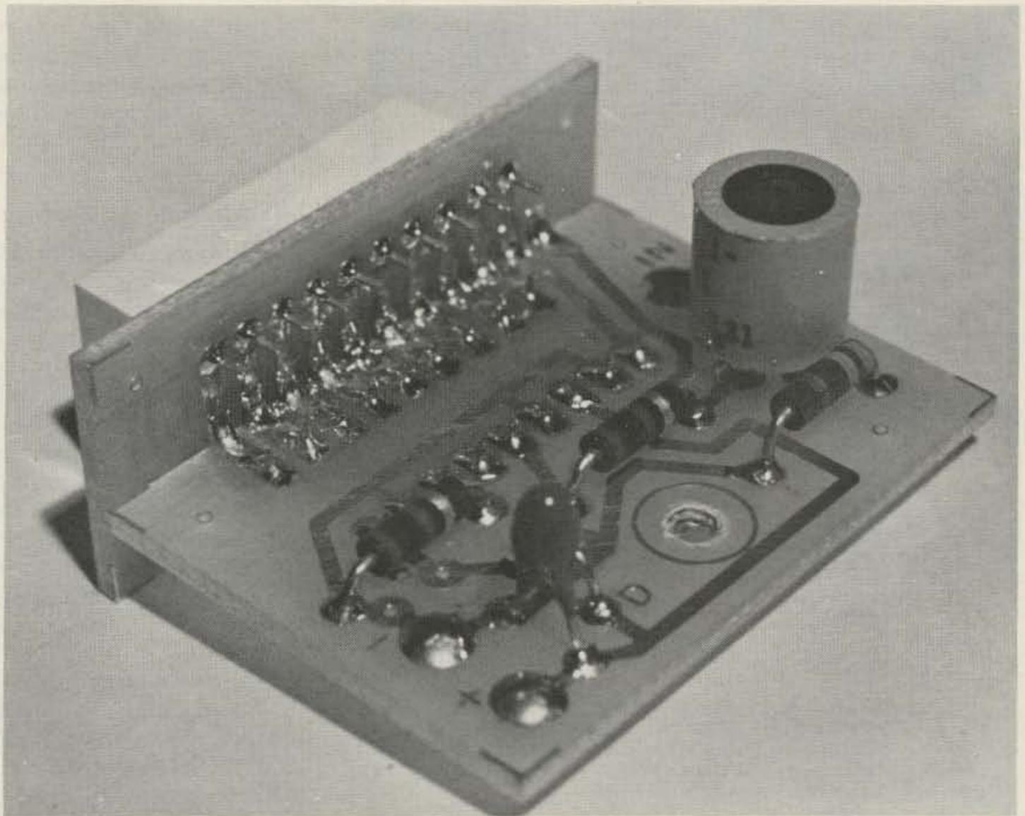
Photo B. The two boards joined using the rows of large pads. The IC is mounted underneath the board.
