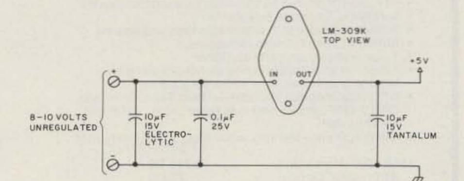
Fig. 3. Schematic of power-supply regulator. The 10-uF capacitors are tantalum and electrolytic; the 0.1-uF capacitor is disc ceramic.
