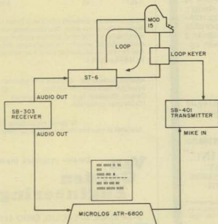
Fig. 1. Station wiring.
