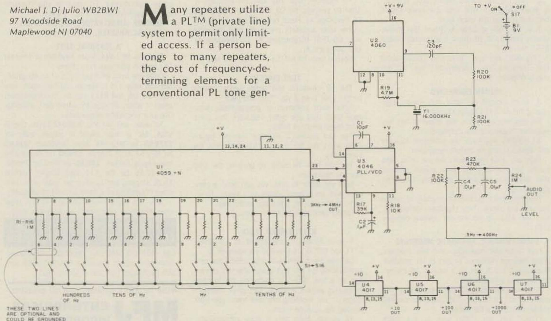
Fig. 1. Synthesized tone generator schematic.
