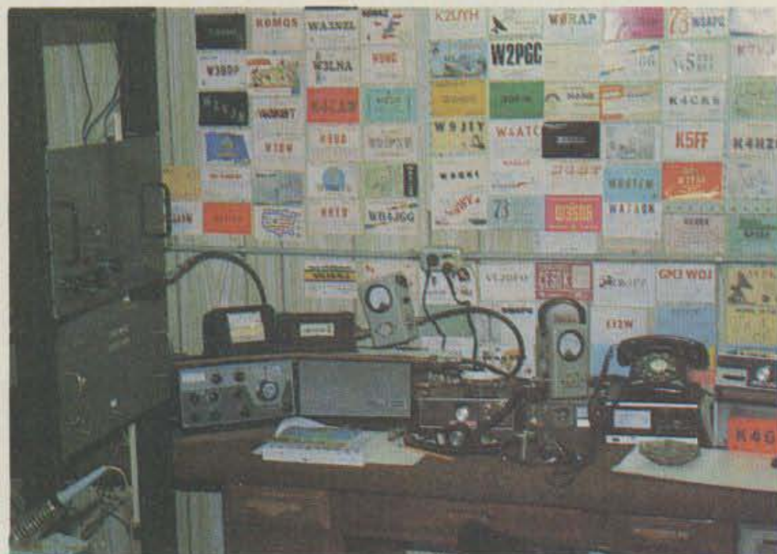
A mix of home-brew and commercial equipment is used to give W8DJY a big signal on 220 MHz.
