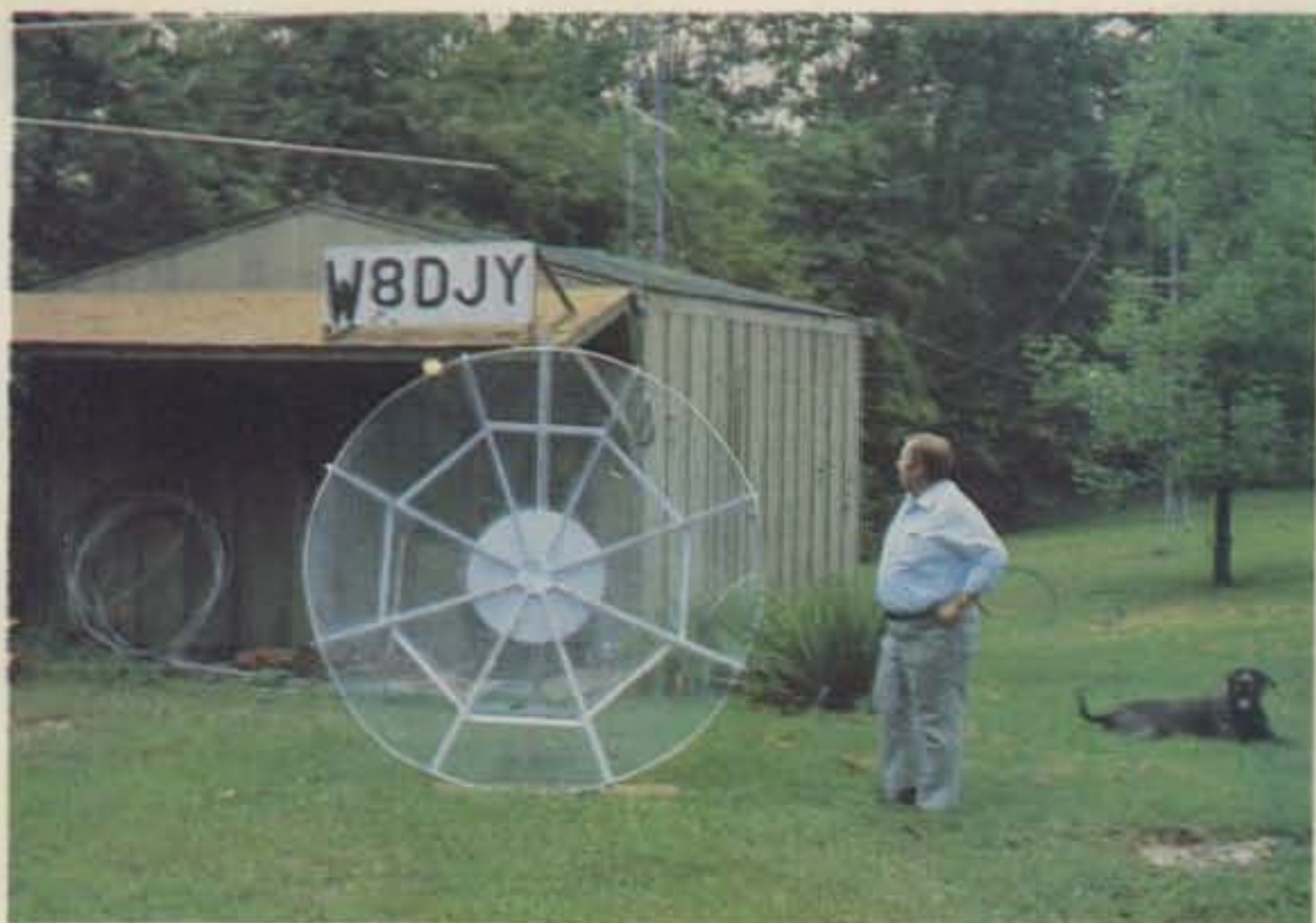
W8DJY spares his family from the squeaks and squawks of ham radio operating by having a separate shack. Inside, there are operating consoles for each of the VHF bands. The 6-foot dish was constructed for less than $100 and will be used on 1296 MHz.
