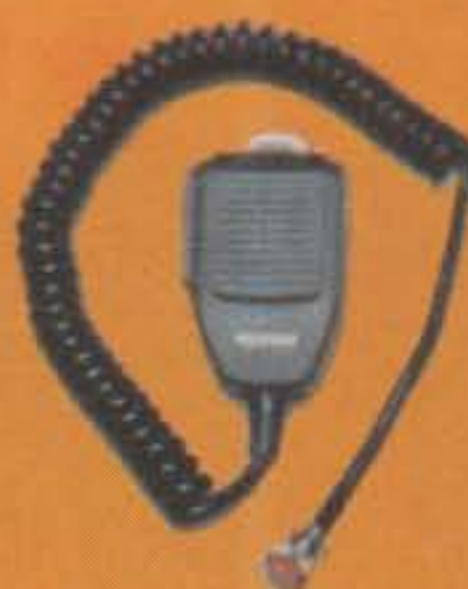
MC-30S (500 \Omega ) dynamic noise-cancelling hand microphone. Also available, MC-35S (50 k \Omega ).
