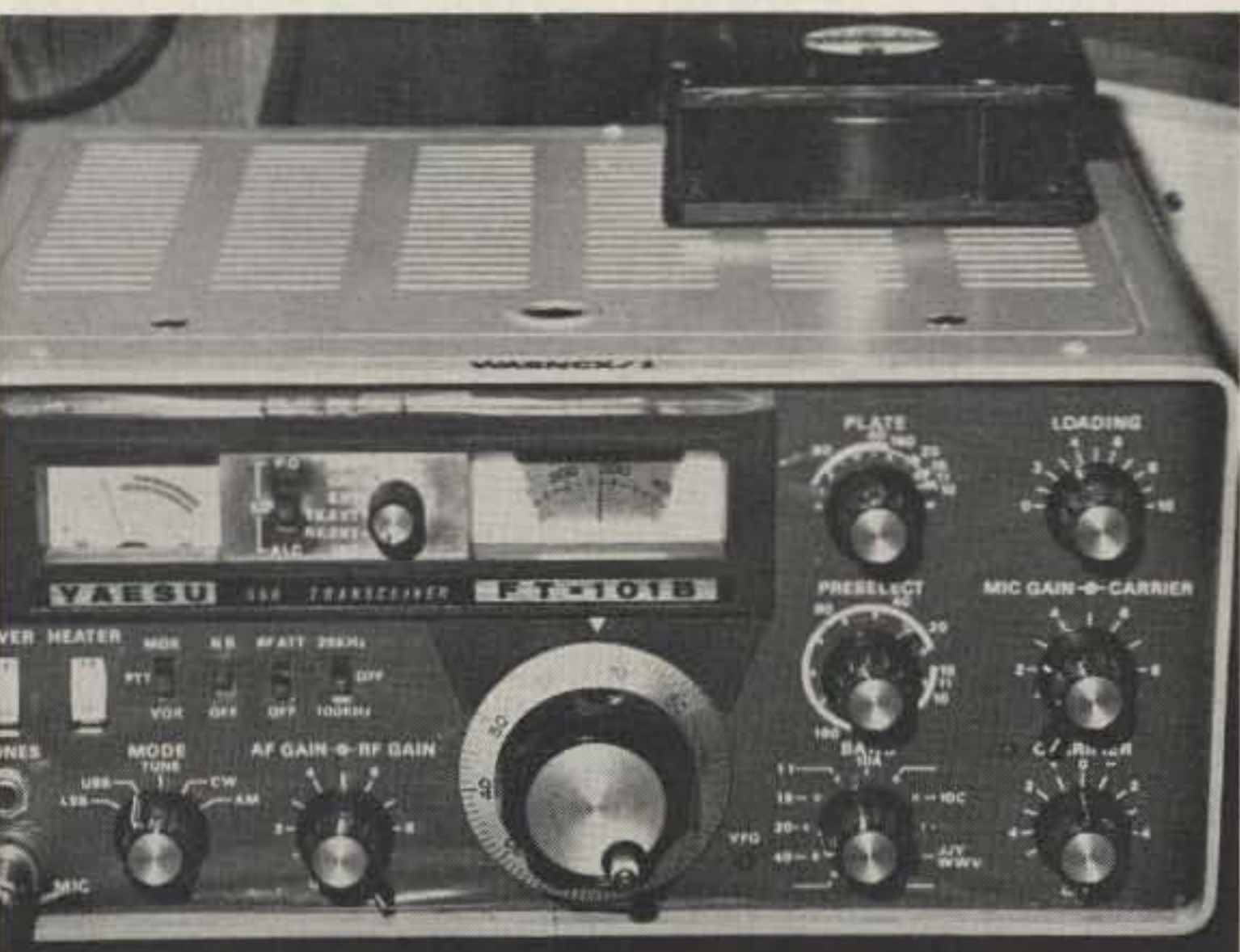
Photo C. This Muffin fan sits over the finals and is mechanically damped by four felt feet.
