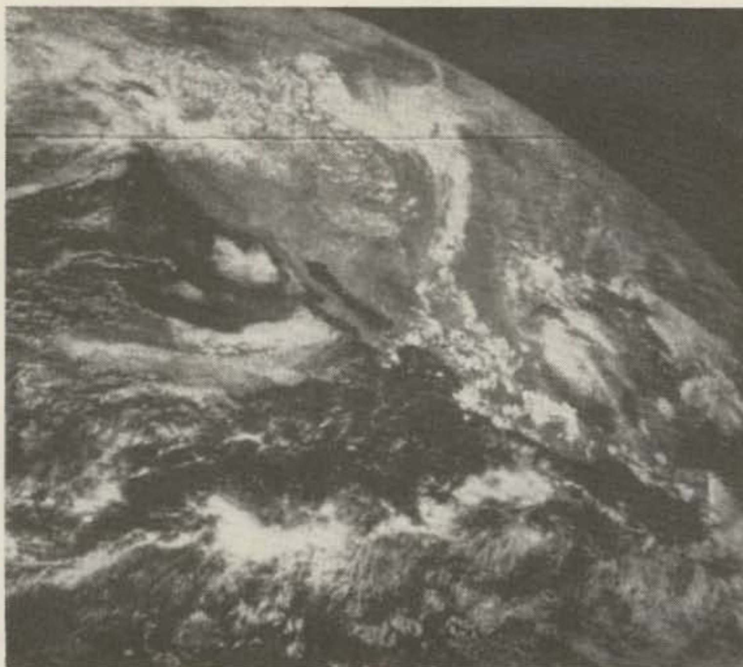
A weather satellite image received with the signal centered in the receiver's passband. All other conditions were identical to those prevailing in the photo where the signal was some 15 kHz off frequency.
