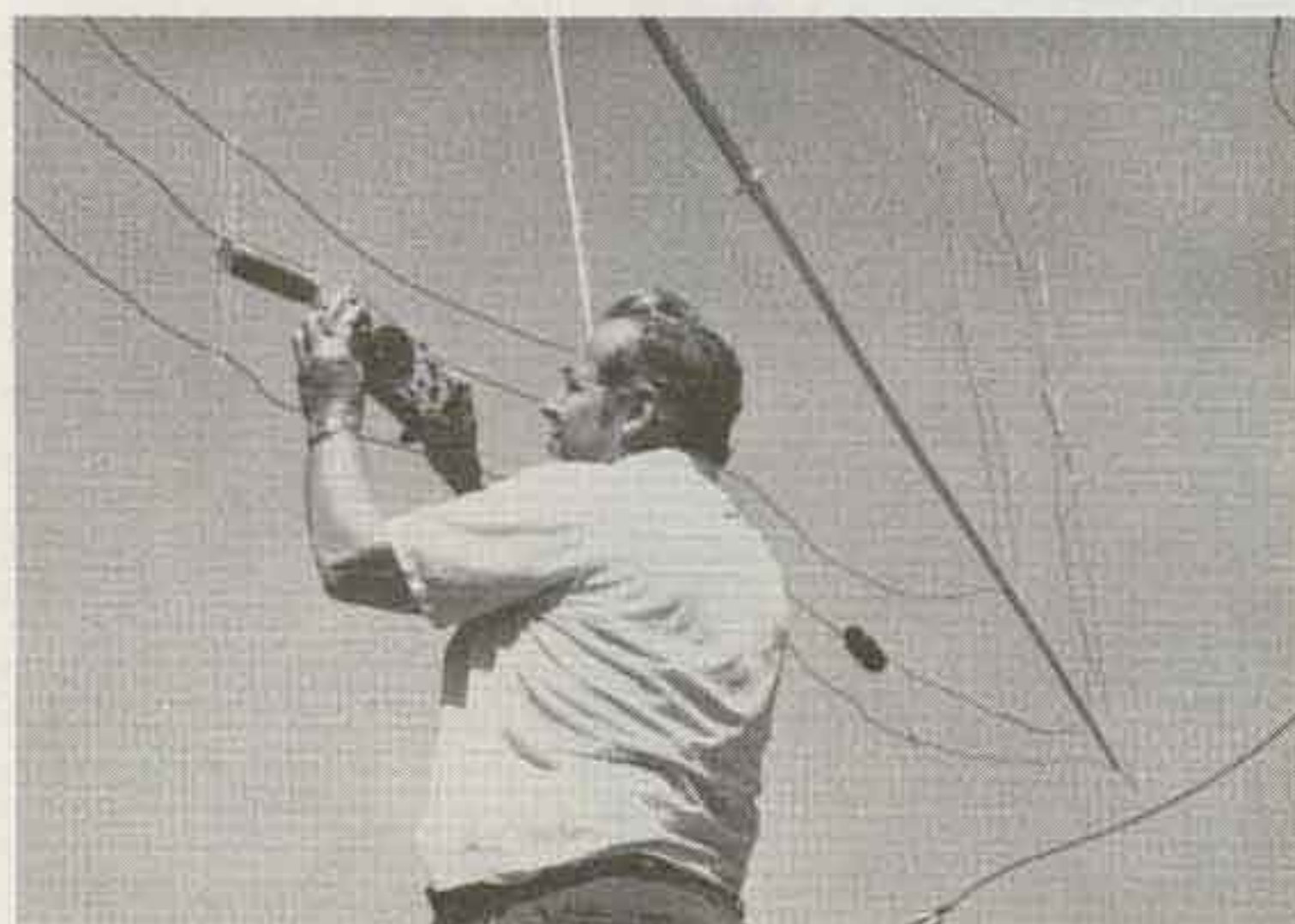
Here the antenna tuning is being checked after two years of operation, using a home-brew dip meter-transistor checker.
