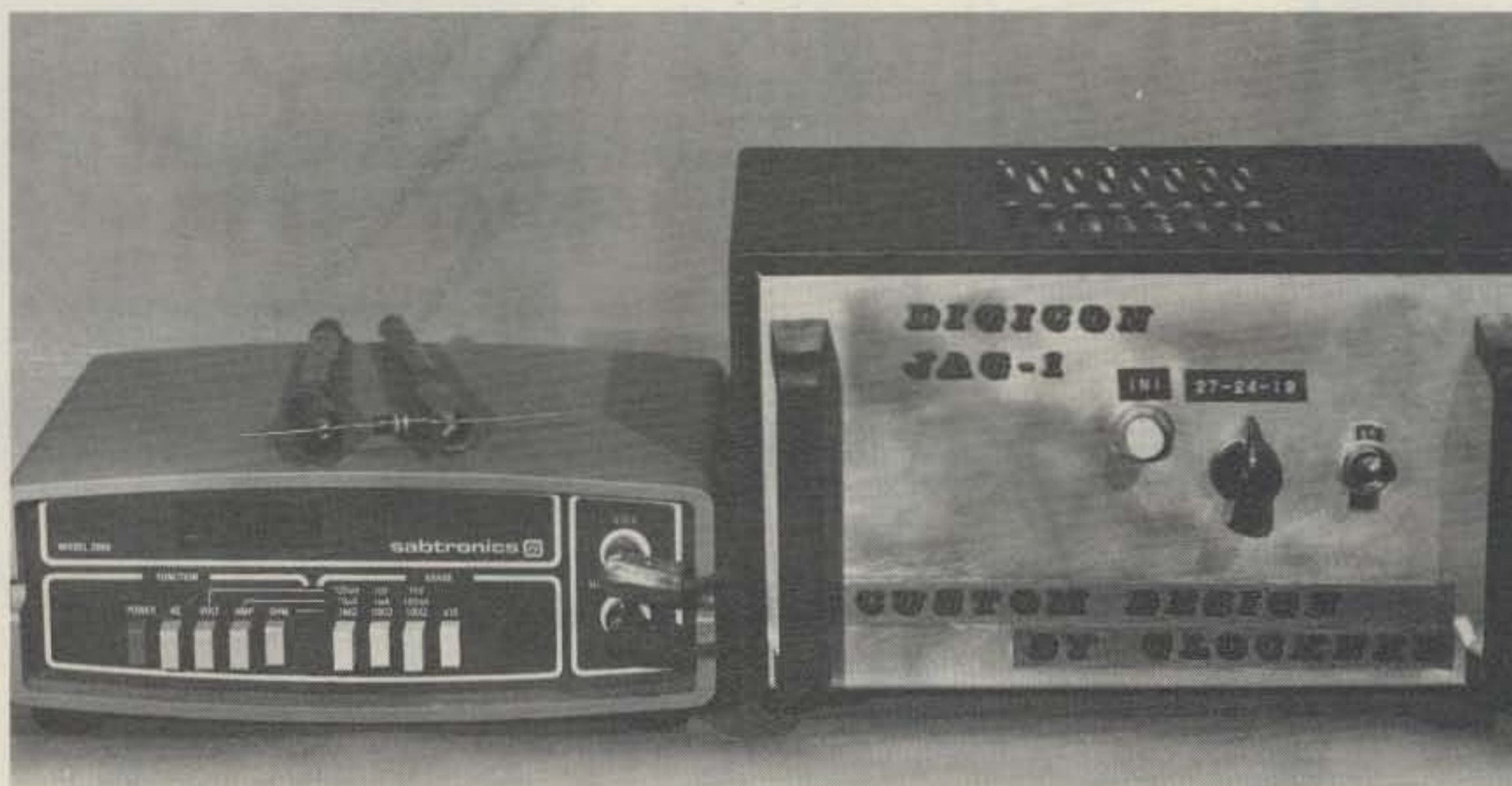
The converter at work. The DMM indicates -108.5 Ohms. (The minus sign is peculiar to the Ohms reading on this DMM.) When the INI button is pushed, the converter will respond with --(minus) . . . . .
