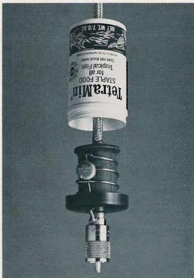
Photo A. The coil protective cover has been removed in this picture to show details of the base coil.
