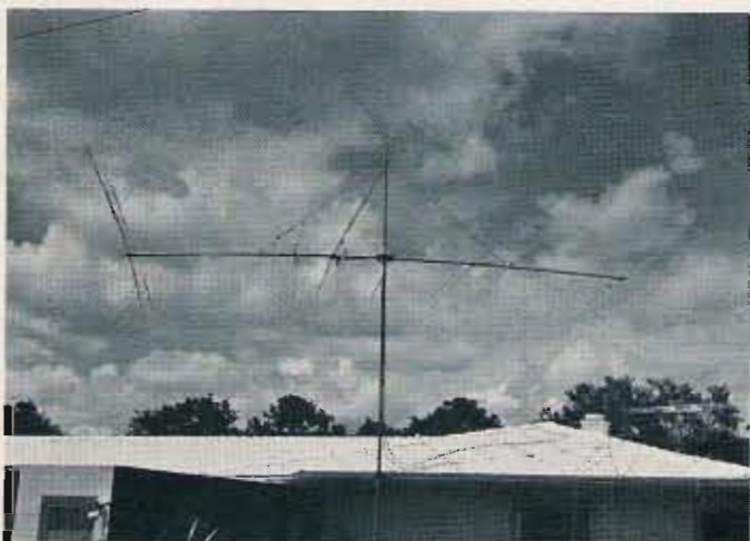
Photo A. A most unorthodox 204BA. Nine elements and two gamma matches radically alter its appearance!
