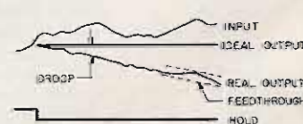
Fig. 6. Representation of the linearity, droop rate, and feedthrough. (Courtesy of Analog Devices, Inc. 3 All rights reserved.)
