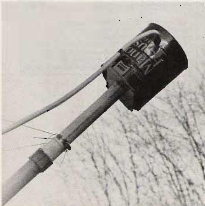
Photo A. This is a feed-horn assembly for use at the 1.7-GHz satellite frequency.
