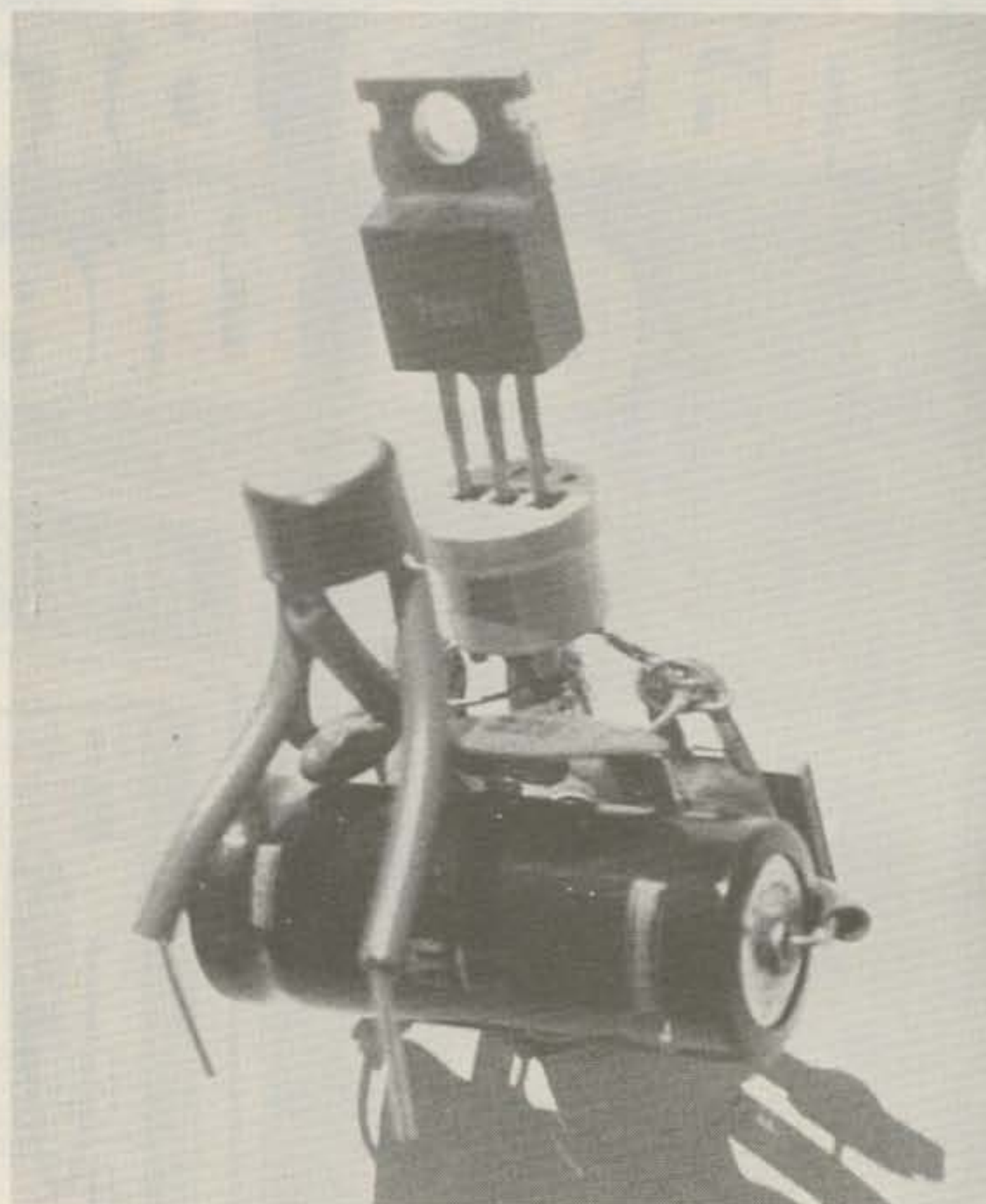
Photo 2. Method of mounting power supply components.
