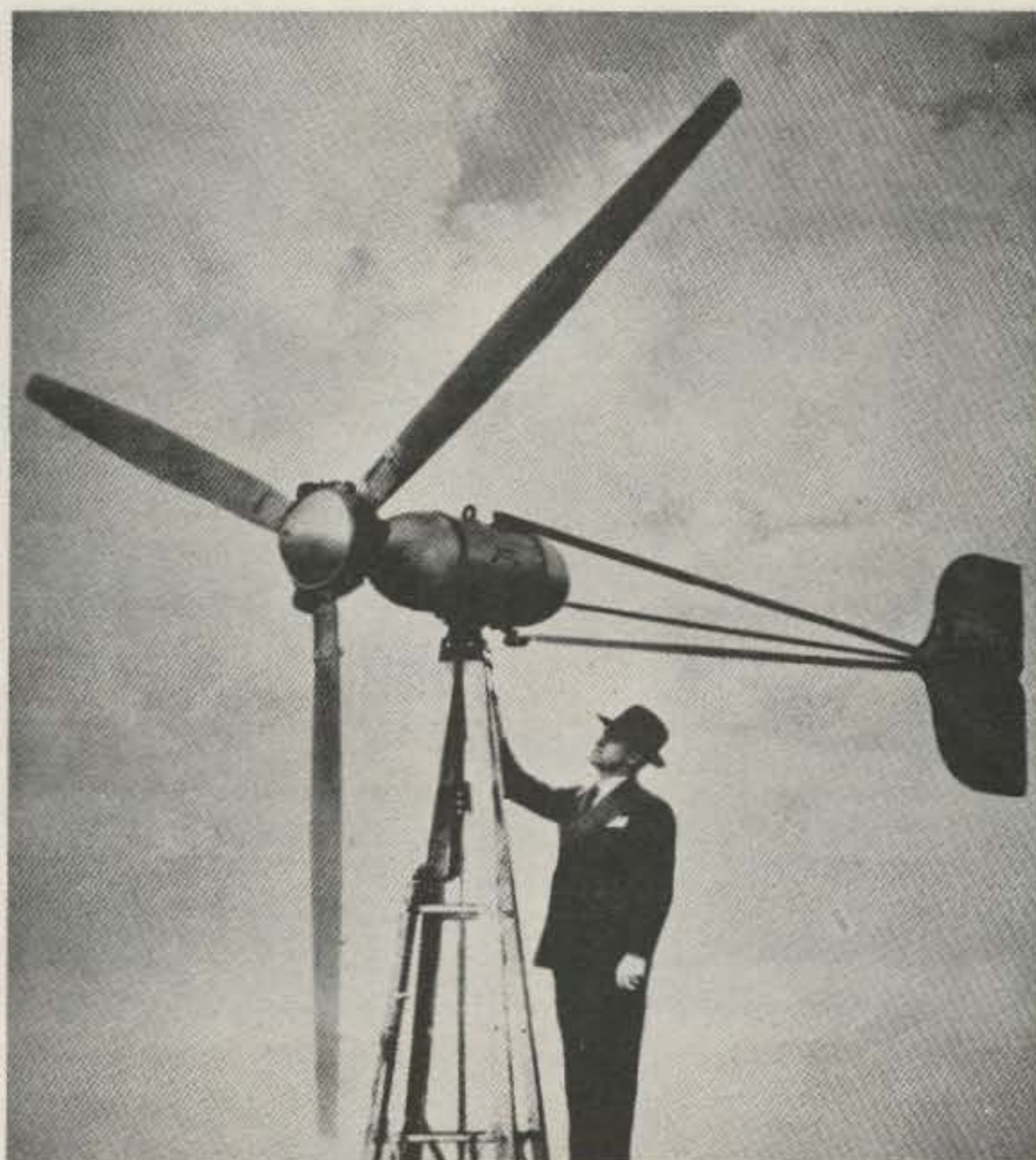
Marcellus Jacobs poses to give prospective customers an indication of the size of the Jacobs wind electric plant.
