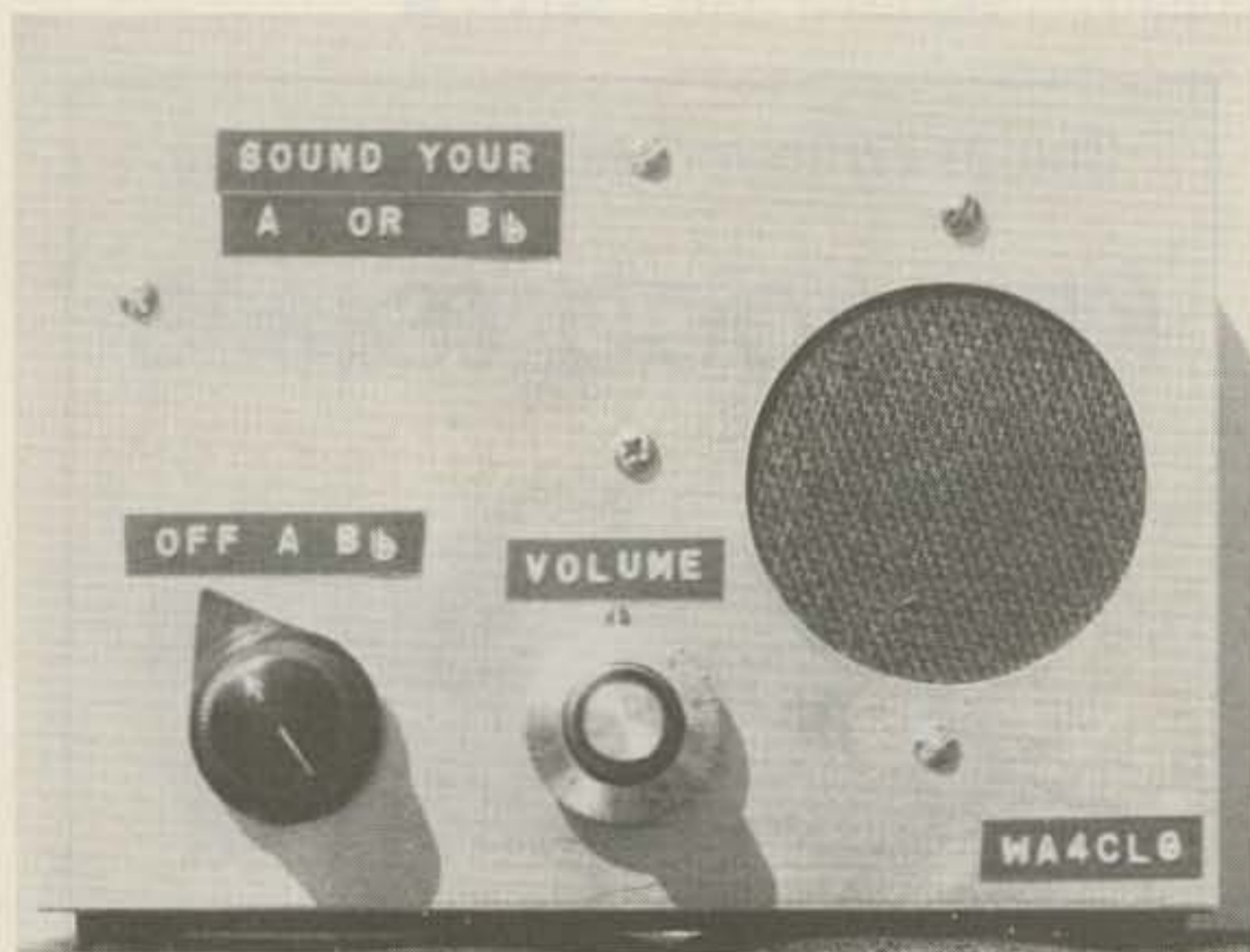
Photo 1. Front panel of completed standard pitch generator.
