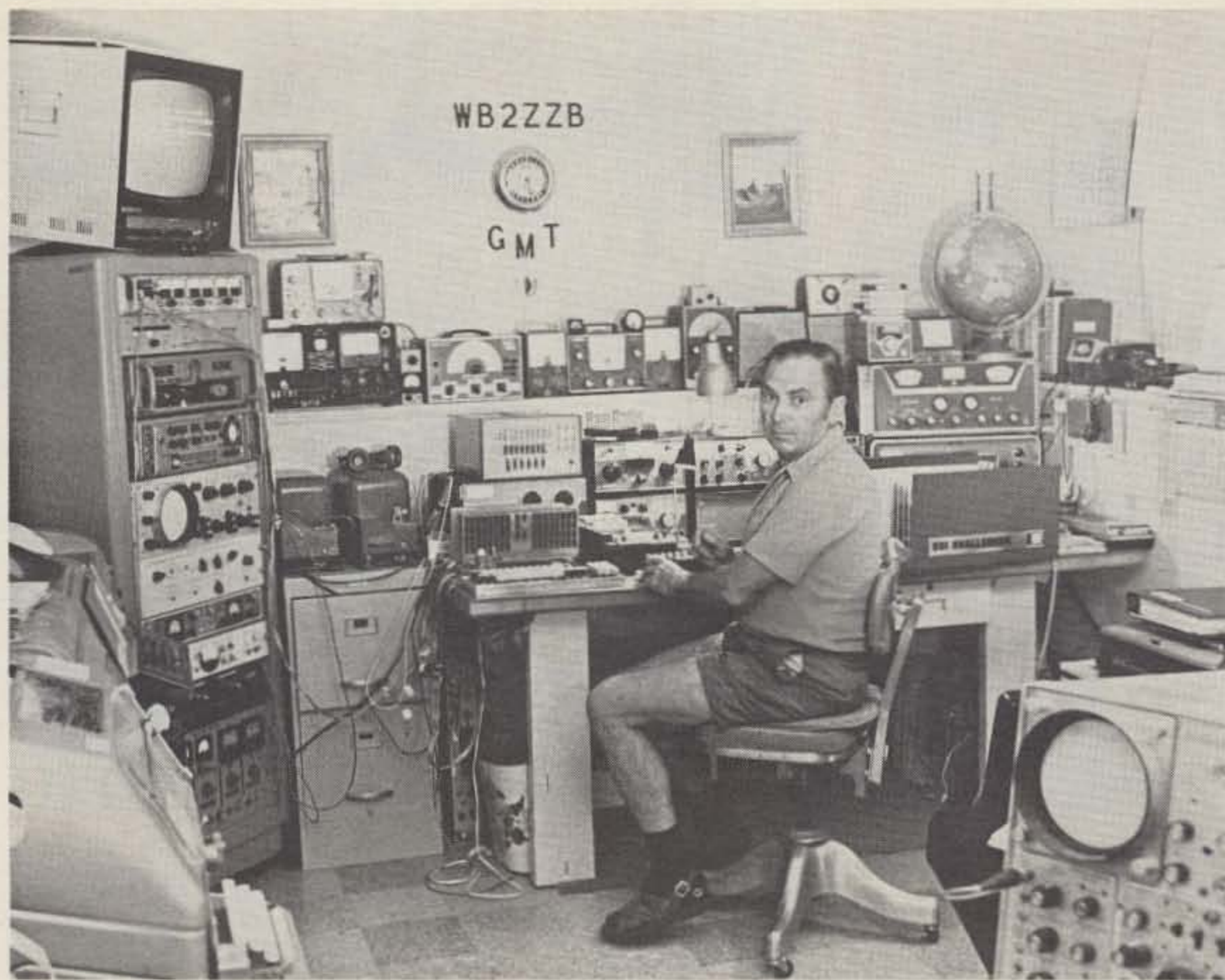
As Hans taps out instructions, they appear on the screen at the top of the rack. Simultaneously, the Teletype™ machine on the left makes a printout.
