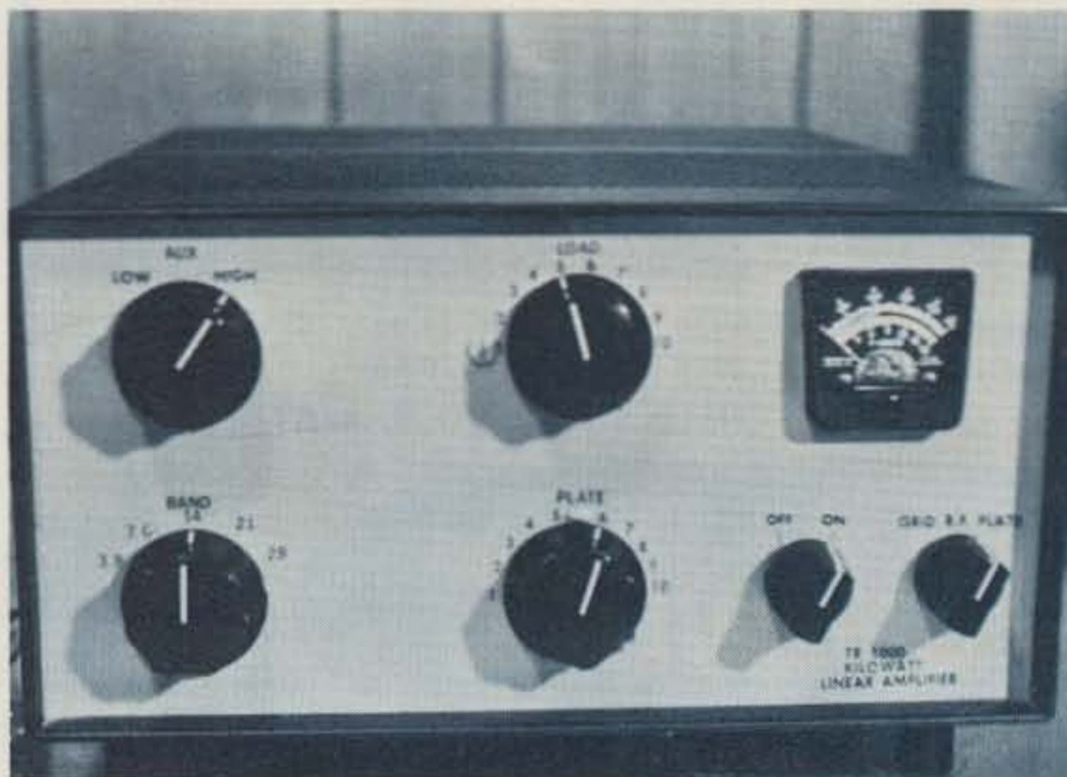
Front view of classic amplifier shows R.L. Drake cabinet and knobs. Illuminated Heathkit-type meter is modified to read amplifier plate current, grid current, and relative output.
