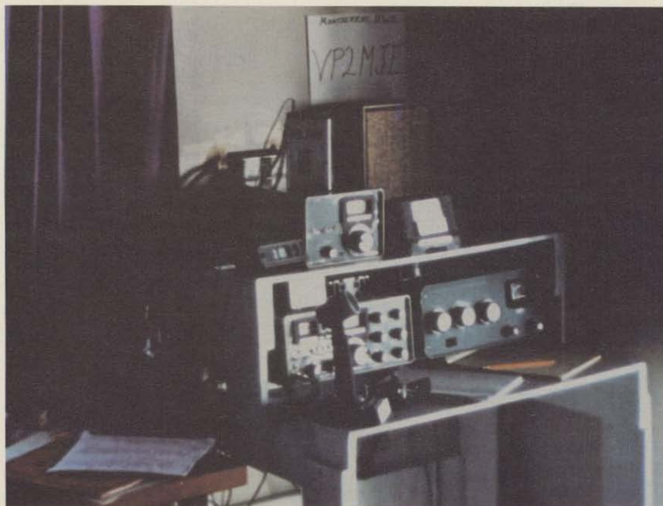
View of operating area. Equipment shown: Yaesu FT-101B, FV-101B, and Heath SB-200 linear.
