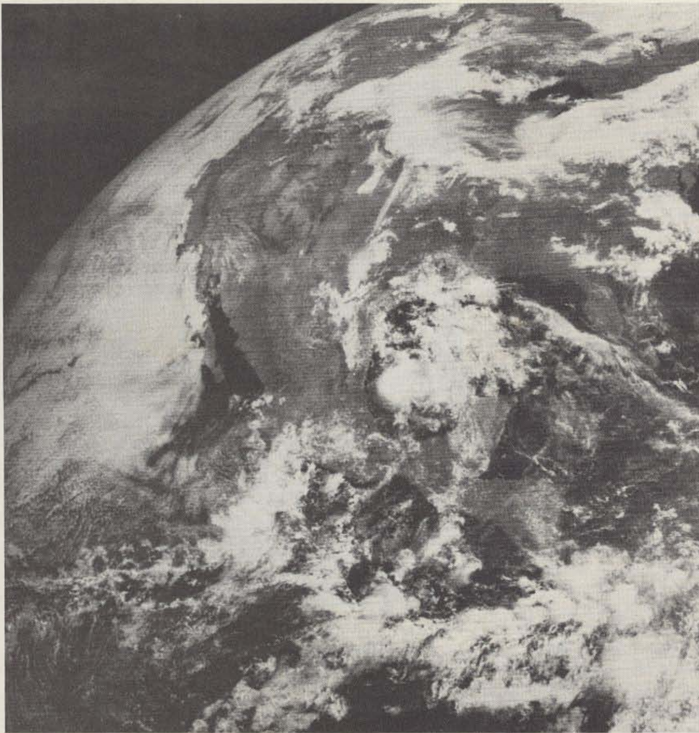
Photo D. This is an example of a properly phased GOES WEFAX picture. It was received and processed by the equipment in Photo C.
