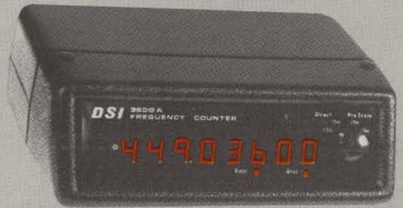
MODEL 3600A $199.95 INCLUDES OVEN TIMEBASE \pm .5 PPM
