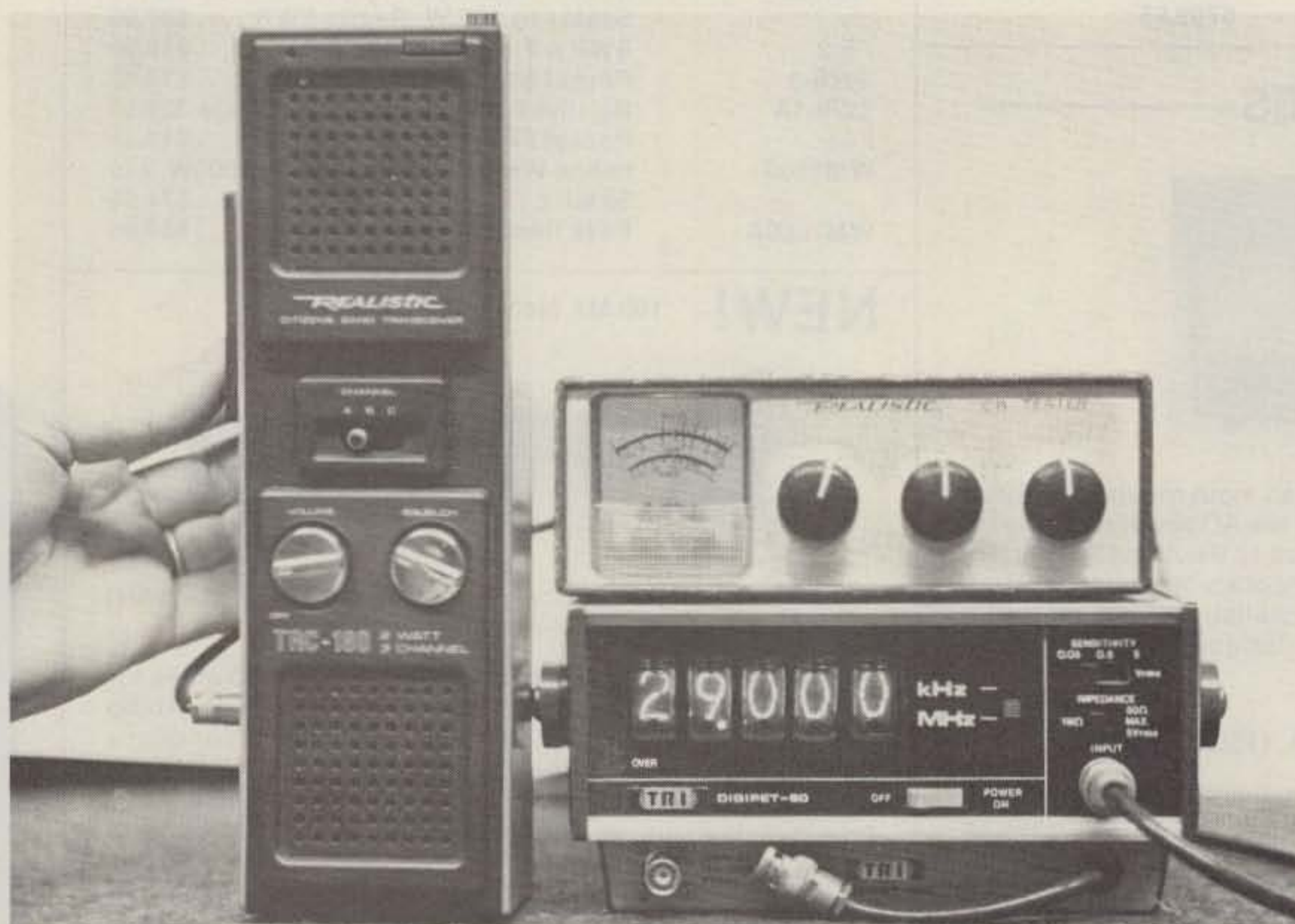
Walkie-talkie using external antenna connection to wattmeter and dummy load. Unit showed an output of over 1.5 Watts at 29.000 MHz.
