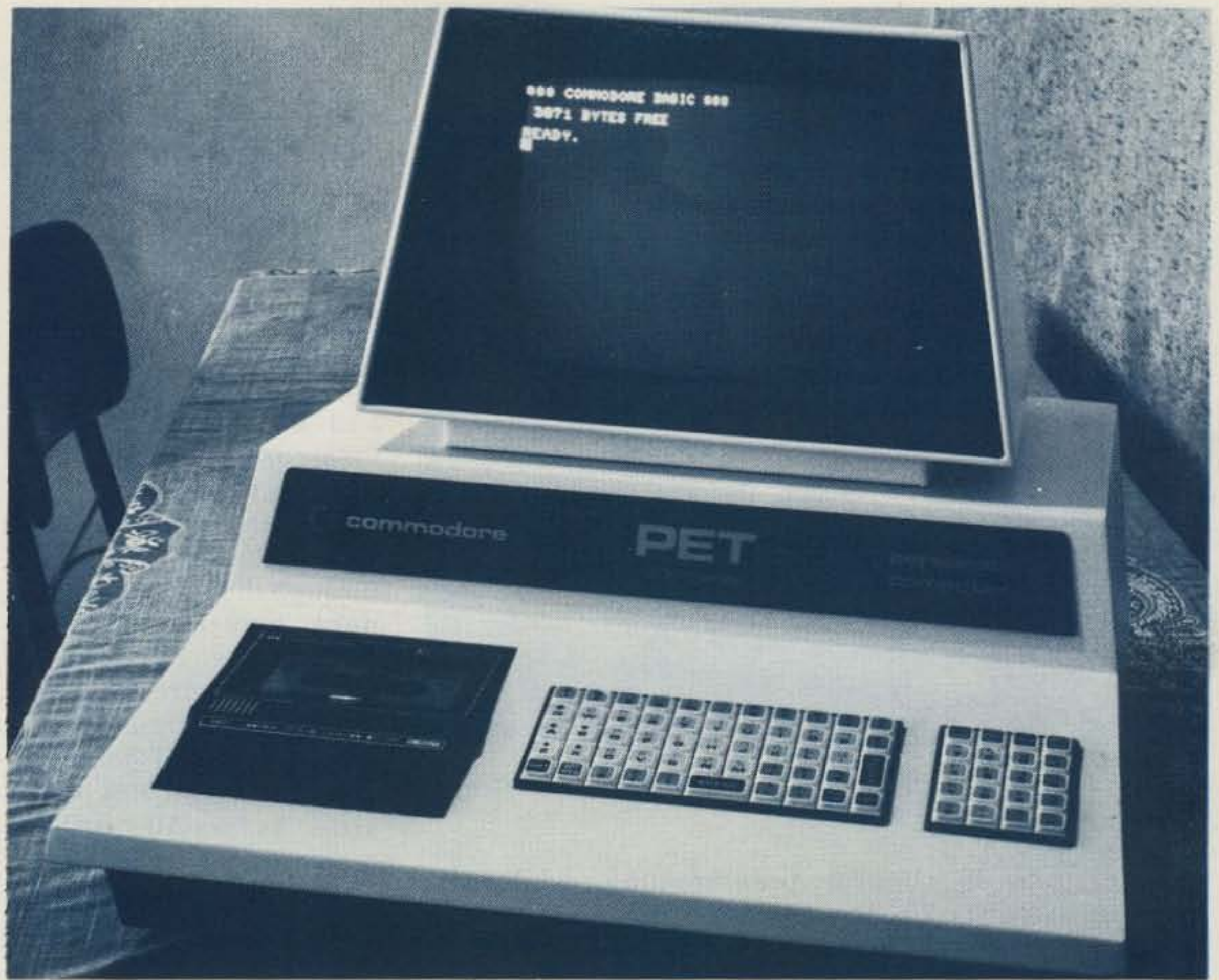
Photo 1. External appearance of the PET, showing keyboard, cassette, and display.
