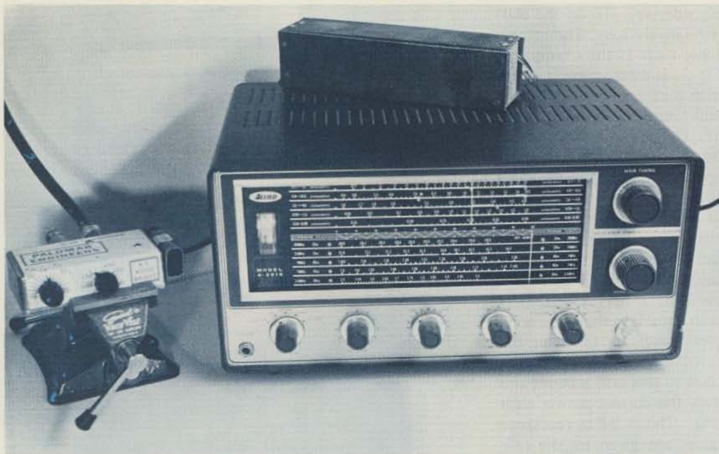
Measuring an impedance with the R-X bridge and a battery-operated receiver.
