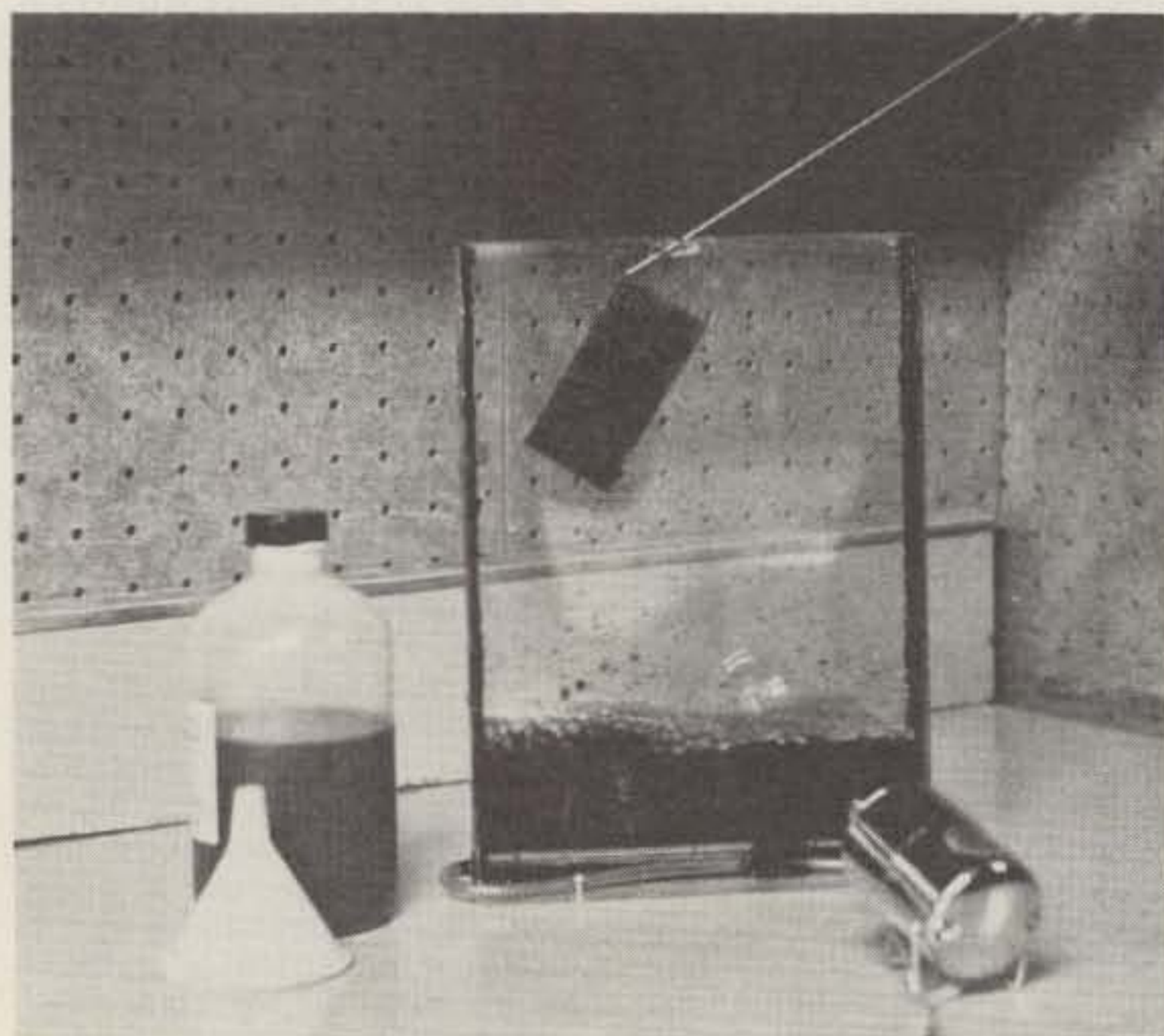
Completed etching tank in action showing removal of finished PC board.
