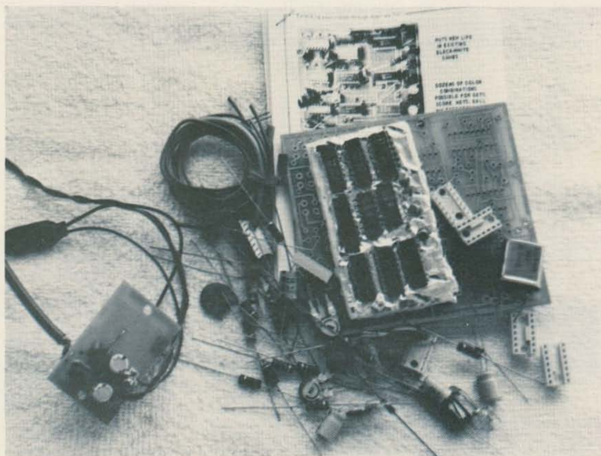
Home brew haven! Here's the ATV Research Chroma-plex 7700 color converter for home video games ready for construction. Highly detailed instructions make this affair just a few hours long. The unit on the left is the ATV Research Pixe-Verter which permits video to modulate a simple VHF oscillator.
