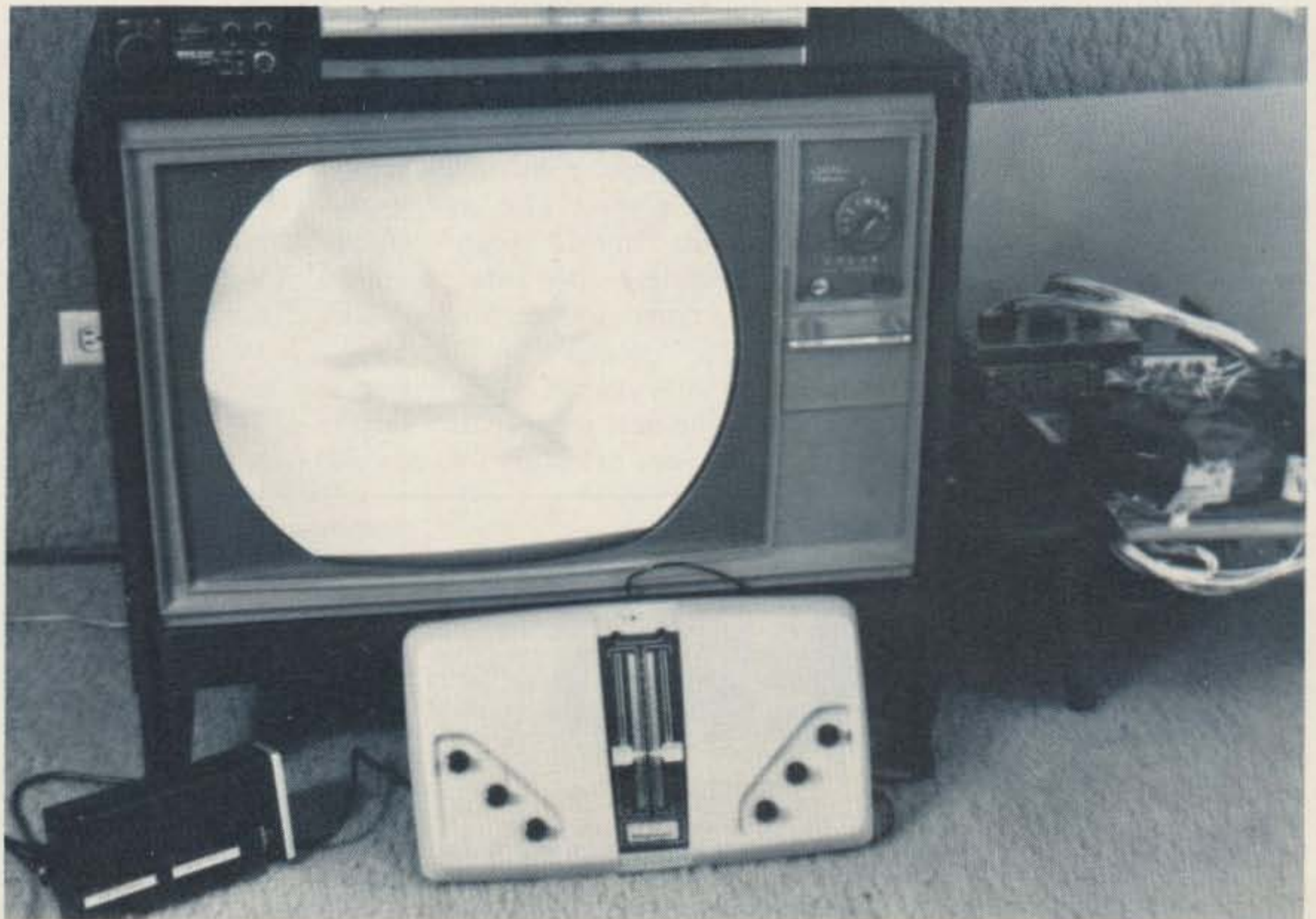
Video entertainment gear set up and ready for action. The cartridge tape deck is propped on the footstool and support circuitry is behind it. The CCTV camera and TV game can drive either television or tape recorder. The recorder can also tape programs during the operator's absence.
