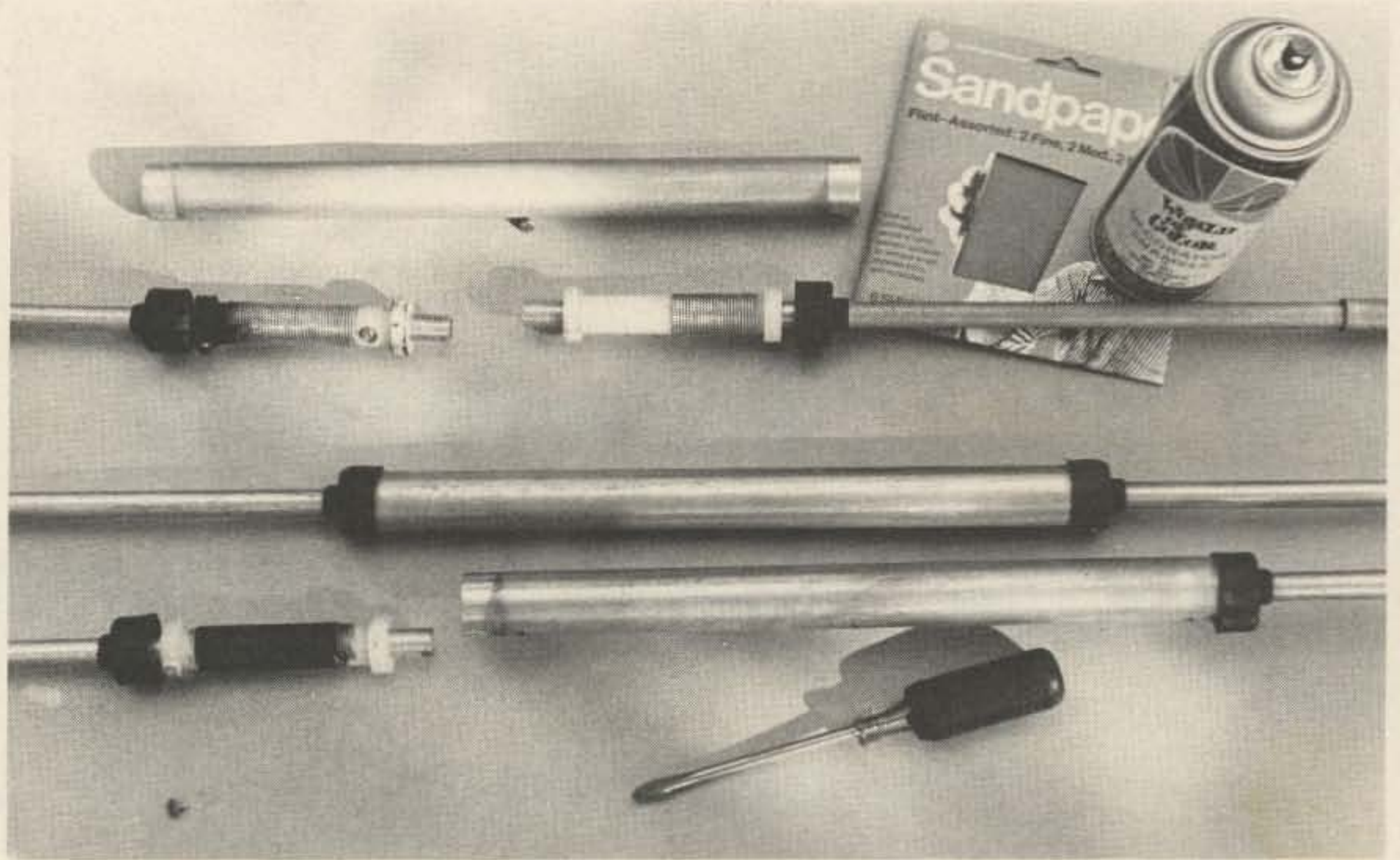
Photo B. This shows what's in a trap and how it's disassembled. The coil in the upper left was charred by a carbonized path, as described in the text. The driven-element coils are coated with Corona Dope to improve rf insulation.
