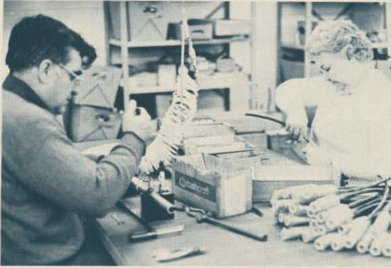
Here's Ray Doville and Claire Jacob assembling baluns for the Cushcraft three-band beams.
