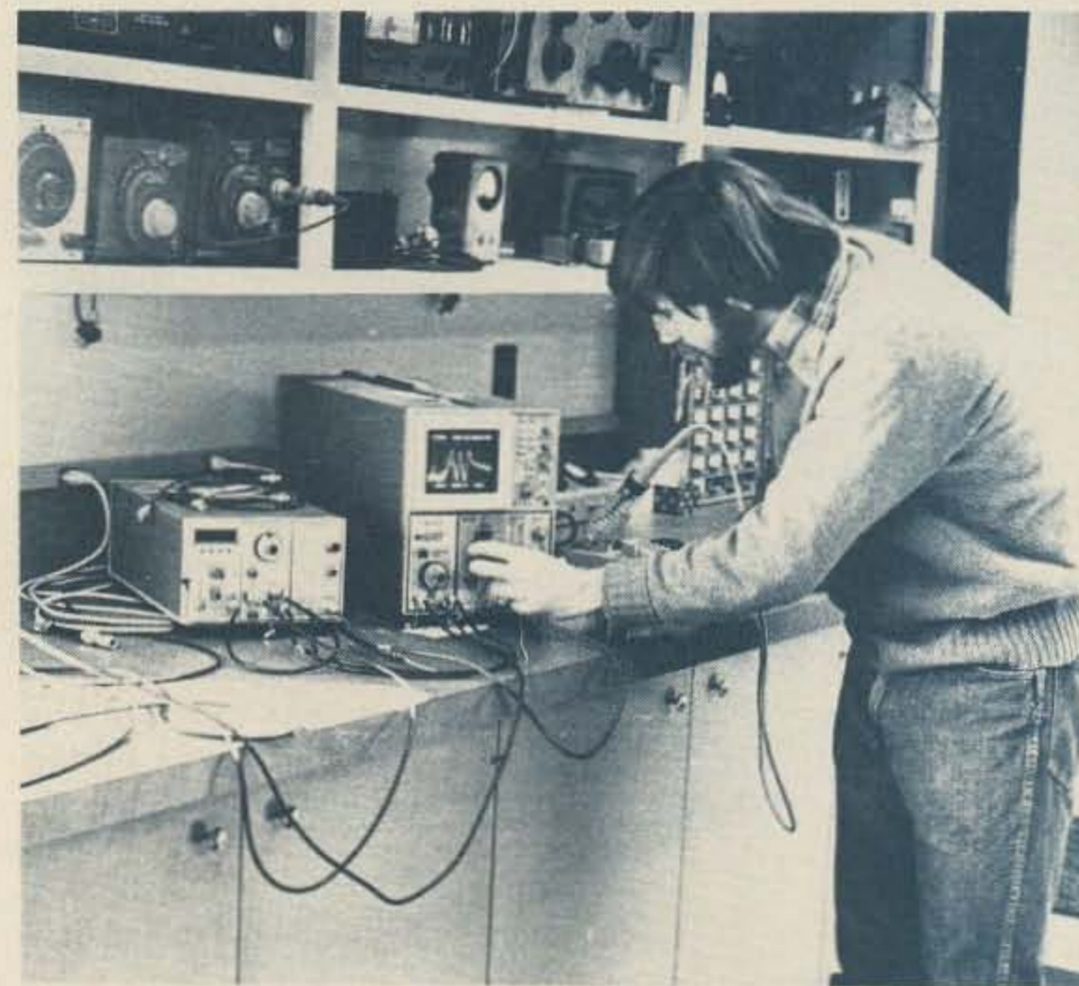
In the lab, where new antennas are developed and current designs are checked for performance, we see Dale Clement WA1FSZ checking the tuning of a three-band beam. The test setup is a ham's dream, with a motor-driven tower for changing antennas easily (well, relatively easily), a frequency sweep spectrum analyzer, and an antenna pickup range fed with hardline coax.
