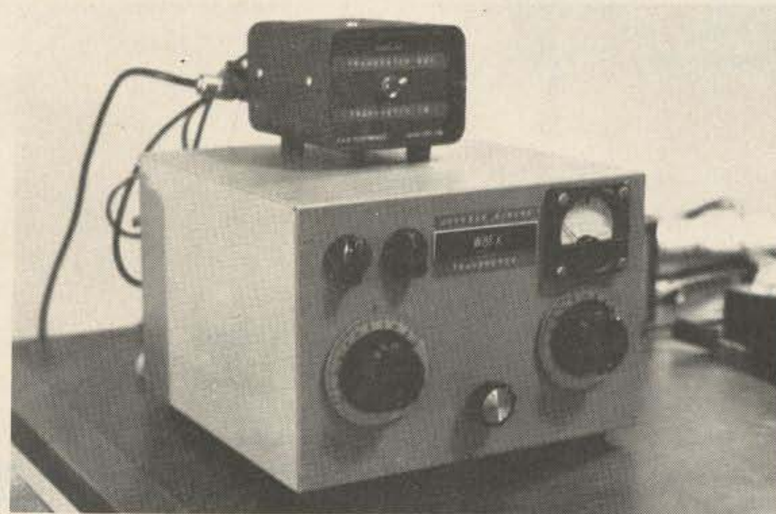
Fig. 2. P & H Model AR-1 linear switch. *2- or 3-position coax switch may be installed to allow antenna or antenna/dummy load selection. **Allows selection of straight-through operation or routing antenna/dummy load through Matchbox coupler. (SW1 is an internal part of the P & H switch and is front-panel mounted.)
