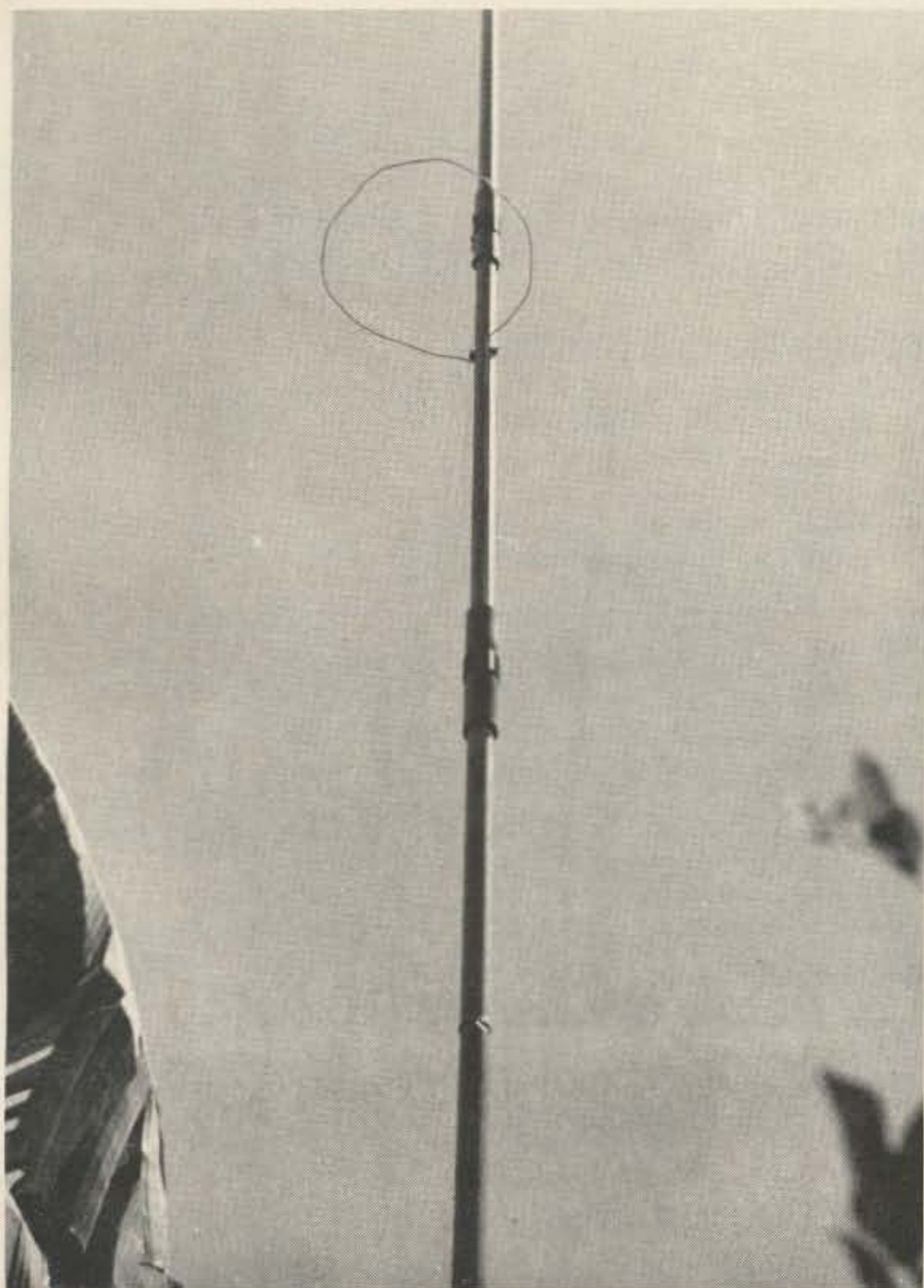
Vertical assembled for use on 20 meters. Operation before and after growth of the plants showed no noticeable difference in swr or effective radiation. Note that no traps are used on this band.
