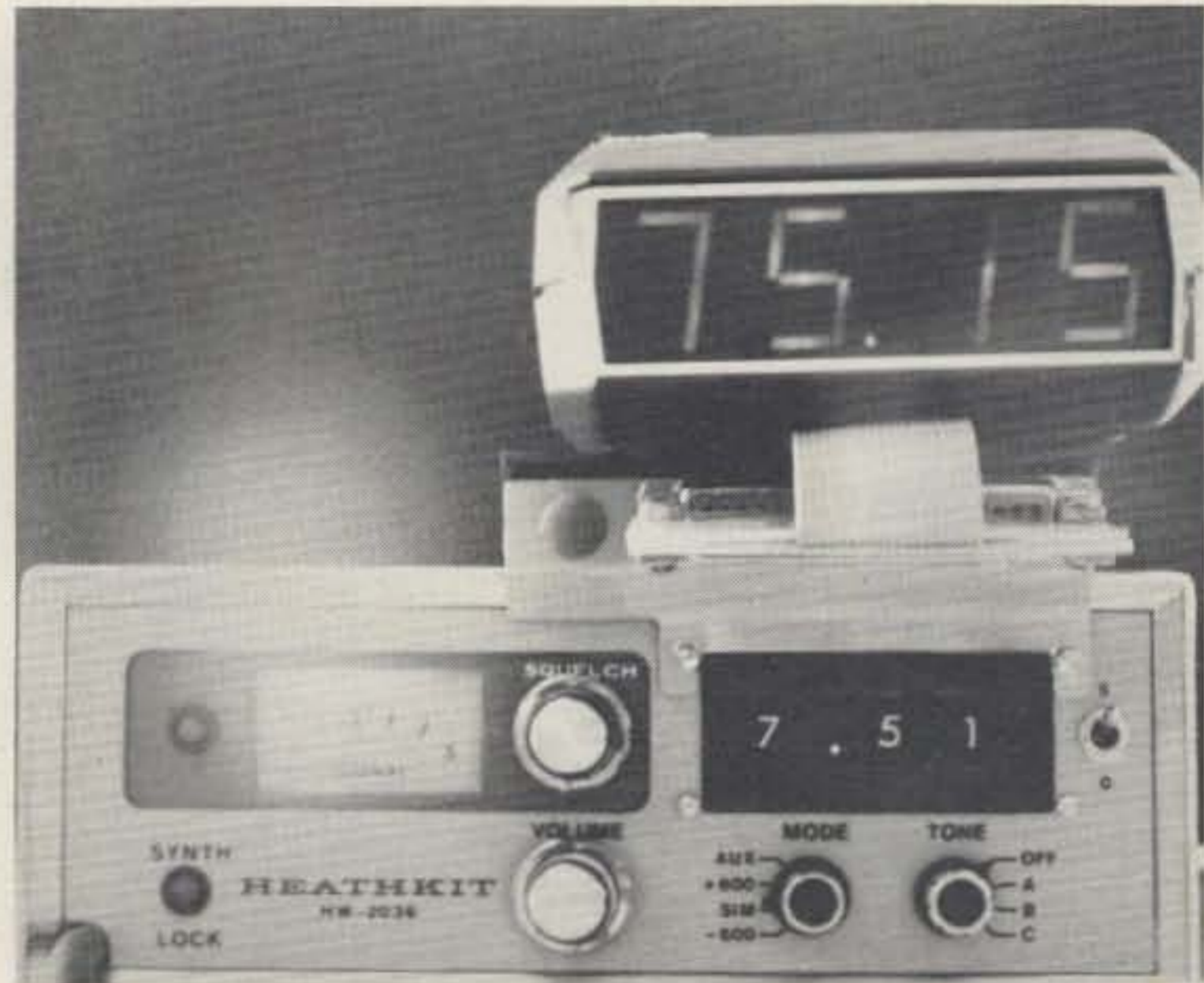
View of completed unit connected to transceiver. The dot in the lower center of the display between 5 and 1 indicates simplex mode.
