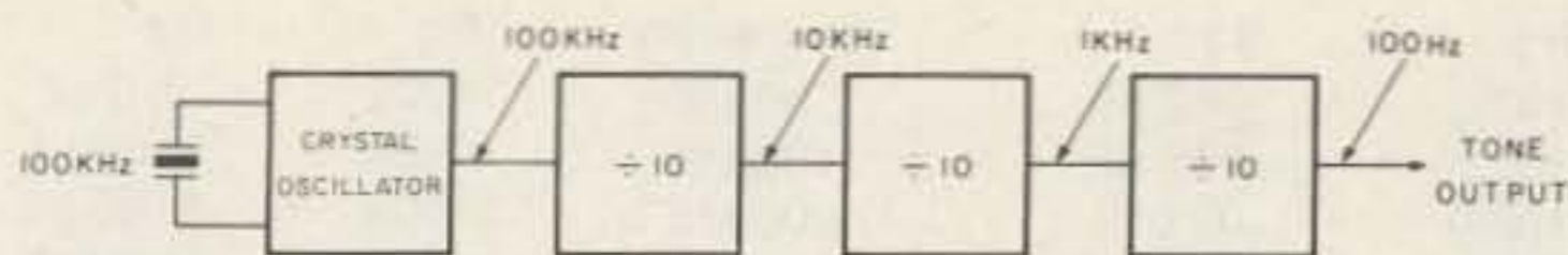
Fig. 1. Crystal-controlled audio tone generator.
