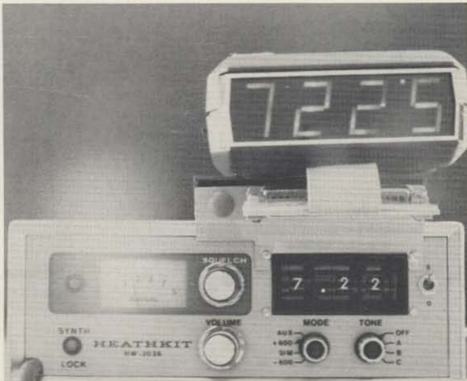
View of completed unit connected to transceiver. For this photo, the display was turned on and the PTT button operated to show mode indication LED. The dot at the upper left corner of the 5 indicates +600 kHz mode. The unit is resting on top of the transceiver for the photo. In the car, the unit attaches to the dashboard by means of Velcro strips glued to the dash and the top of the display unit.
