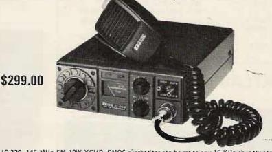
IC-22S. 145 MHz FM 10W XCVR. CMOS synthesizer can be set to any 15 KHz ch. between 146 & 148 MHz by diode matrix board. Spurious attenuation far better than FCC spec. 10W or 1W. IDC modulation control.
