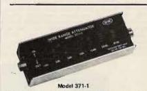
Protect your receiver or converter from overload, or proinde step attenuation of low-level RF signals (rom signal generators, preamolifiers, or converters Seven rocker switches provide attenuation from 1 dB to 61 dB in 1 dB steps. Switches are marked in dB, 1-2-3-5-10-20-20. Sum of actuated switches (IN position) gives attenuation With all switches in OUT position, there is NO insertion loss Attenuator installs in coaxial line using UHF connectors
