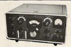
KWM-2A TRANSCEIVER \$3533.00 Unmatched for mobile and fixed station applications. 175W on SSB, 160W on CW. Switch select up to 14 optional Xtals. Can be used for RTTY. Filter type SSB generation. Automatic load control. Inverse RF feedback. Reimeability-tuned variable oscillator.
