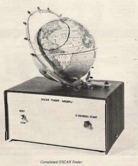
quentially turning on and off to simulate the position of OSCAR. The project used several gearing arrangements, entirely too many LEDs, and a 115-position rotary switch to accomplish its task. I felt this to be too costly and mechanically complicated, and I was prompted to simplify this otherwise excellent article.
