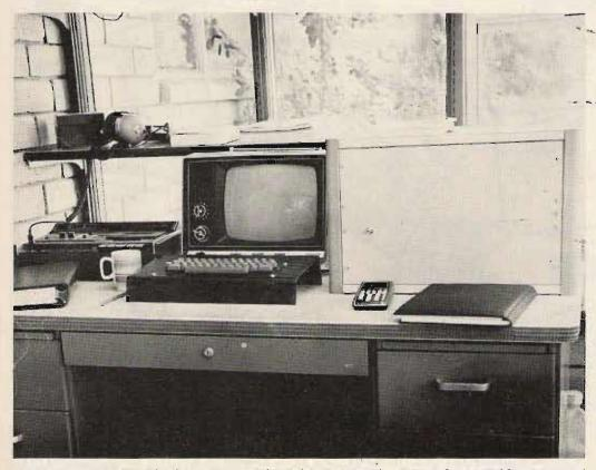
The microcomputer. The large box on the right contains the Digital Group Z-80 system and power supply.
