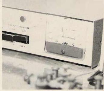
Many modern terminal units use a meter for tuning. A steady value indicates a properly tuned RTTY signal. Once the signal is tuned, the printer can be activated. The TU pictured is the HAL ST-5000.
