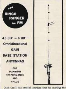
world's most popular 2 meter antenna twice as good. The new Ringo Ranger is developed from the basic AR-2 with three half waves in phase and a one eighth wave matching stub. Ringo Ranger gives an extremely low angle of radiation for better signal coverage. It is tunable over . broad frequency range and perfectly matched to 52 ohm coax.
