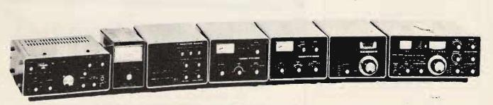
Left to right - FT-620B, 6 Meter Transceiver • YP-150, Dummy Load Wattmeter • YO-100, Monitor Scope • FTV-250, 2 Meter Transverter • FTV-650, 6 Meter Transverter • FV-101B, External VFO • FT-101E 160-10 M Transceiver
